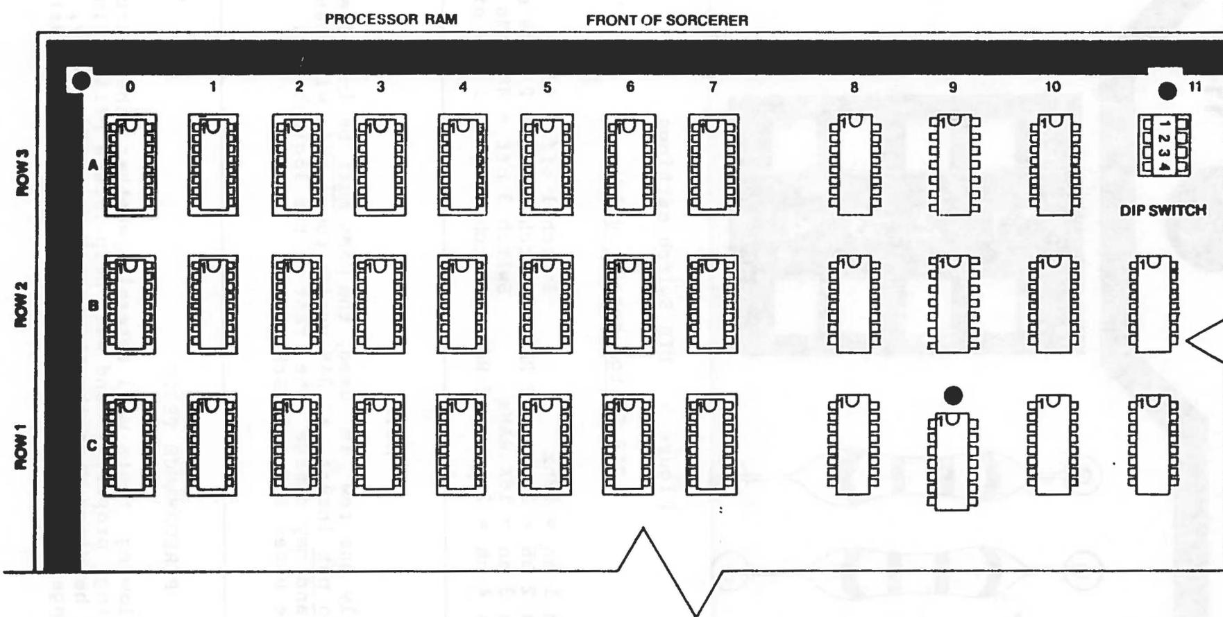
Figure 4 RAM Sockets and RAM DIP SWITCH, locations
