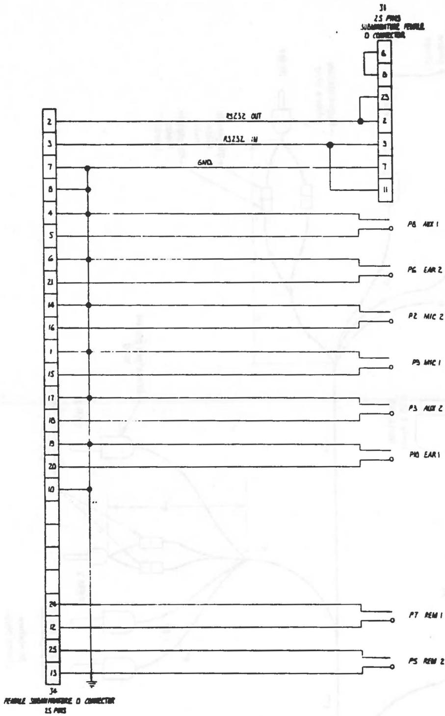
Figure 8 Serial Data Cable, Schematic
