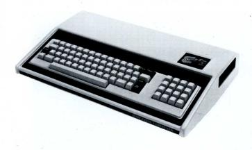
The EXIDY Sorcerer™ Computer uses a Z80 microprocessor; EXIDY's optional plug-in ROM PAC™ software makes the system powerful and flexible.
