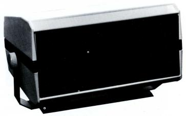
The EXIDY Video/Disk is a compact single unit styled to match the Sorcerer. It includes a twelve-inch video monitor with P31 phosphor, and a dual disk drive with built-in controller card. The Video/Disk plugs directly into the Sorcerer computer's 50-pin expansion connector; an S-100 expansion unit is not required to operate the disks. The Video/Disk comes with a disk operating system, full documentation, a cable for connection to EXIDY's Sorcerer computer, and a swivel base.
