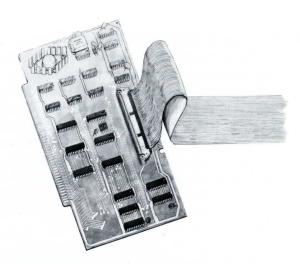
The EXIDY I/O Expansion Kit contains an S-100 interface card and a cable which attaches the card to the Sorcerer's 50-pin expansion connector. The interface card has the same bus controllers and buffers as the EXIDY S-100 Expansion Unit; it fits into any other S-100 mother board and allows the Sorcerer to control the bus. The interface card has a 2 MHz clock and receives power from the S-100 mother board.
