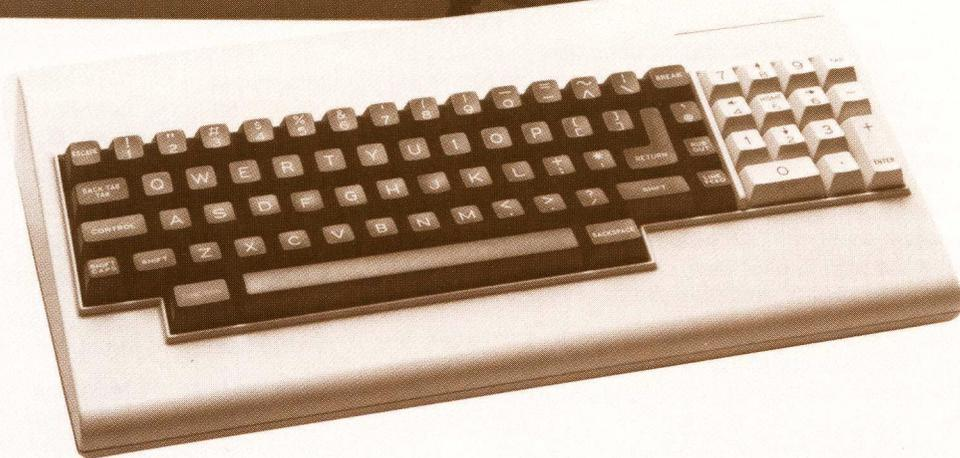
The TS-1SP Smart Paging Terminal offers all of the editing features of FALCO's popular TS-1, plus it has 16K memory for data storage at the terminal. This memory offers flexible control of data display and transmission.
