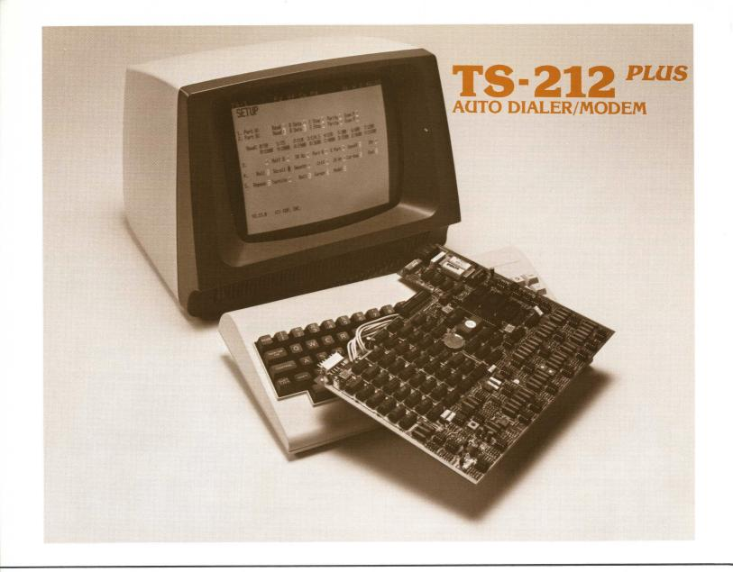
TS-212 PLUS provides cost effective, high performance 300 or 1200 bps, full duplex data communications over the switched network. It will originate and auto answer calls. It is compatible with all industry standard 212A, 103 and 113 series modems.
