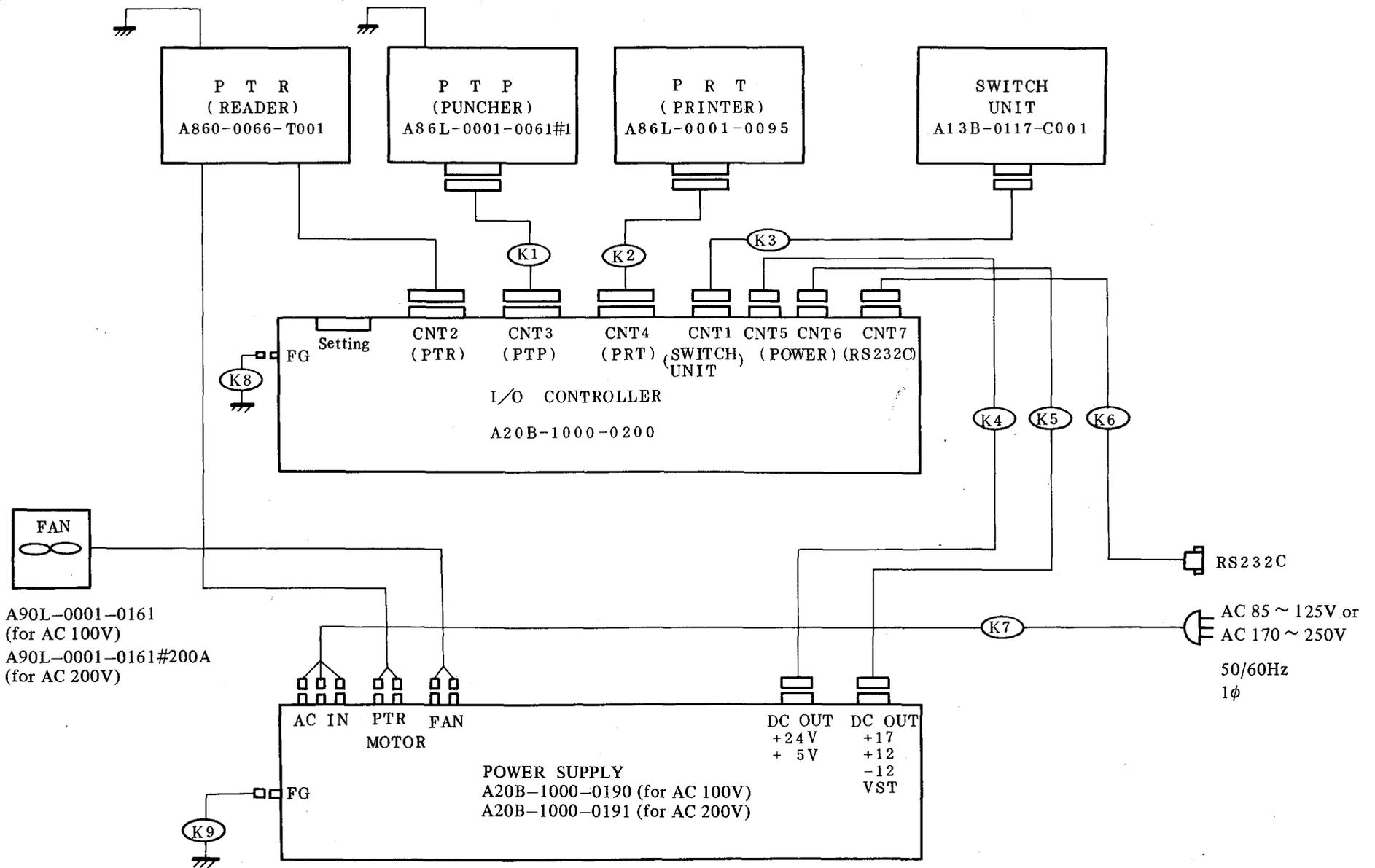
Fig. 5.1.2 FANUC PPR General Connection Diagram
