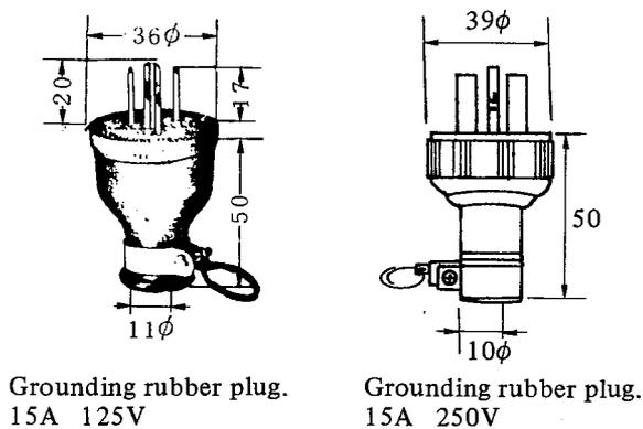
Fig. 6.2.1 (b) Tip connector of power cable
