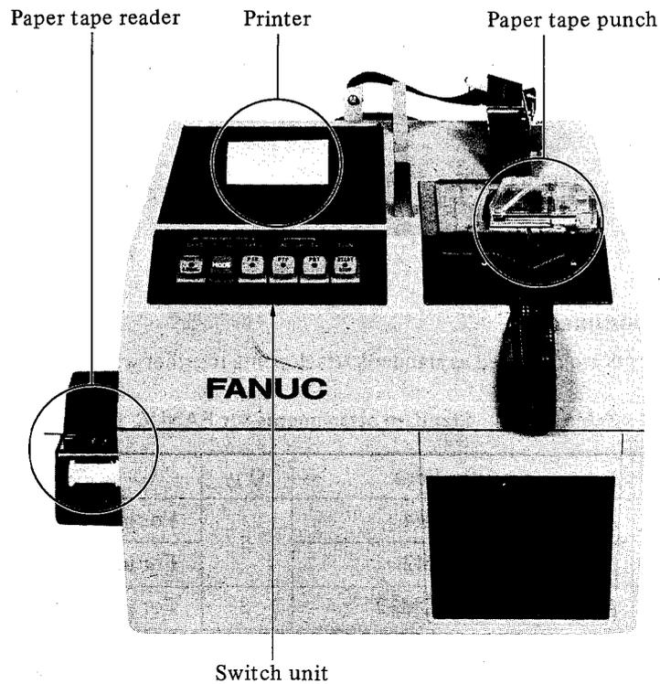
Fig. 2 Names of component parts of FANUC PPR
