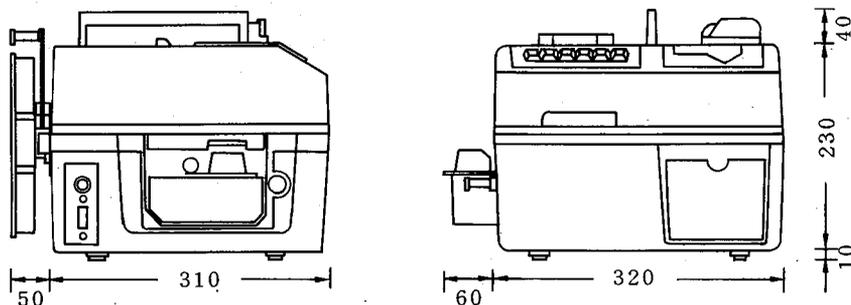
Fig. 1.2.2. External dimensions of FANUC PPR
