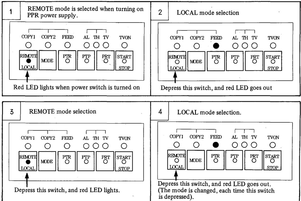
*(Note) When the printer, puncher or tape reader is operated, don't depress REMOTE/LOCAL key switch.*
