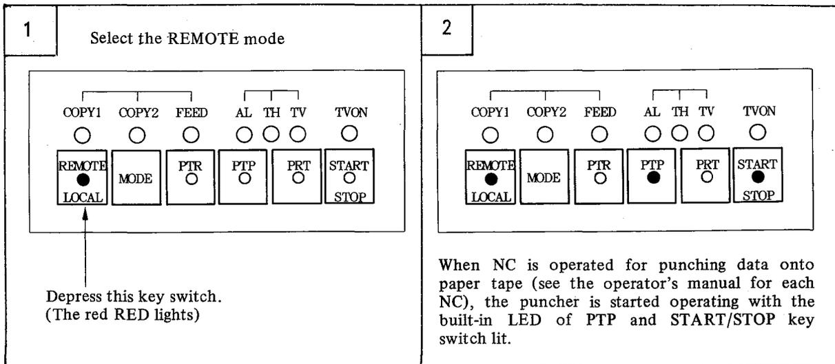
(Note) When the puncher is operating, don't depress PTP and START/STOP key switch.
