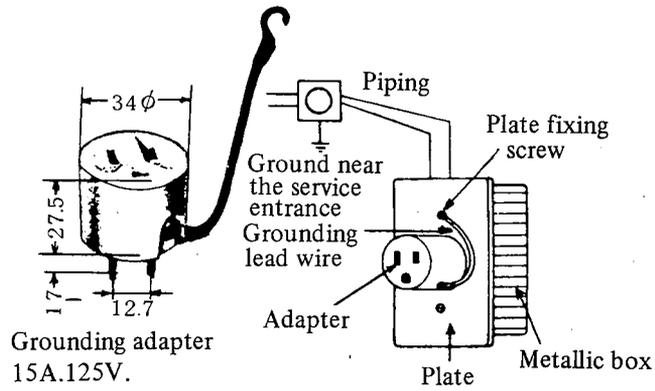
Fig. 6.2.2 Method of using the grounding adapter
