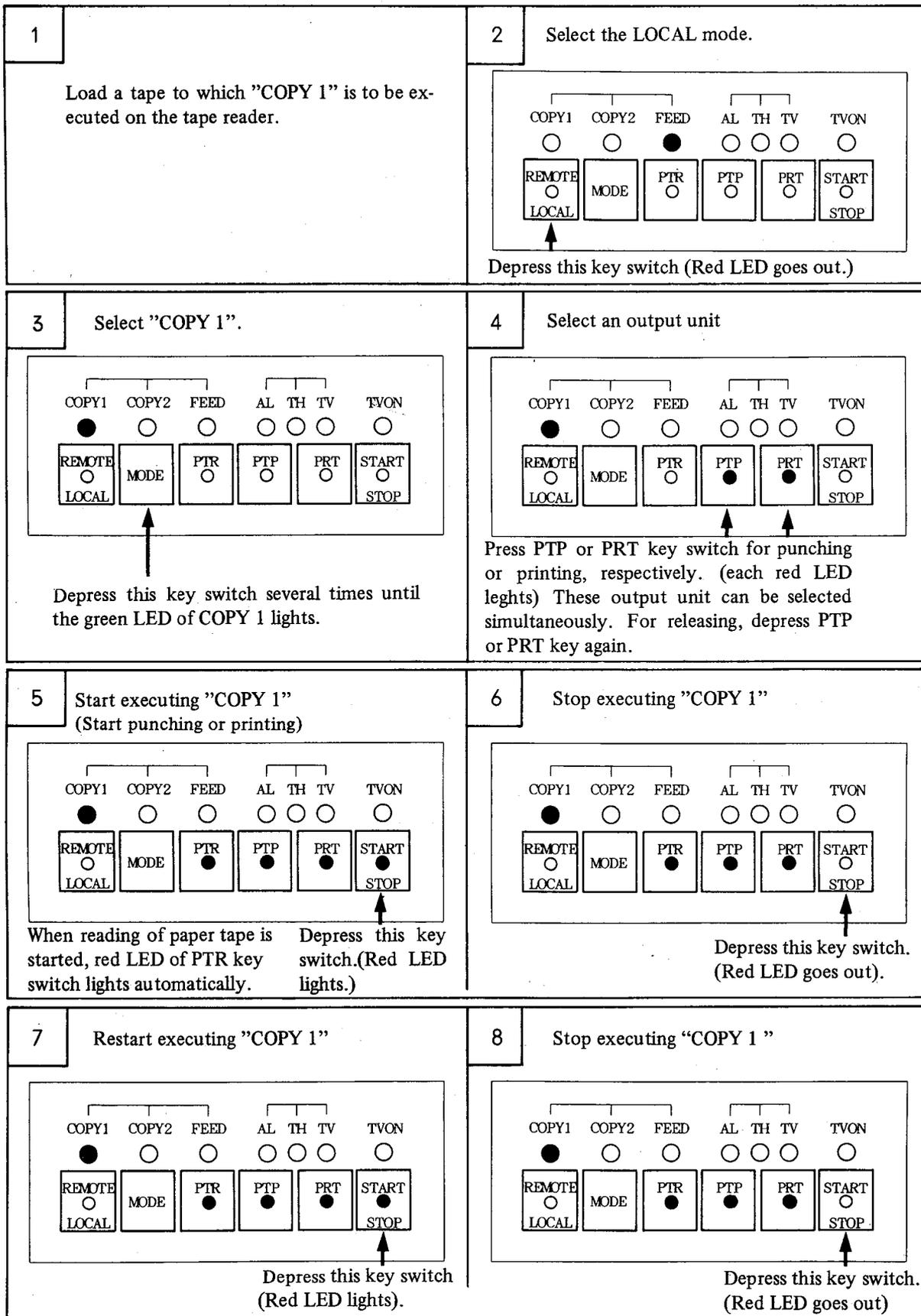
(Note) When the printer, puncher, or tape reader is operating, don't depress MODE key switch. Stop operating by depressing START/STOP key to change the mode, such as COPY 1 to COPY 2.
