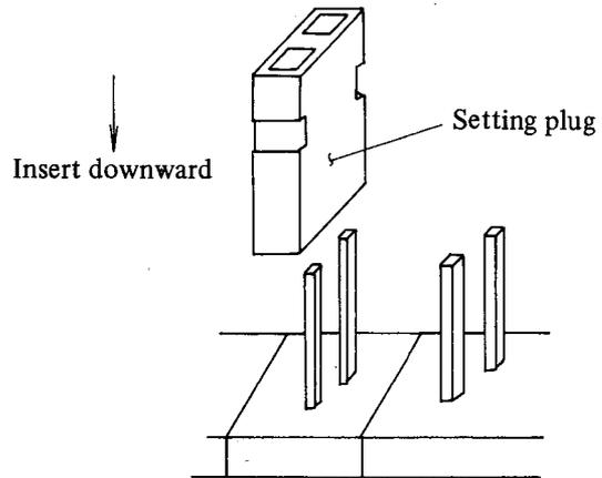
(Note) Turn off the power switch before setting. This setting becomes effective when the power switch is turned on again. If this setting is changed with the power switch turned on, it is not effective.
