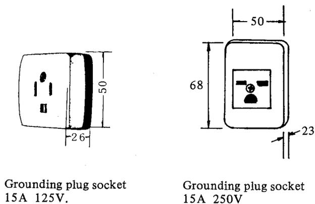
Fig. 6.2.1 (a) Example of power plug socket
