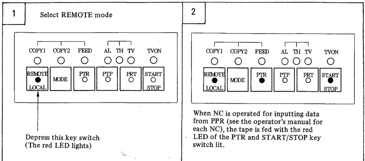
(Note) When the tape reader is operated, don't depress START/STOP key switch.
