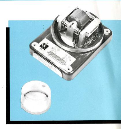
DRIVE: The drum is normally driven at 22,500 RPM by a 400 cycles per second, 117 volt, 3 phase supply. Power input at 400 cycles per second is 5 watts. The rotor may be operated at any supply frequency from 60 to 400 cycles per second to provide a wide range of operating speeds.
