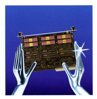
System 68000 VME SYS68K/SIO-1 Multi Protocol Serial I/O Controller
