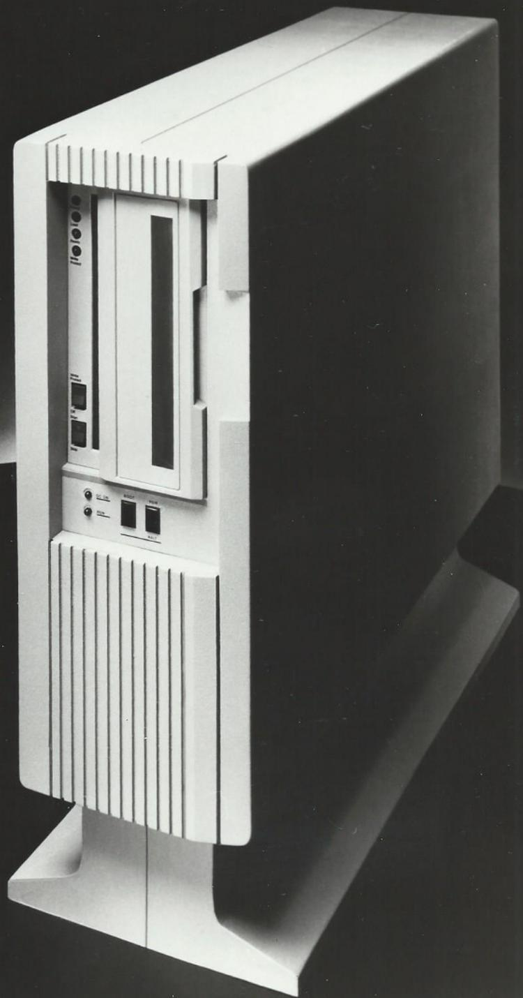
The Ford/Higgins variable architecture computer system offers a choice of PDP-11/23 PLUS processor with DEC operating systems or a 68000 CPU with UNIX<sup>tm</sup> operating system. The basic pedestal system includes 256KB of RAM memory and 40MB of fixed/removable disk storage.
