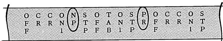
Now the requirements of the Master Program Tape have been completely determined. To punch the Master Program Tape the Punch Switch is put in ALL position and the codes are punched in the exact sequence indicated. Once these
