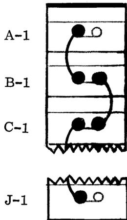
A connection is made from an outlet of A-1 to an outlet of B-1. The other outlet of B-1 is connected to an outlet of C-1. This plugging, in effect, connects A-1, B-1, and C-1 together. The remaining outlet of C-1 is then connected to an outlet of J-1.
