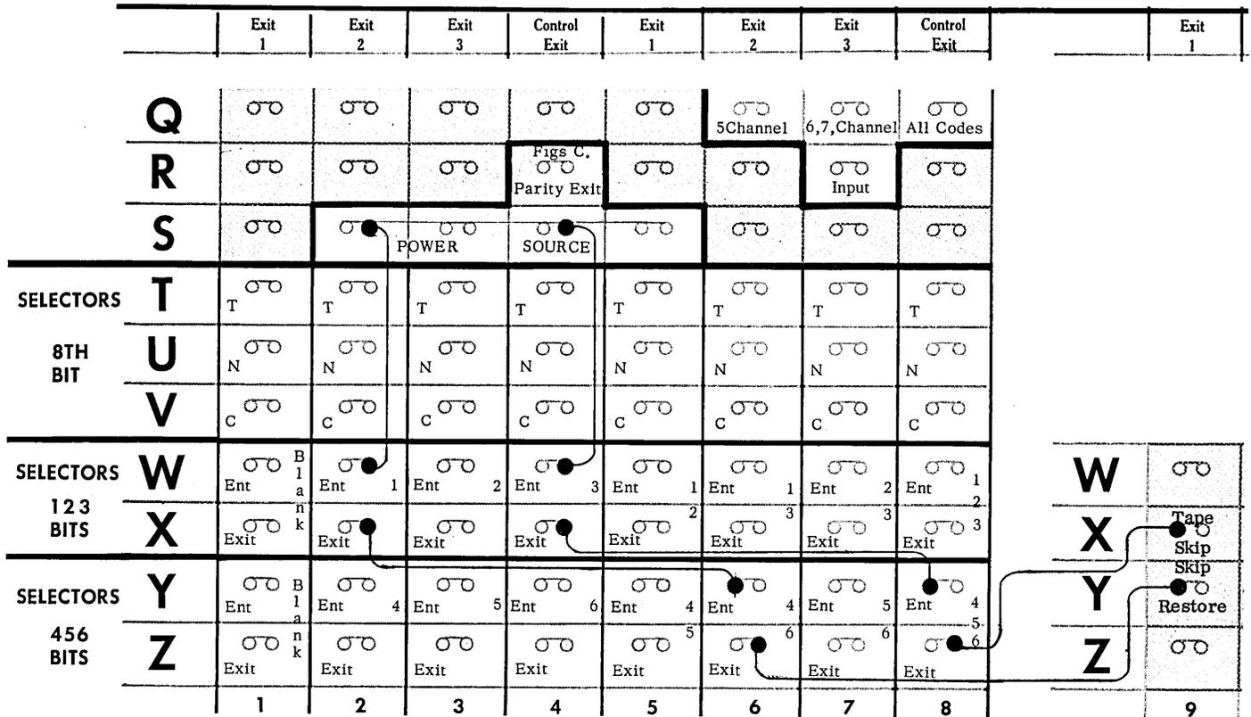
an output code. If it were required that the Skip Restore code punch an output code the CODE EXITS (G13, 14, 15) would be wired to the proper CODE ENTRIES in the standard fashion and the CONTROL EXIT (G16) would be wired to the proper functional entry (FIGS PRECEDENCE, LTRS PRECEDENCE, or NO-PRECEDENCE). Of course, if jumper connection P8-Q8 were made ( ALL CODES - NO PRECEDENCE), it would not be necessary to wire the control exit to a functional entry hub.
