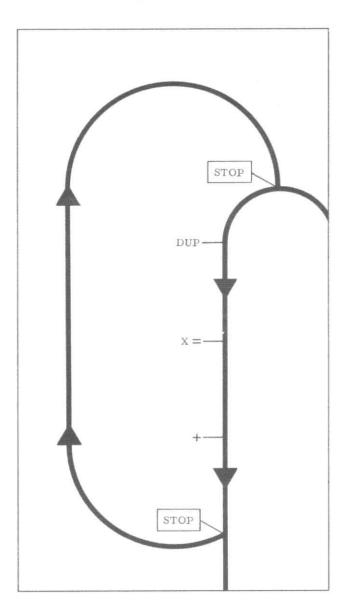
This ability to perform a manual loop allows us to re-use, indefinitely, the first portion of a program, avoiding the remaining instructions. The 1151 is the only desk-top programmable calculator that offers this program flexibility.
