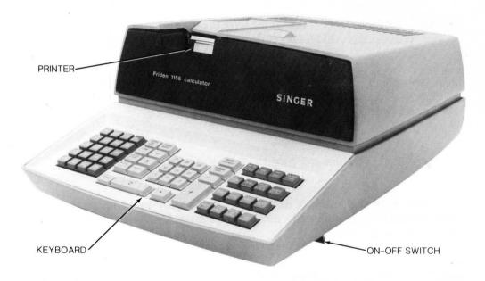
The ON-OFF switch is located on the right hand side of the machine, under the KEYBOARD. Turn the 1155 on. The PRINT wheel will spin, the decimal setting will be set at two, and •00 will print . . . the 1155 is ready to work.
