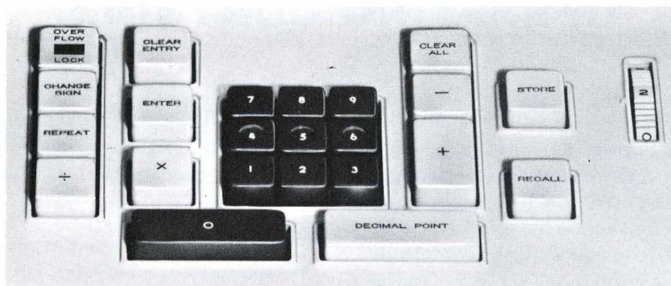
Register #2. The product will appear, decimally aligned, in Register #1. To multiply, the procedure is as follows: (1) Index the multiplicand (2) Touch ENTER key (3) Index the multiplier (4) Touch the Multiplication ( $\times$ ) key.
