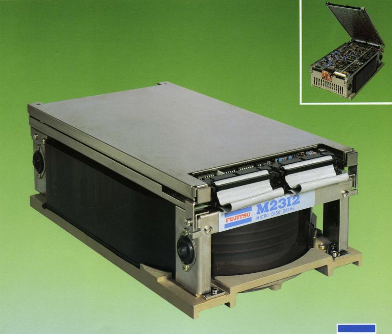
The M2311K and M2312K are 8-inch Winchester-type fixed disk drives designed to provide cost-effective storages for small computer systems and intelligent terminals in a broad spectrum of applications. Each drive consists mainly of a disk enclosure and three printed circuit boards. The disk enclosure integrates three or four disks, five or eight Winchester-type contact start/stop heads, a rotary actuator, a DC spindle motor, and IC read preamplifiers all in a small completely sealed package.
