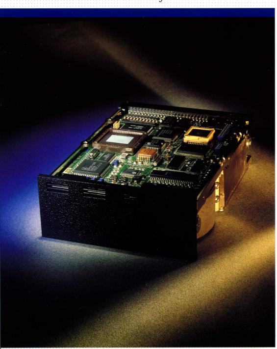
A high-performance family of 3.5-inch SCSI and AT drives, with formatted storage capacities from 330 to 520 megabytes.
