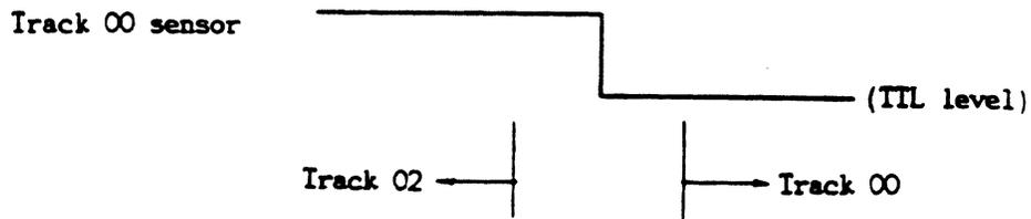
Figure 3-12 TP7 Track 00 Detect Waveforms
