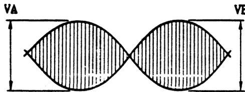
**Figure 4-11 Lobe Pattern for Track Alignment**
