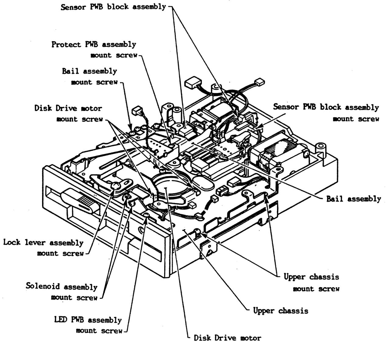
Figure 5-2 Top View of Disk Drive (View 2)
