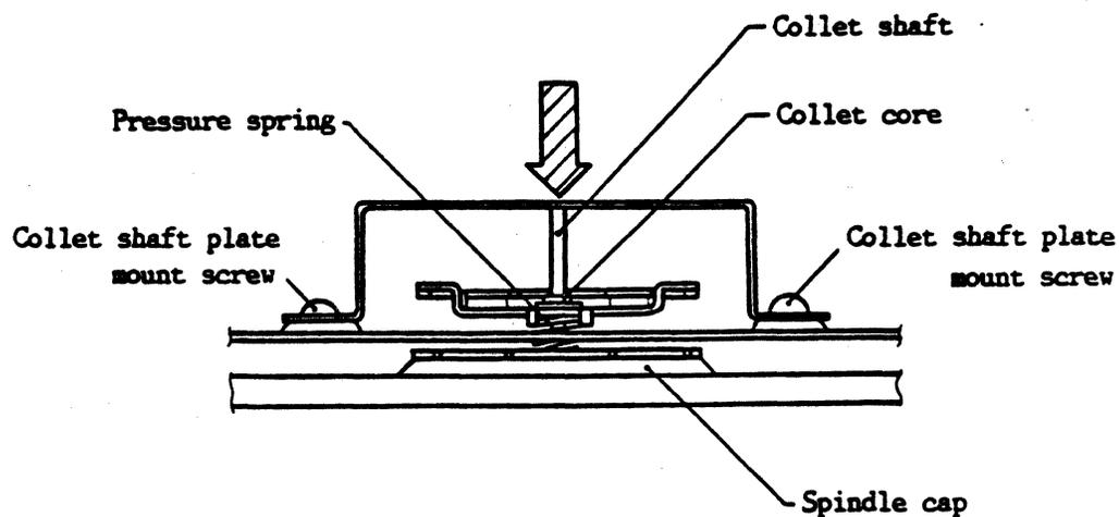
Figure 4-3 Collet Shaft Adjustment
