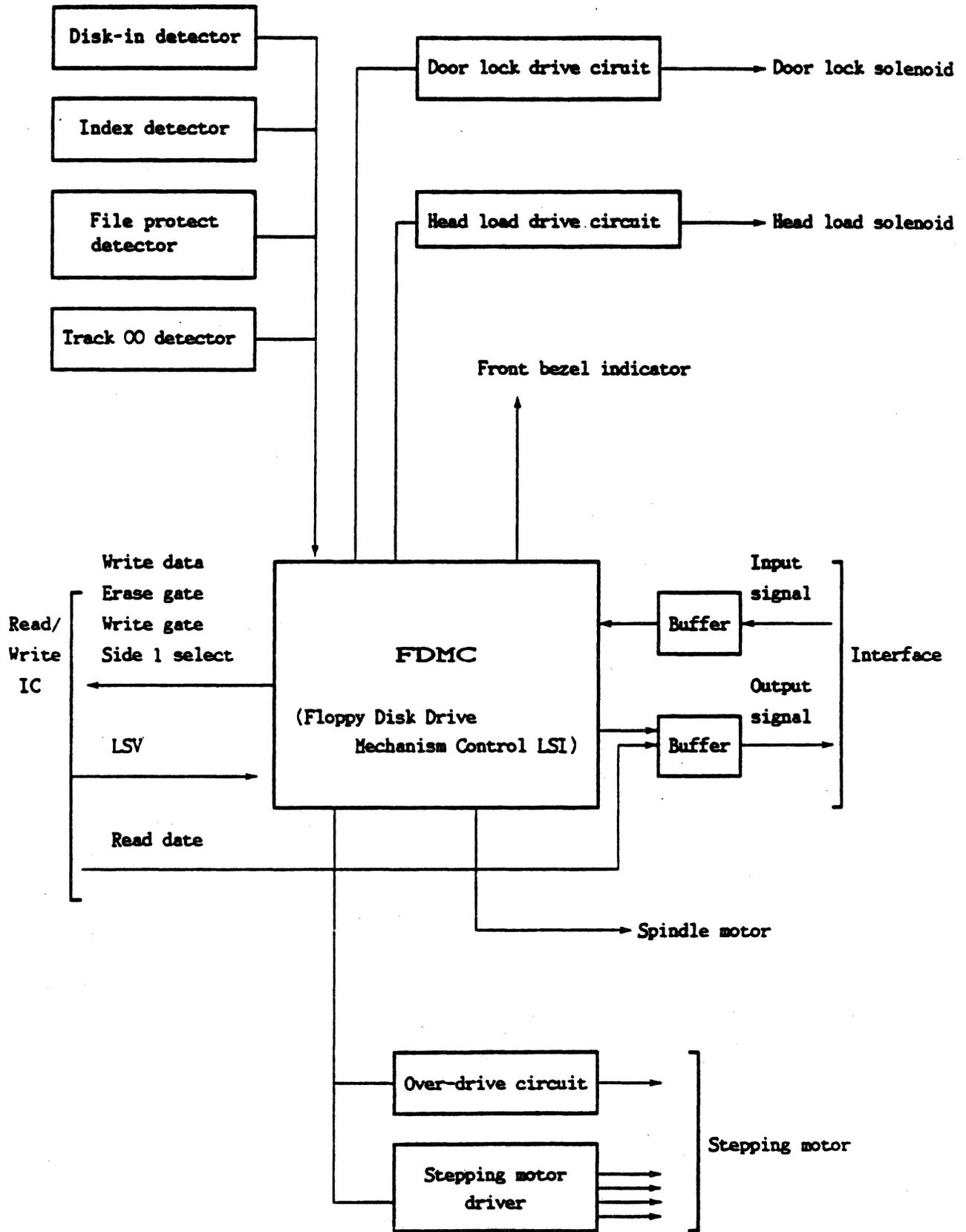
Figure 3-6 Control Circuits
