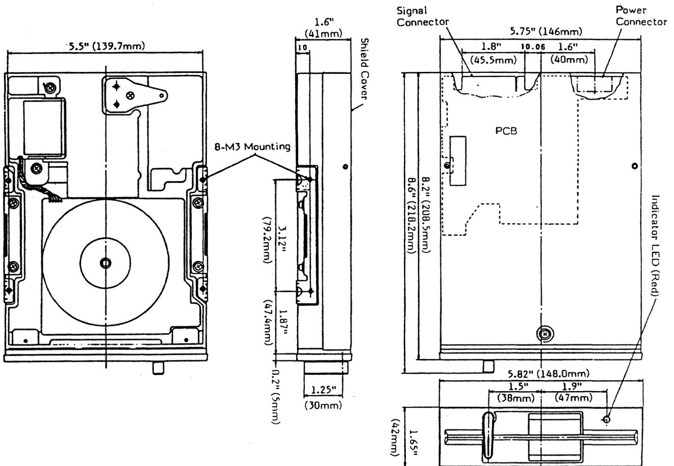
Figure 2-1 External Outline Drawing of Disk Drive
