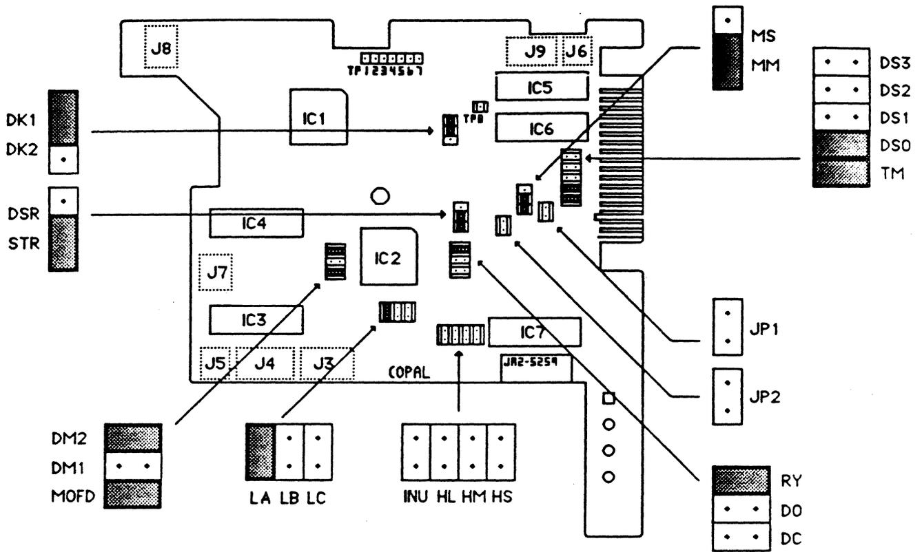
Figure 5-6 M2552K Revision 1 Circuit Card Layout
