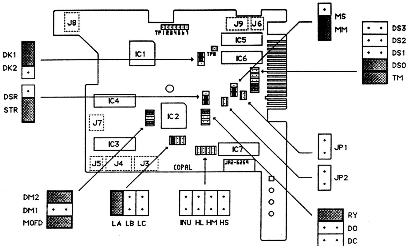
Figure 4-1C M2552K Revision 1 Circuit Card - Jumper Locations
