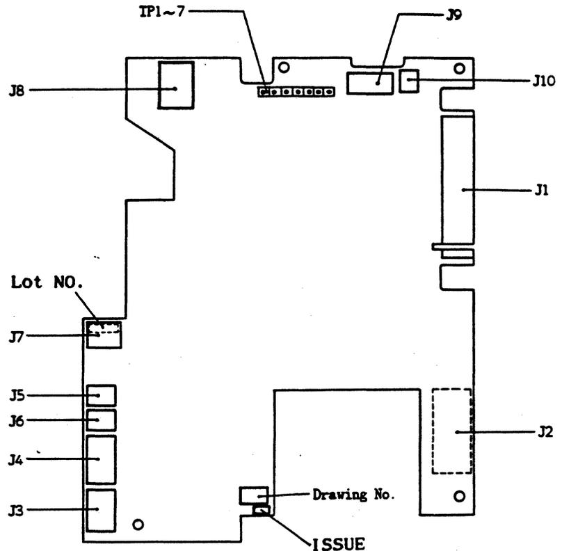
Figure 3-8 Location of Connectors and Test Points
