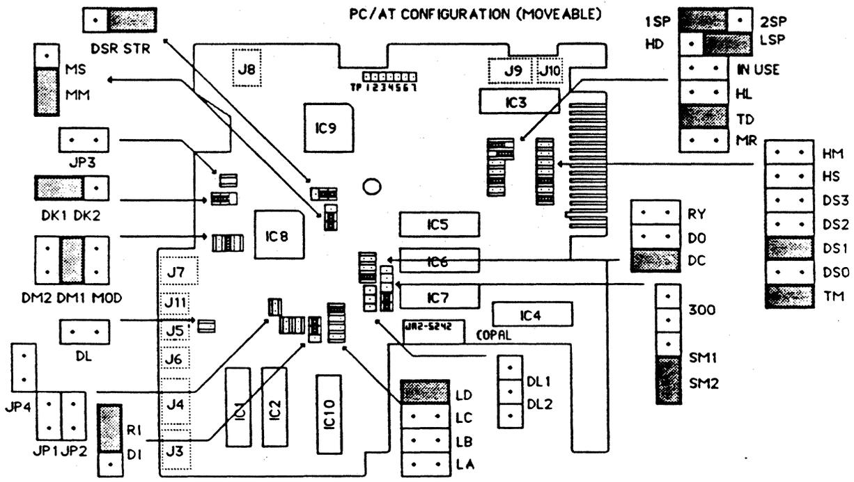
Figure 5-7 M2553/54K Revision 2 Circuit Card Layout
