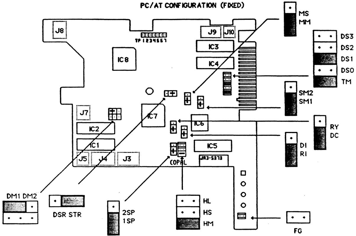
Figure 5-8 M2553K Revision 3 Circuit Card Layout
