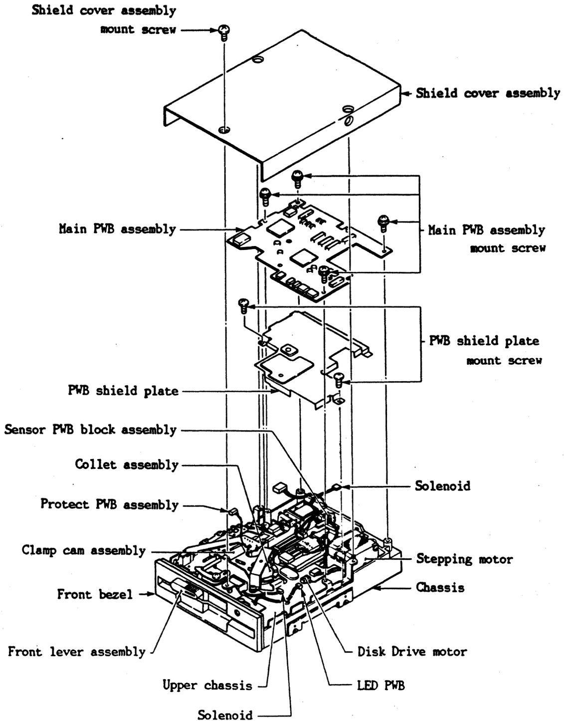
Figure 5-1 Top View of Disk Drive (View 1)
