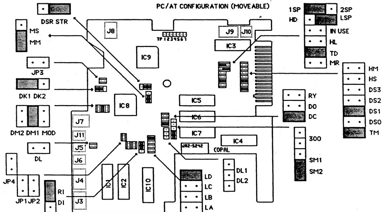
Figure 4-1A M2553K/54K Revision 2 Circuit Card - Jumper Locations
