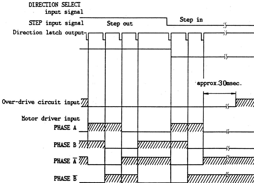
Figure 3-7 Typical Stepping Motor Control Circuit Waveforms
