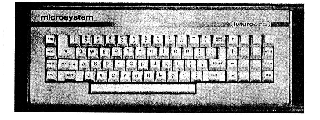
Futuredata AMDS keyboard The special keys on the left are used in text editing. The arrow keys on the right scroll or space through text (Editor) or memory (Debugger). The keys on the far right are hardware control function keys.
