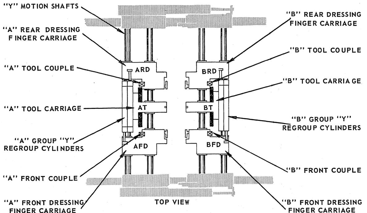
FIG. 2 - "Y" MOTION CARRIAGES AND REGROUP CYLINDERS
