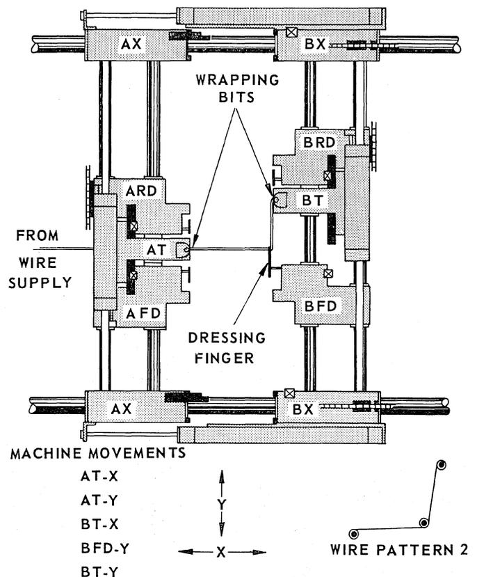
FIG. 9 - FINAL CARRIAGE POSITIONS PATTERN 2
