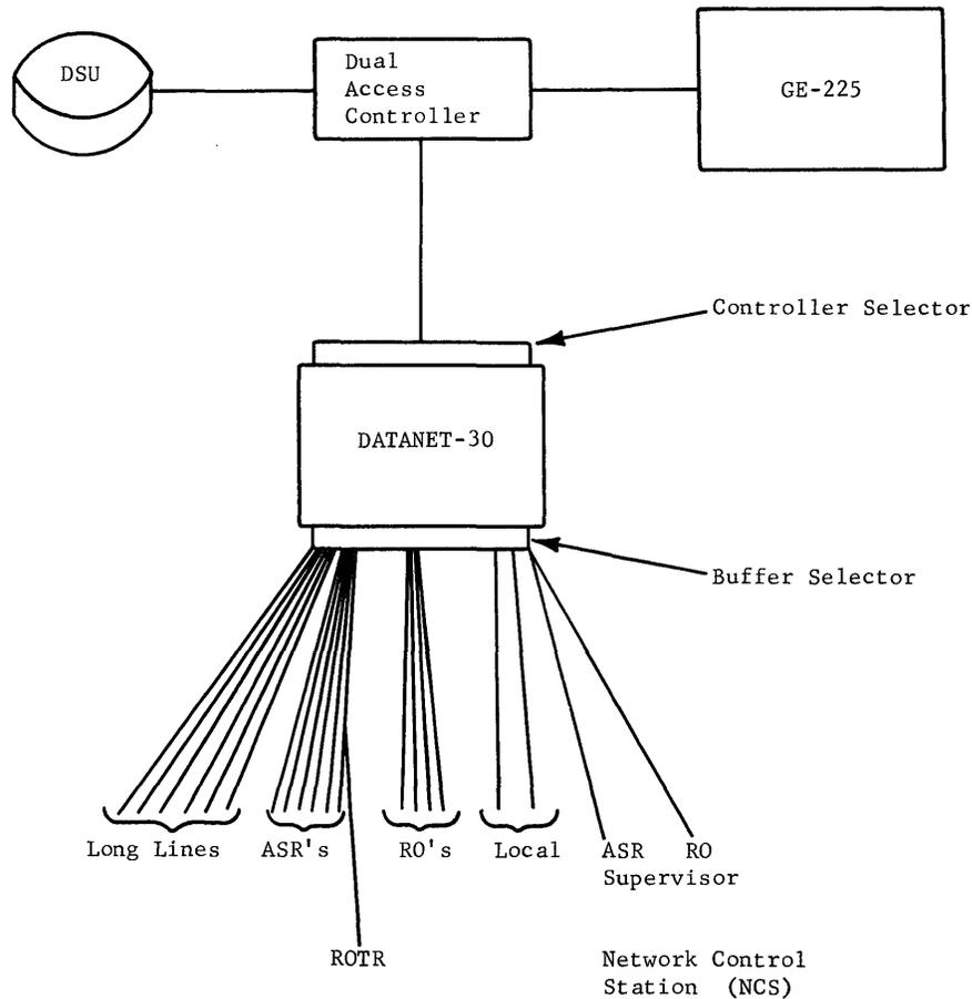
Figure 2. Relay Center Equipment Configuration
