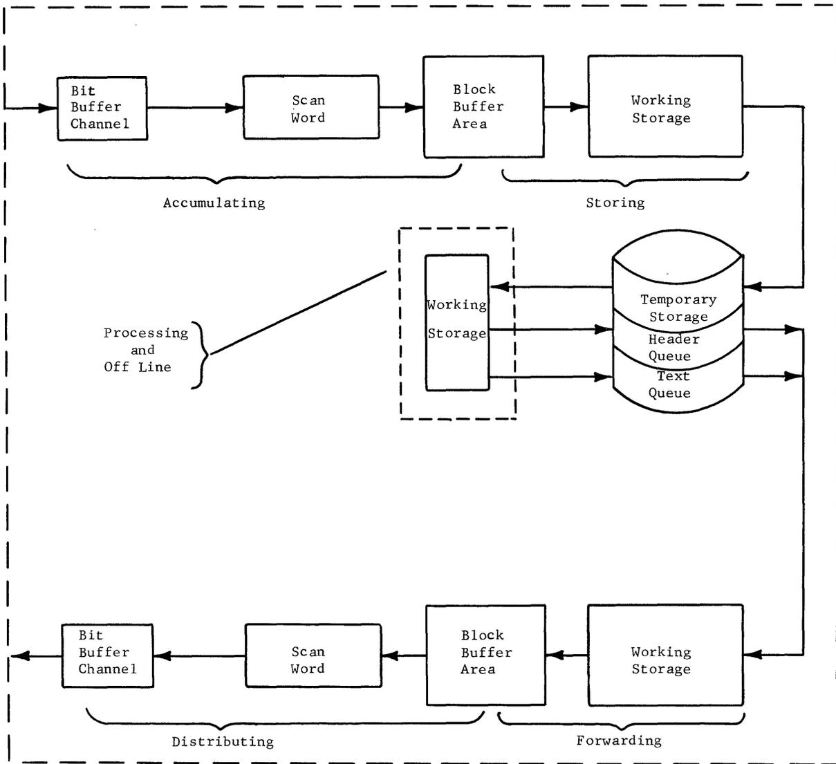
Figure 3. System Functional Block Diagram
