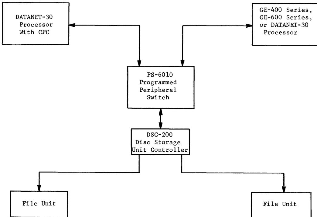
Figure 30. Typical PS-6010 Switch Application
