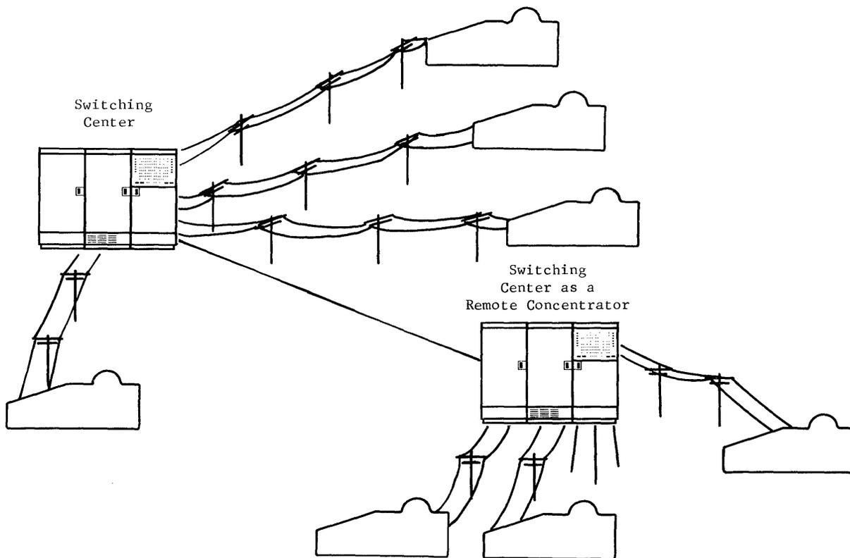
Figure 5. Communication Lines with a Remote Concentrator
