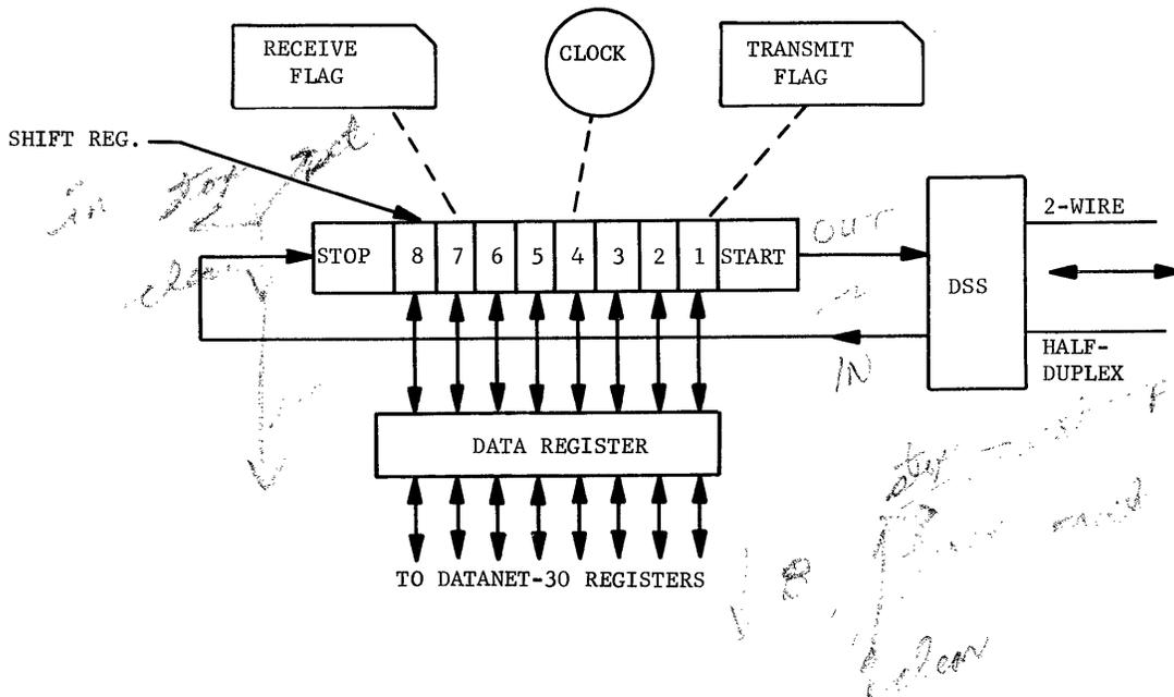
Figure 16. Character Buffer Transmit and Receive
