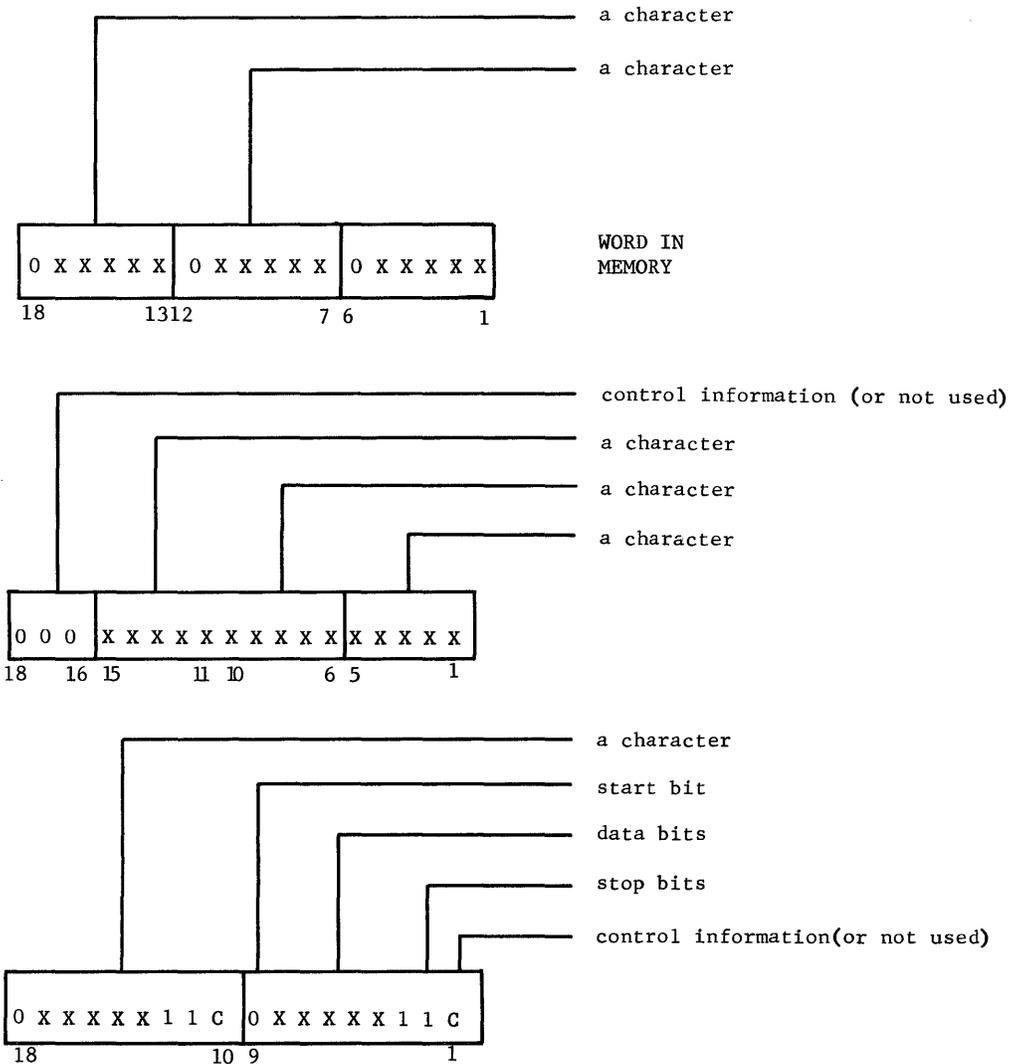
Eight-level Teletype characters can be stored conveniently in memory as six-bit characters because the DATANET-30 has special instructions to facilitate stripping off and checking the parity and control bits when a character is received and generation and insertion of parity and
