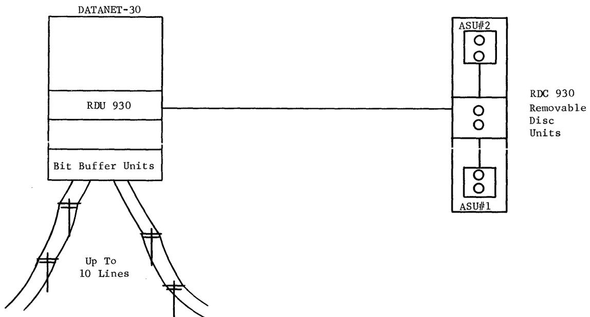
Figure 2. System with RDC 930 Units
