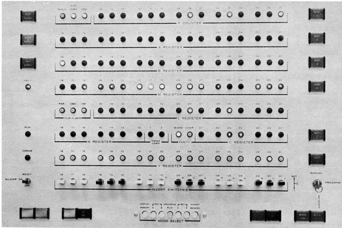
Figure 36. The Control Console
