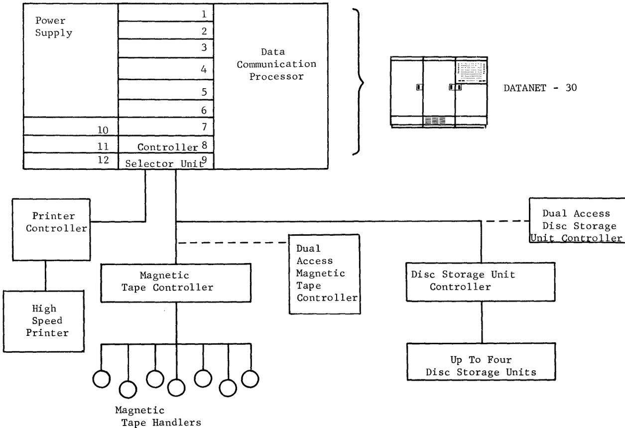
Figure 25. DATANET-30 with Controller Selector Unit and Peripheral Equipment
