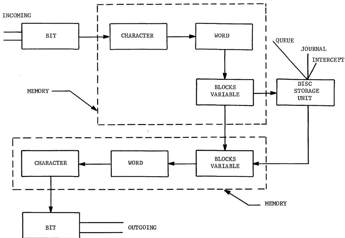
Figure 33. Data Flow Functional Block Diagram
