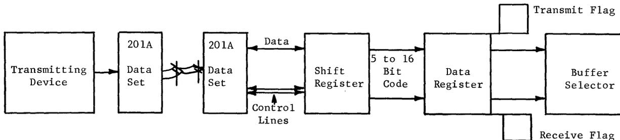
Figure 18. Character Buffer Channel Block Diagram
