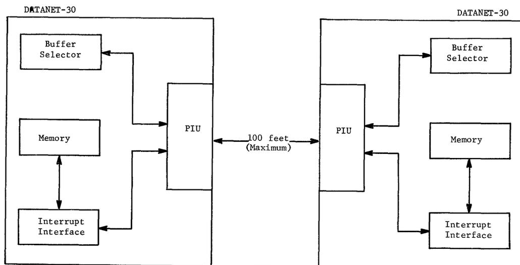
Figure 21. PIU Connecting Two DATANET-30's
