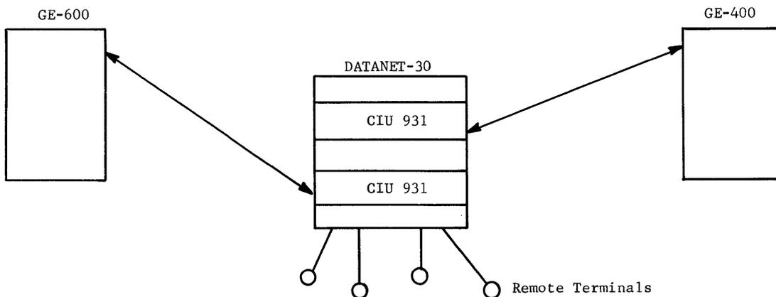
Figure 22. CIU 931 Connecting a DATANET-30 with an External Computer
