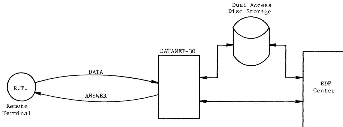
Figure 9. Remote Data Processing
