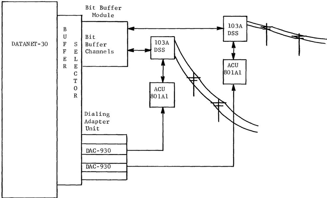
Figure 19. Dialing Adapter Units with Telephone Equipment and Bit Buffers
