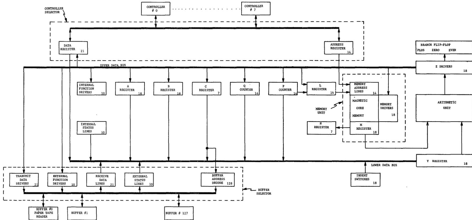
Figure 35. Detailed Block Diagram DATANET-30
