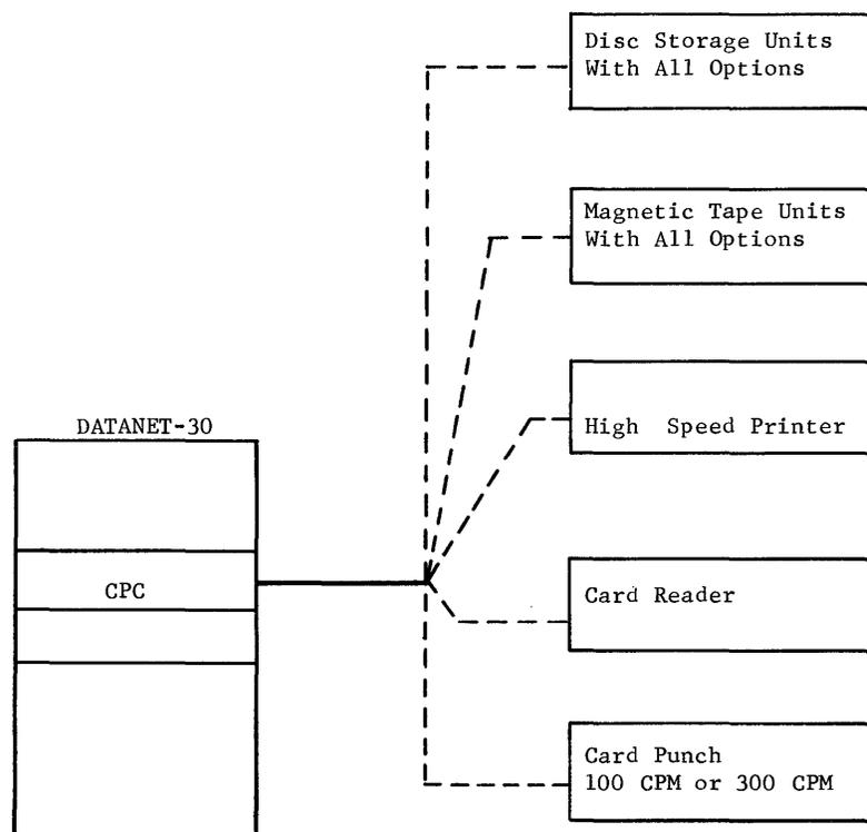
Figure 26. CPC Peripheral Equipment
