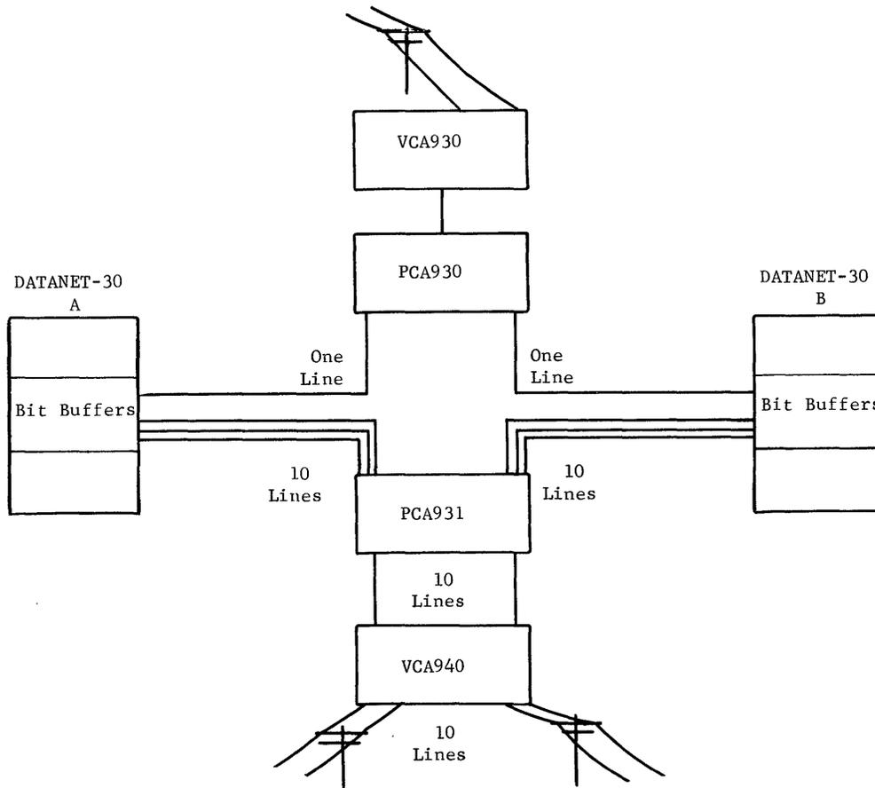
Figure 31. Parallel Channel Adapter Block Diagram
