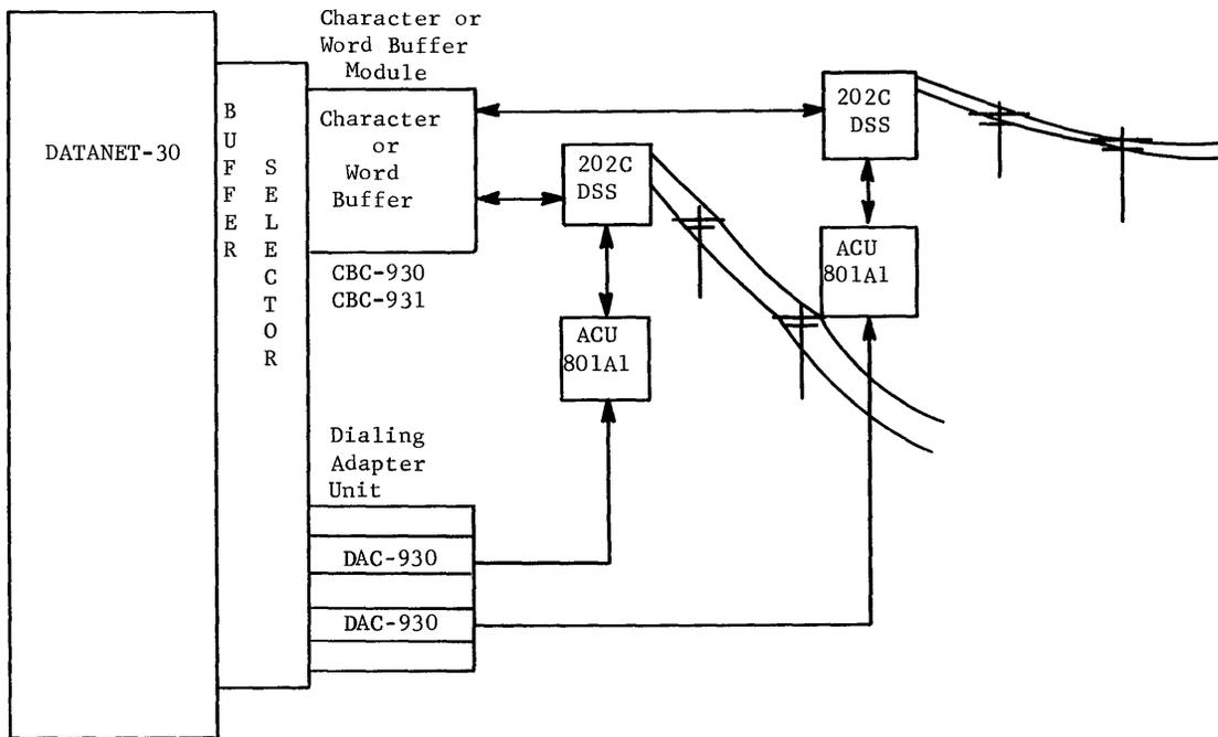
Figure 20. Dialing Adapter Units with Telephone Equipment and Character or Word Buffers.
