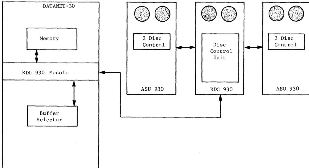
Figure 27. DATANET-30/RDC 930 Block Diagram
