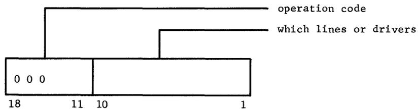
The C counter instructions have two fields plus some bits which are available for expanding the size of the C counter:
