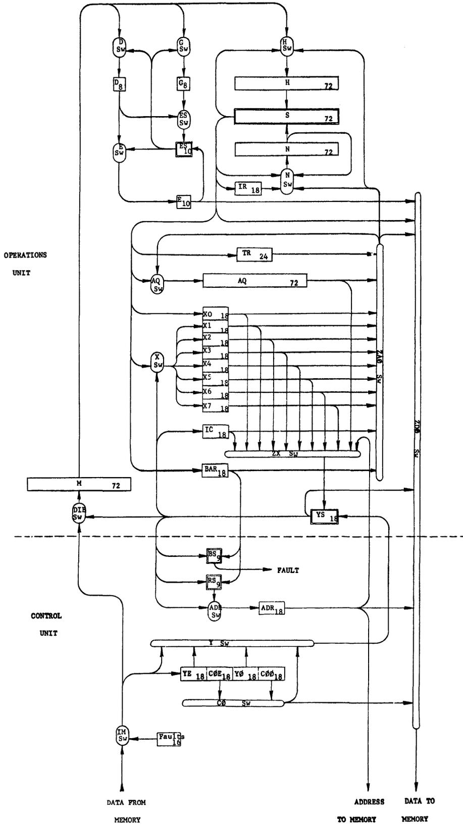
Figure II-1. Block Diagram of Principal Processor Registers
