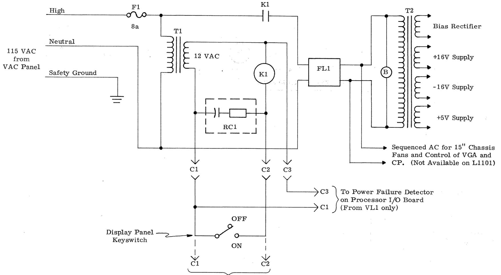
Where other VL's are to be sequenced by the same keyswitch, C1 and C2 are connected in parallel so that the switch will pick-up K1 in each supply. VL's serving Multiplexer Bus common to more than one Processor are normally not sequenced and C1 is jumpered to C2 on such supplies.
