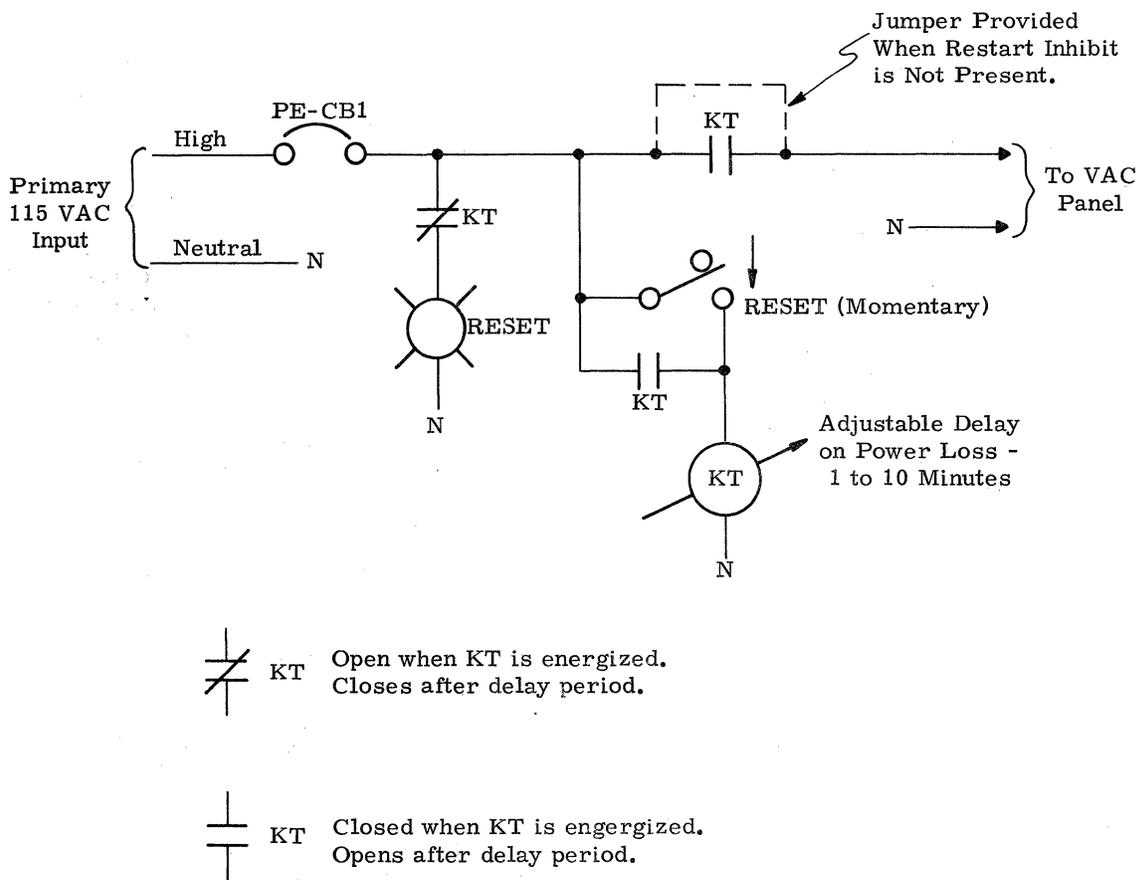
Fig. THEORY.4 Simplified Schematic, Auto. Restart Inhibit Timer
