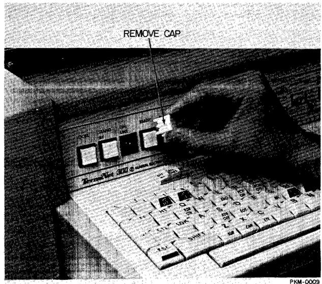
Figure 3-10. Removing Cap.
