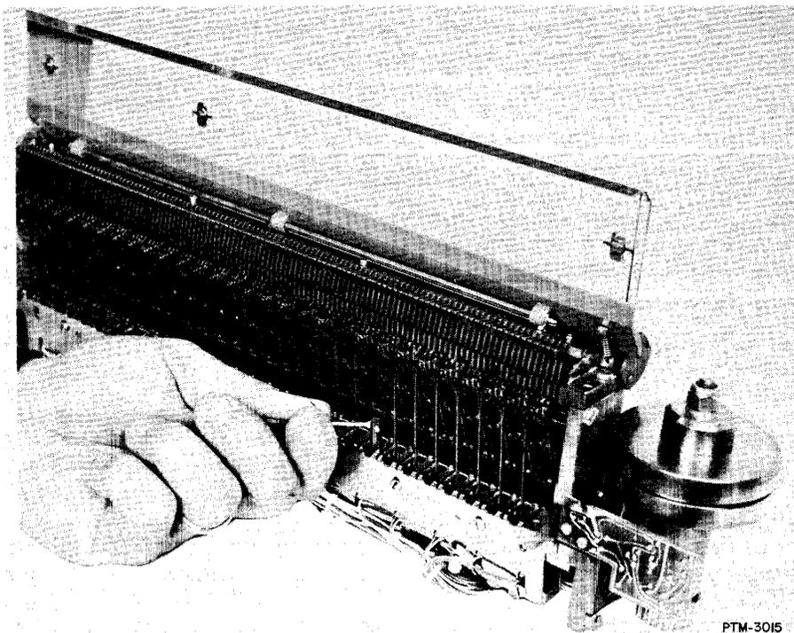
Figure 5-35. Clevis and Plunger Removal.
