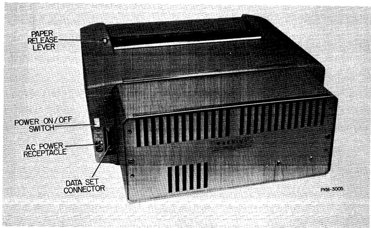
Figure 3-3. Right Rear View of Printer.
