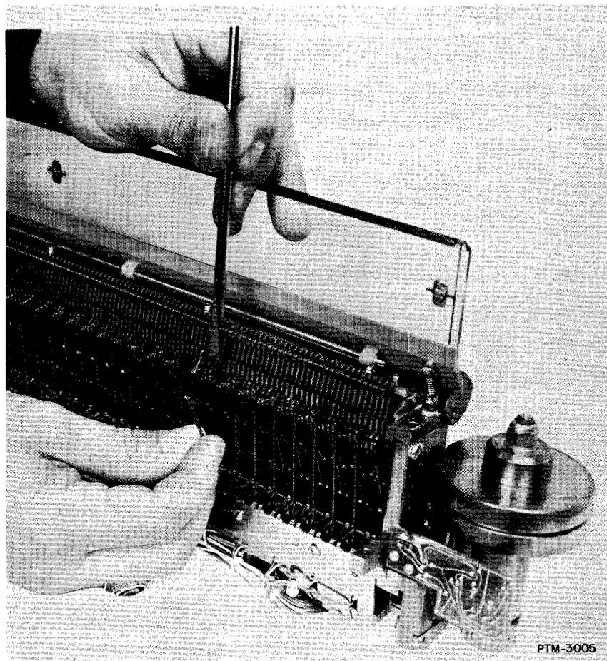
Figure 5-34. Clevis Disconnect.
