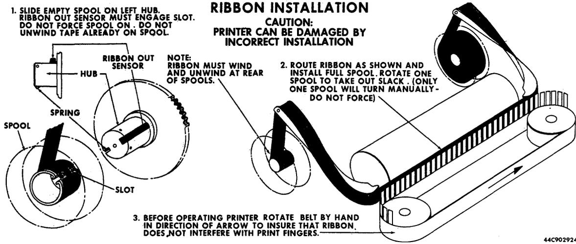
Figure 3-8. Ribbon Installation.
