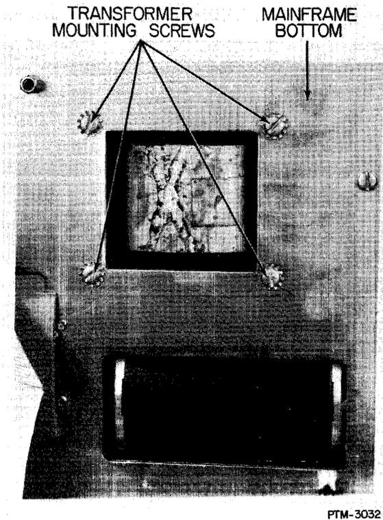
Figure 5-29. Power Transformer Mounting.
