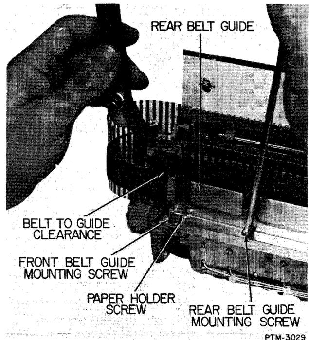
Figure 5-26. Rear Belt Guide Adjustment.
