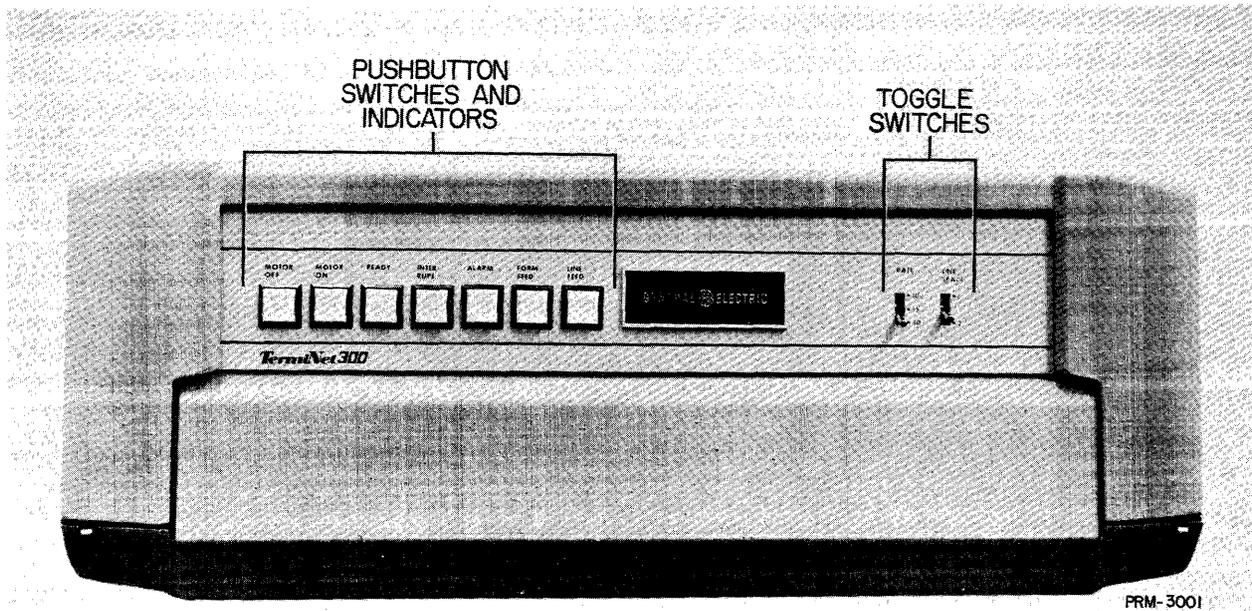
Figure 3-2. RO Control Panel
