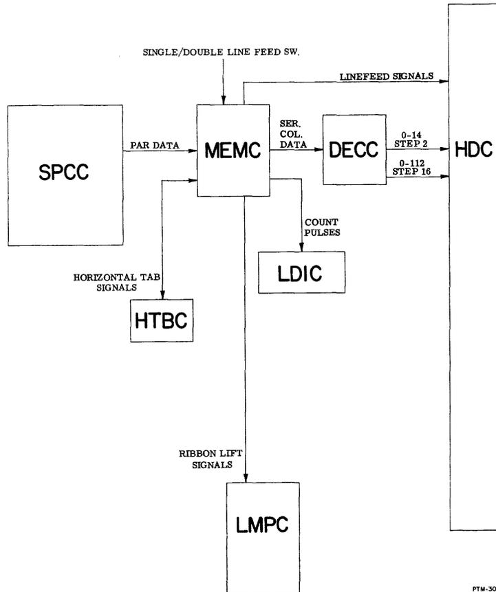
Figure 3-37. Functional Block Diagram of MEMC, DECC, HTBC, and LDIC.
