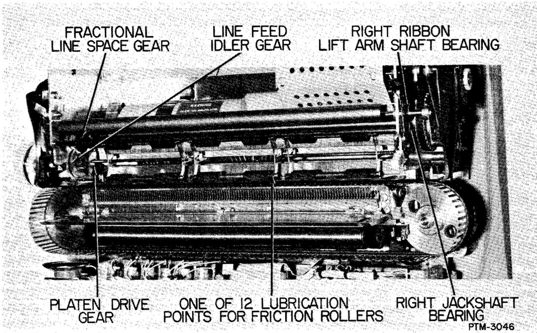
Figure 5-5. Lubrication Points - Printer Interior.
