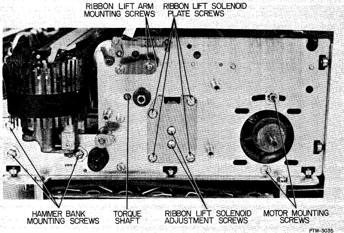
Figure 5-13. External Right Side View of Printer.
