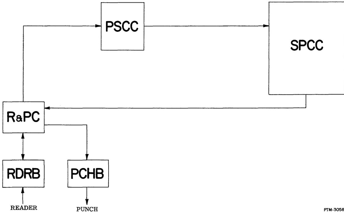
Figure 3-41. Functional Block Diagram of RDRB and PCHB
