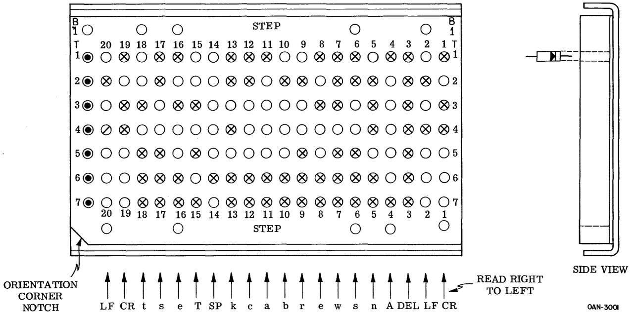
1. Diode positions are indicated with symbol ⊗ for sample message shown below block drawing.
