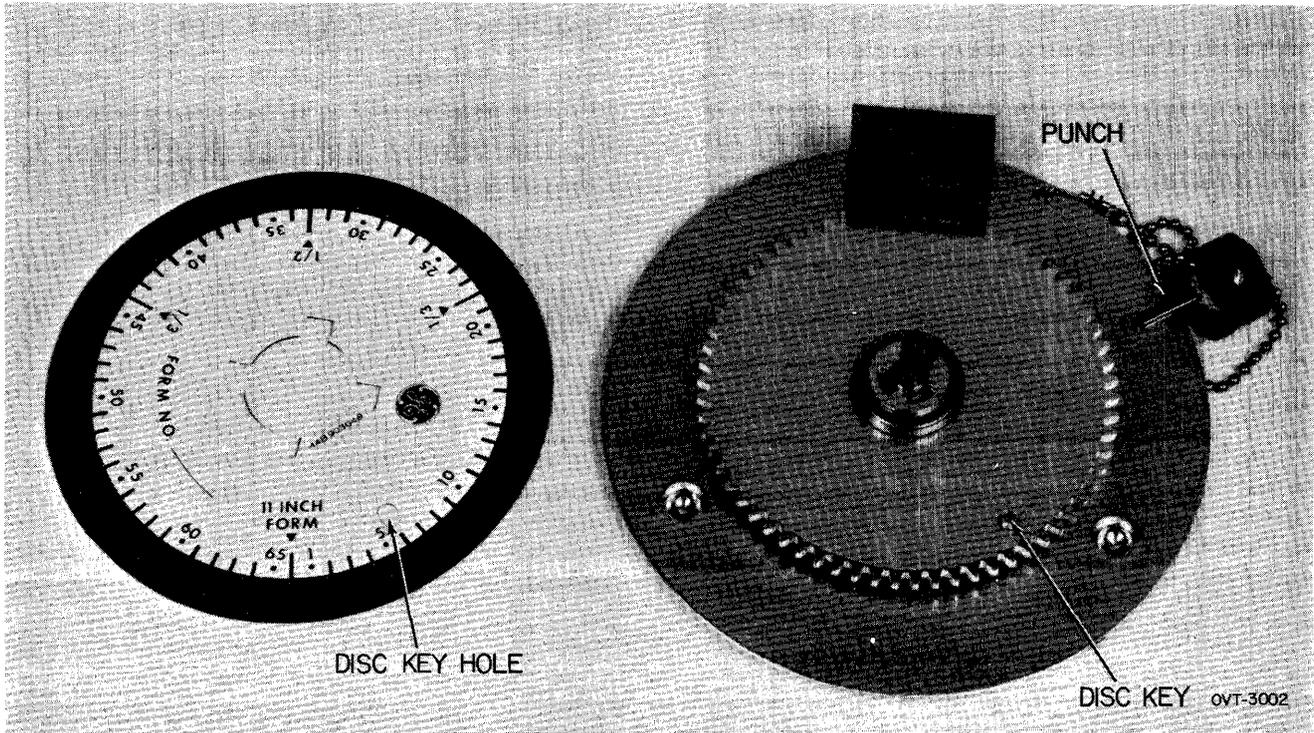
Figure 3-20. Programmable Disc and Disc Punch.
