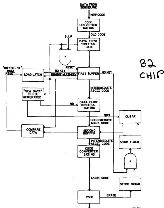
Figure 3-24. Functional Block Diagram of the Keyboard.
