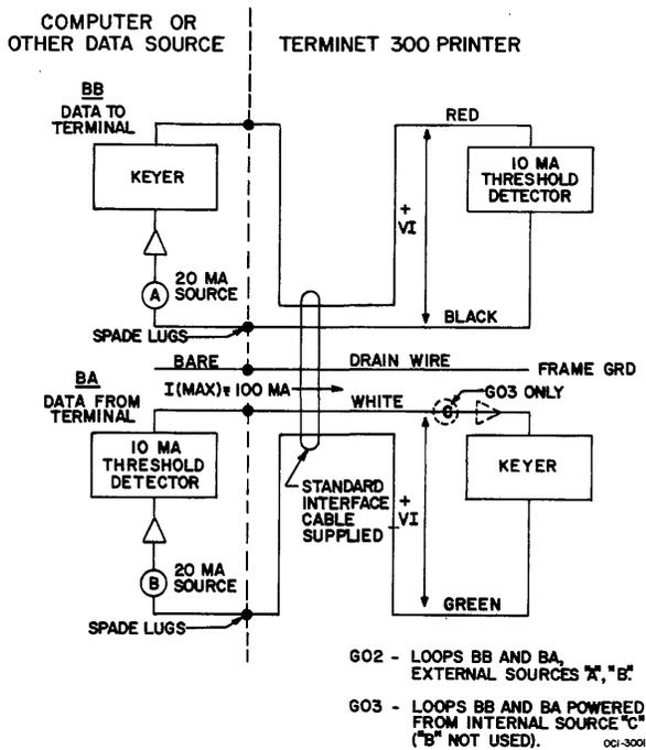
Figure 3-16. Current Loop Interface System.
