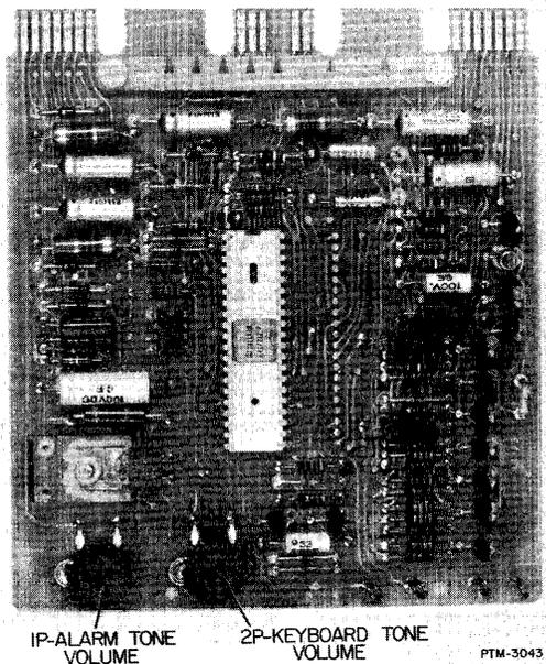
Figure 5-39. T&amp;AC Board Adjustments.
