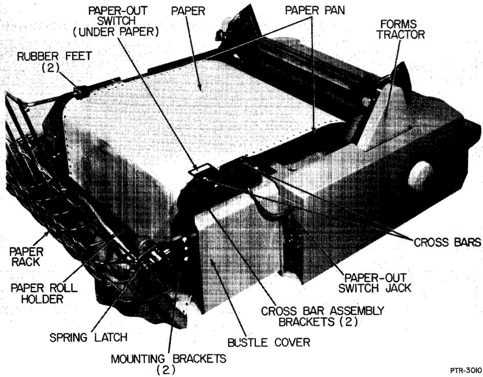
Figure 3-17. External Paper Handler Using Forms Tractor.
