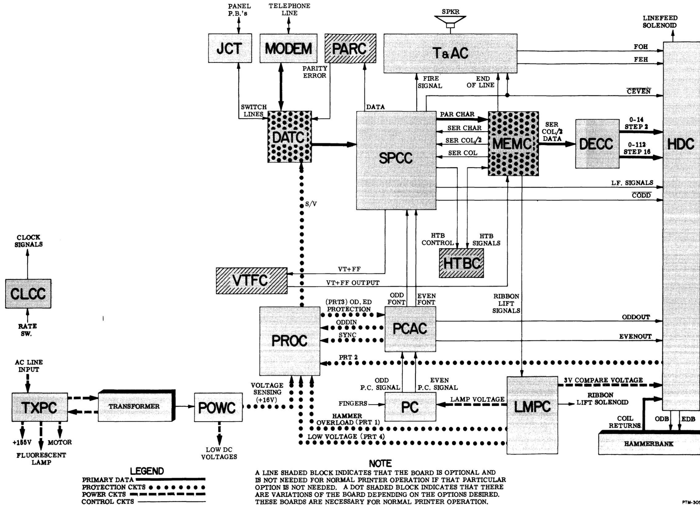
Figure 3-33. Functional Block Diagram of RO TermiNet 300 Printer
