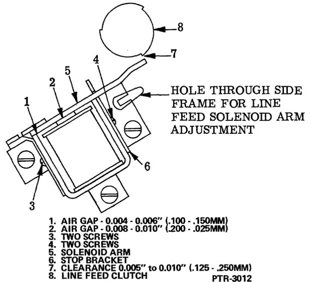
Figure 5-20. Line Feed Solenoid Adjustment.
