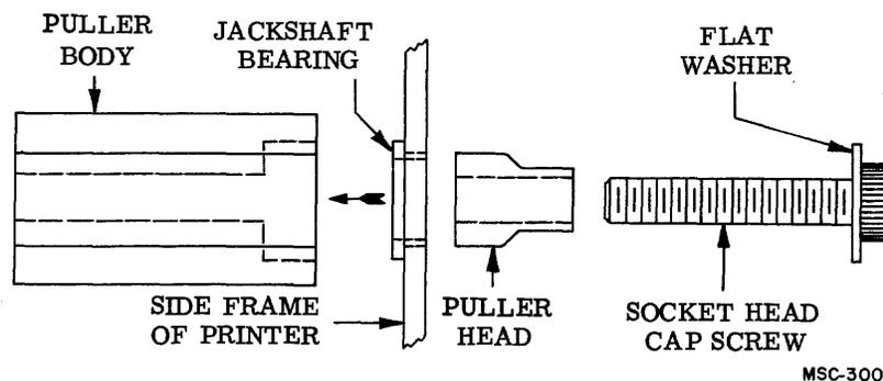
Figure 5-22. Bearing Puller.
