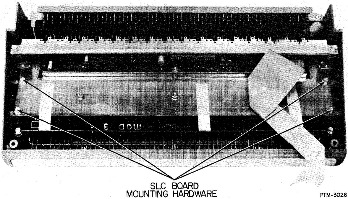
Figure 5-8. Sense Line Combined Board Mounting.
