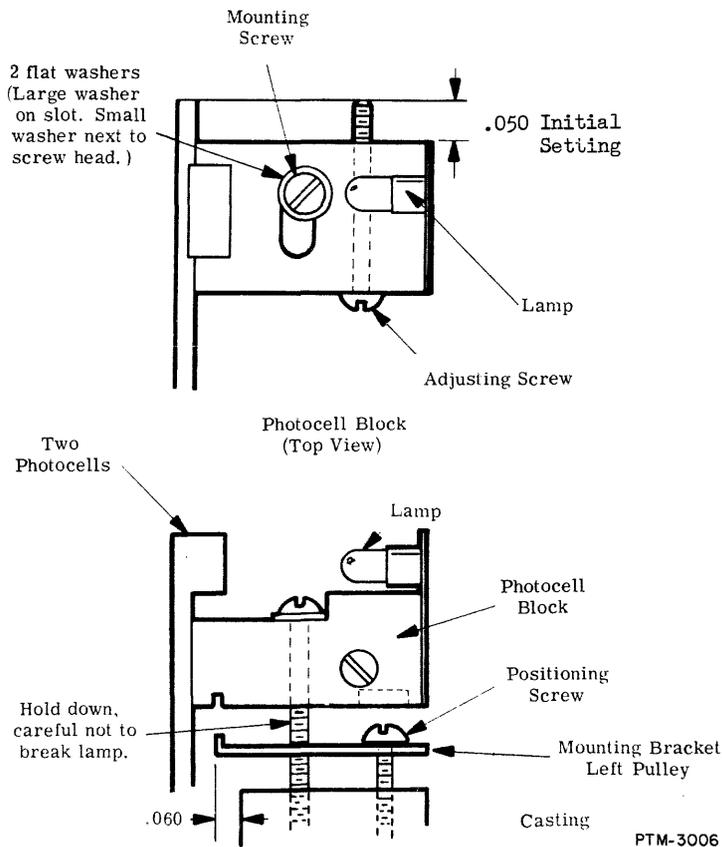
Figure 5-36. Preliminary Photocell Adjustment.
