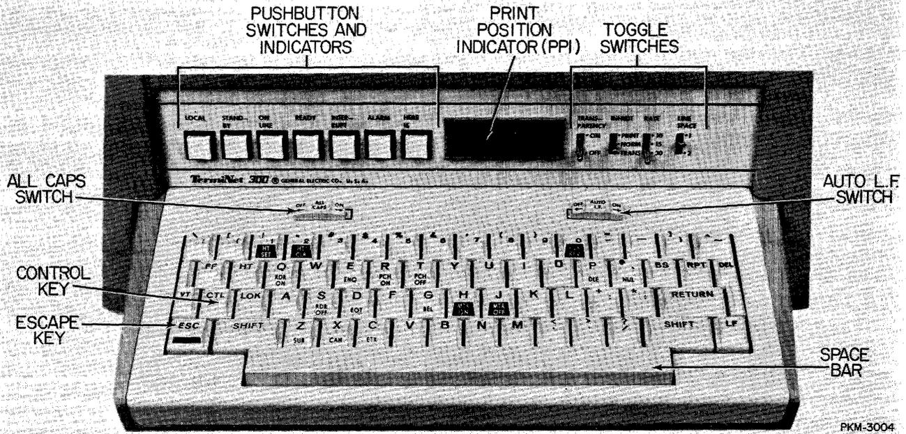
Figure 3-1. KSR Keyboard and Control Panel
