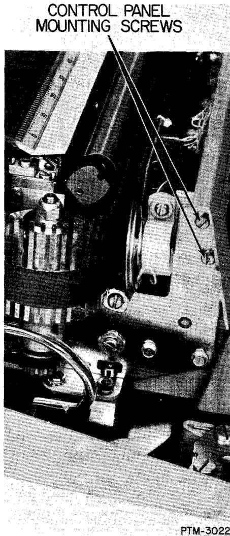
Figure 5-31. Control Panel Mounting.
