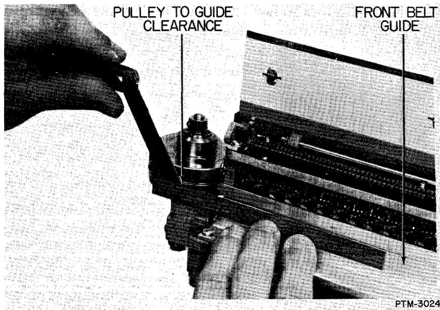
Figure 5-28. Front Belt Guide Adjustment.
