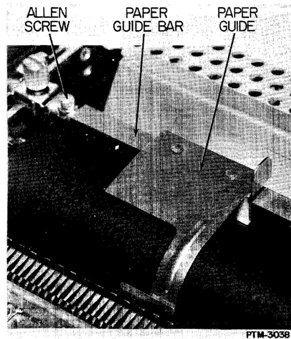
Figure 5-40. Anti-Snag Assembly.
