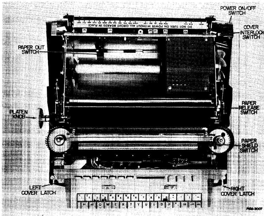
Figure 3-5. Switch Locations and Manual Controls.
