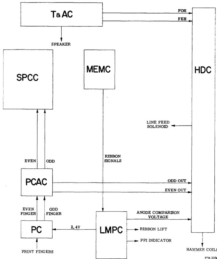
Figure 3-39. Functional Block Diagram of LMPC, PC, and PCAC
