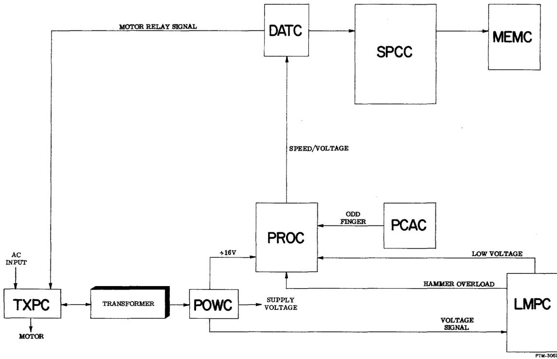
Figure 3-40. Functional Block Diagram of PROC, TXPC, and POWC
