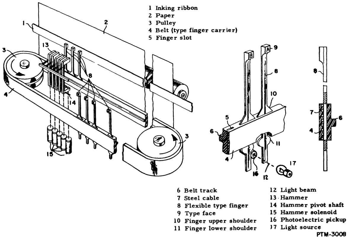
Figure 3-25. Hammer and Print Belt Assembly.
