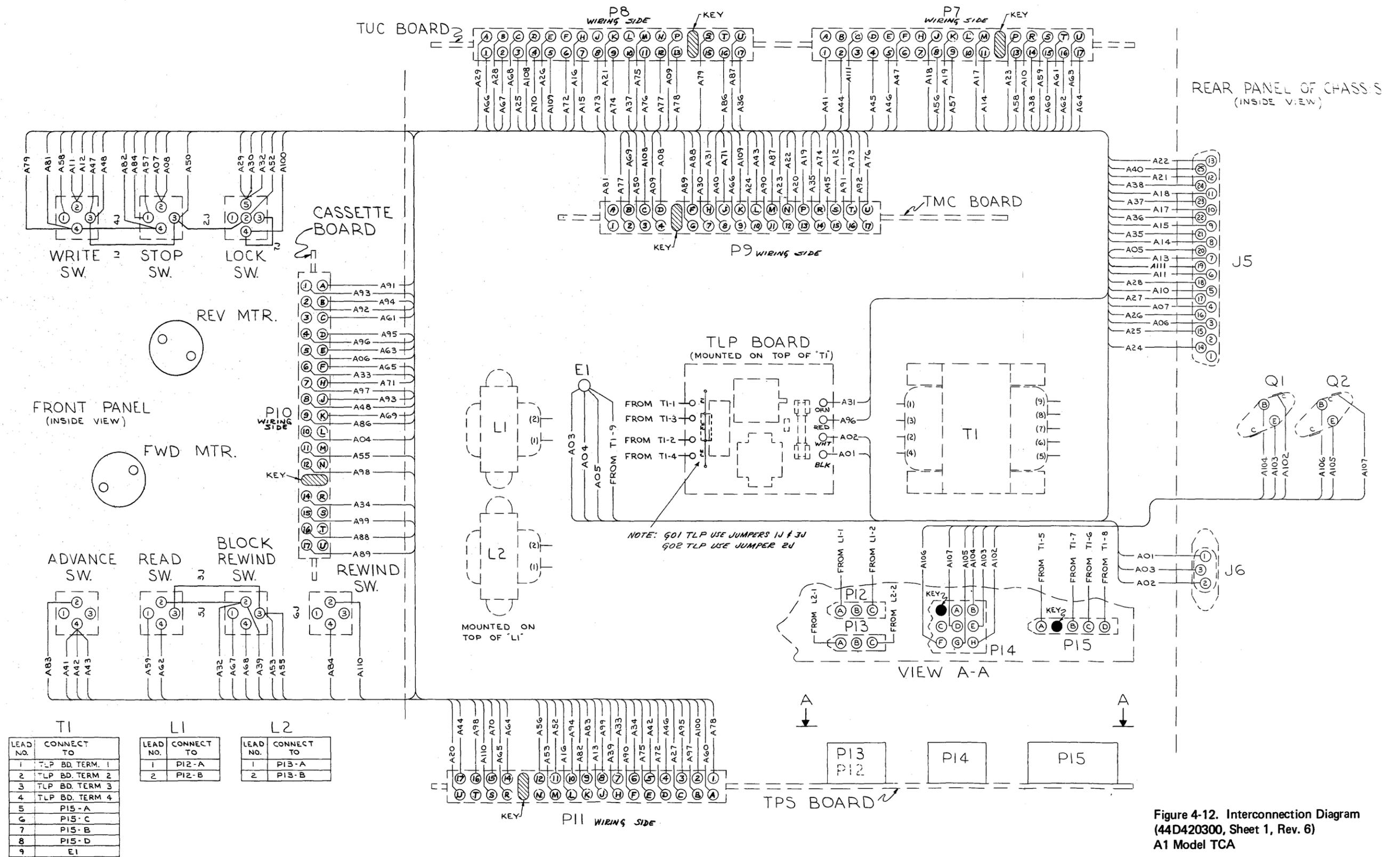
Figure 4-12. Interconnection Diagram (44D420300, Sheet 1, Rev. 6) A1 Model TCA
