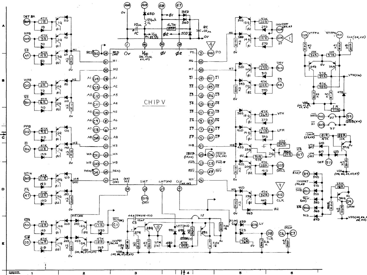
Figure 4-2. TRP/1 Printed Circuit Board (44C420203-G01, Rev. 3) - A1 Model TCA
