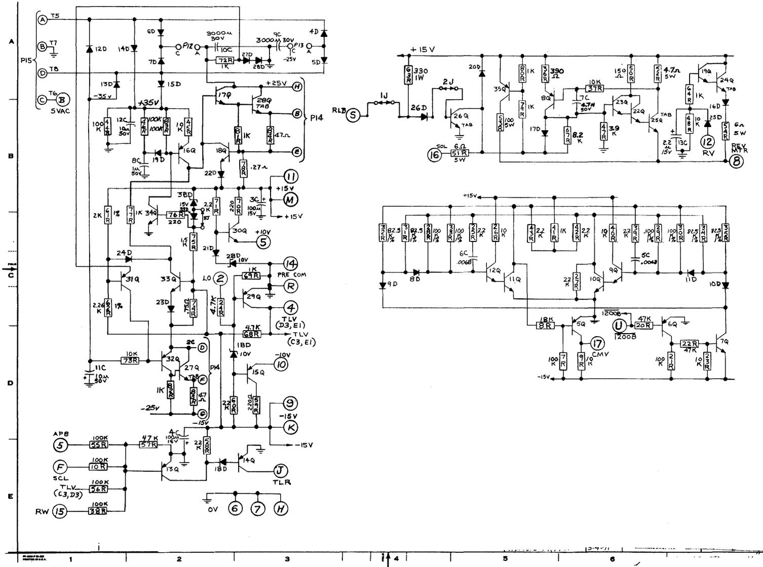
Figure 4-5. TPS/1 Printed Circuit Board (44C420202, Rev. 11) - A1 Model TCA
