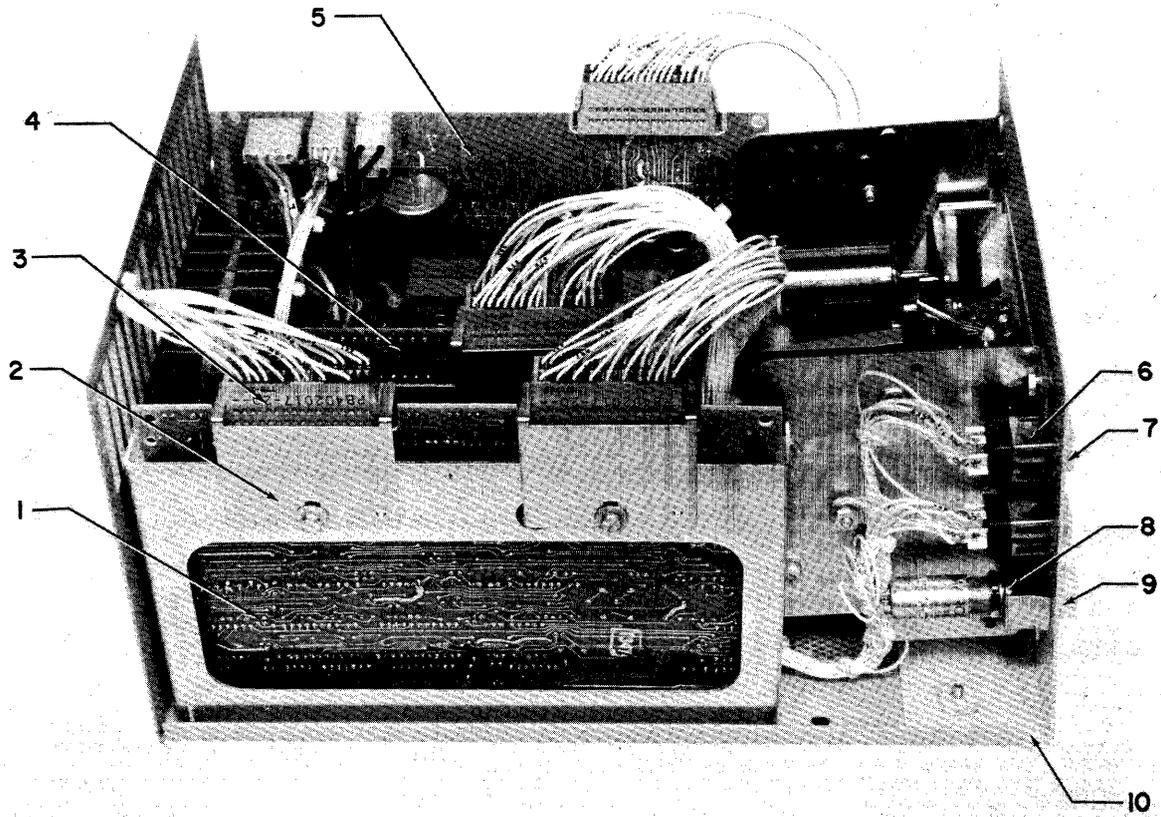
Figure 6-1. Printed Circuit Boards and Connectors and Brackets
