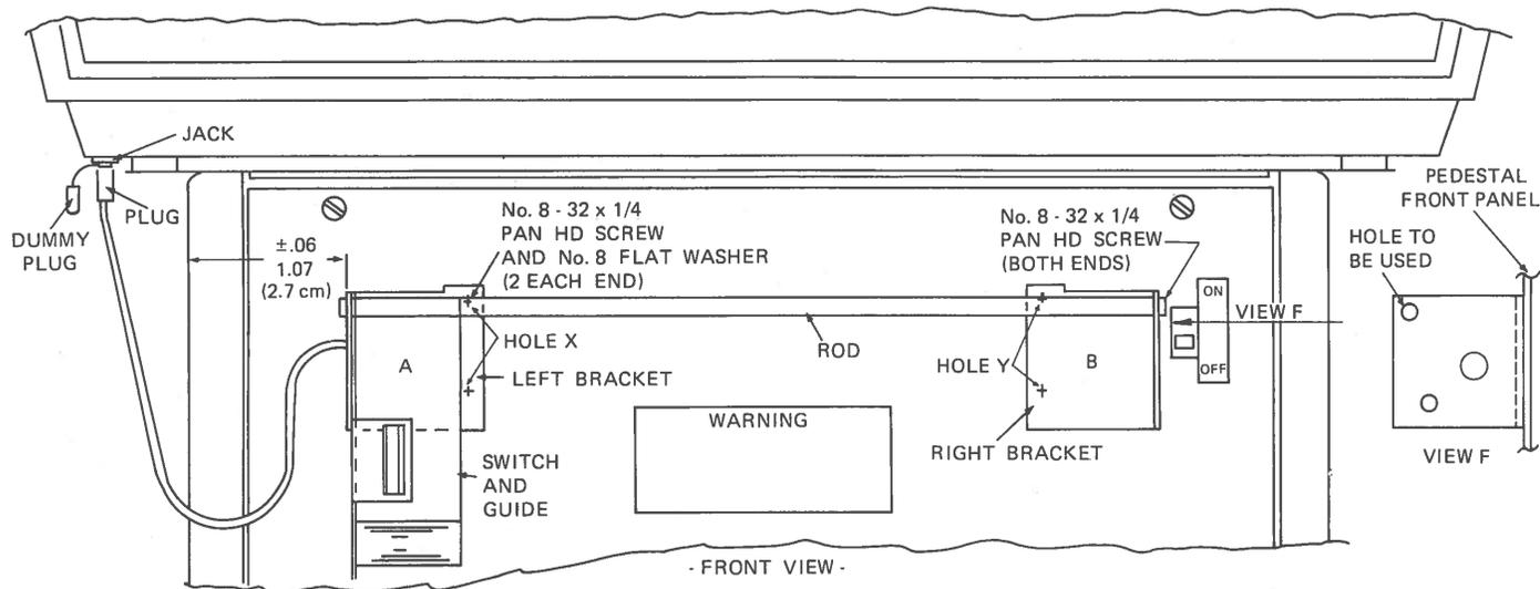
Installation of Optional Front Paper Low Switch Kit
