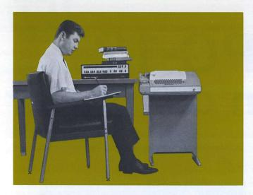
The SPC-12 Automation Computer is a new kind of digital computer—designed to work in an industrial climate, unattended and around the clock. Industrial reliability is assured by the SPC-12's worst case design, its wire-free construction, its use of integrated circuits, its wide-temperature (Lithium) memories, and its exhaustive environmental testing and factory burn-in procedures. It can be operated and maintained by non-technical personnel.
