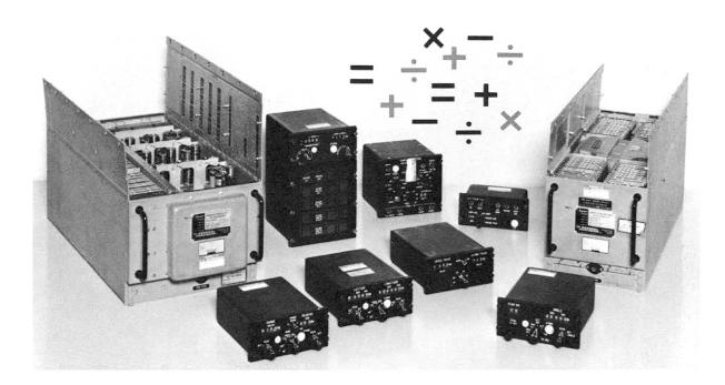
A general-purpose digital computer system performing complex real-time computing and control operations, this Kearfott-designed equipment, originally produced for automatic navigation in the C-141 aircraft, quickly demonstrated its adaptability to other applications including space guidance and control as the GPK-33.
