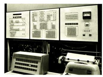
Close-up of control panels for CPU subsystem is shown in photo above. Controls on panel at right are arranged conveniently for use by operator. Banks of indicator lamps on other panels display status of peripheral devices and programs.
