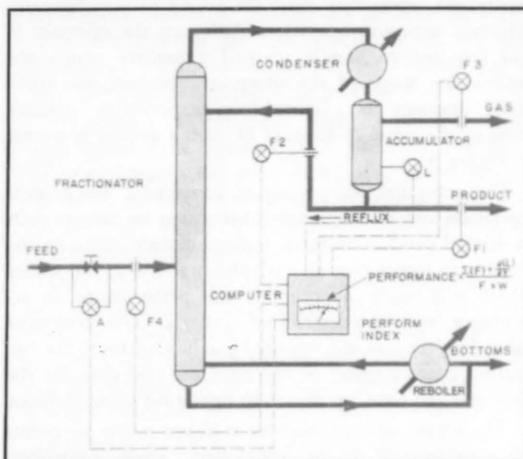
Figure 3. Diagram of Southwestern Industrial Electronics analog computer installed on Humble fractionating tower to provide tower performance index readings. (See ISAJ, April '59, page 56.)
