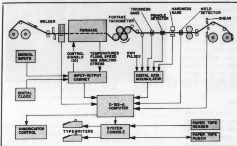
General Electric's concept of a computer control installation for a continuous annealing line.
