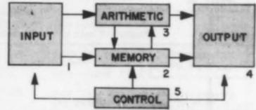
(4) **Output.** Path for data out of computer. Common output units are: typewriters, printers, digital-to-analog converters, digital displays, magnetic tape and punched tape.
