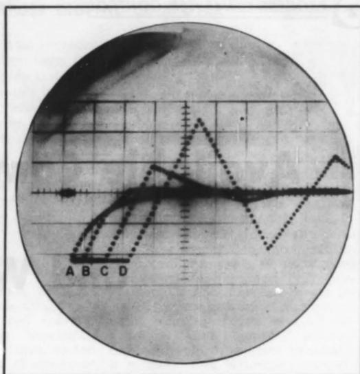
Figure 7. Oscilloscope view of a simulated control system error signal in response to decreasing sampling rates. Curve A shows error signal with continuous analog controller (proportional response) with step change in set point. Curves B, C & D show increased instability of same system with a sampled data controller (same settings) as sampling rate is decreased.
