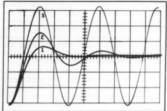
Figure 9. Analog computer results of solution of the equation shown in Figure 6, showing the effect of air resistance or damping.
