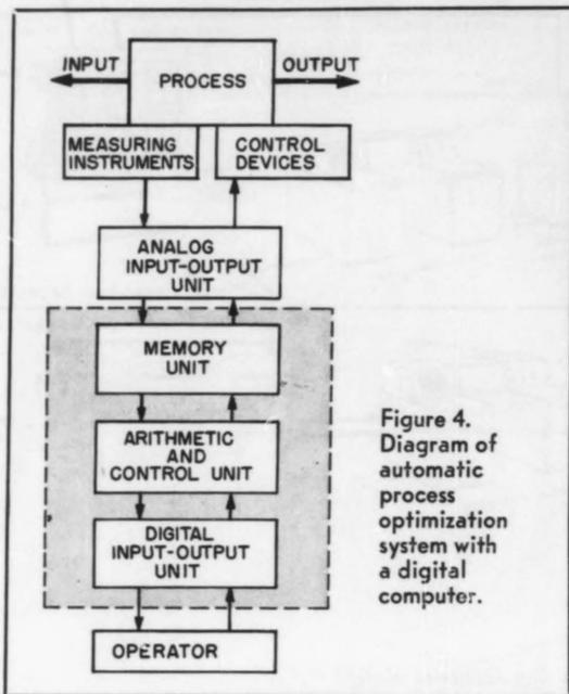
Figure 4. Diagram of automatic process optimization system with a digital computer.
