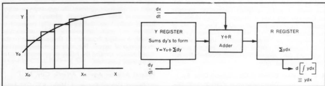
Figure 10. Block diagram of digital integrator used in the digital differential analyzer and approximation of the integral by summation. (Courtesy, Litton Industries.)
