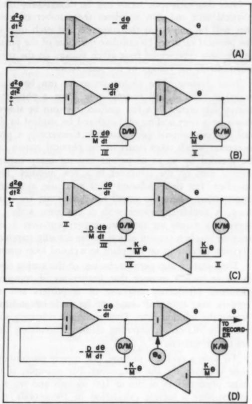
Figure 7. Analog circuit development for solving the typical second order differential equation representing the system shown in Figure 6.
