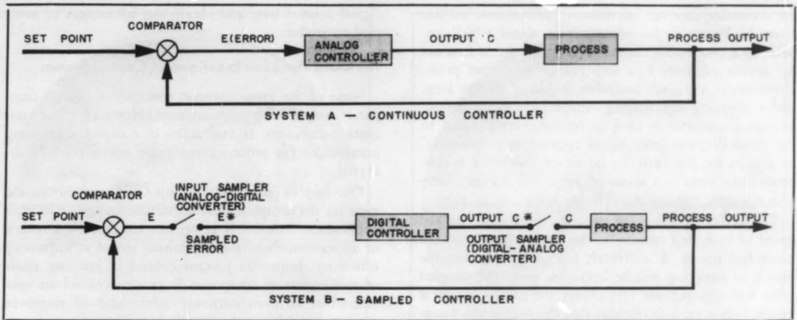
Figure 5. Comparative diagrams for a process control system employing continuous analog signals and one employing a digital controller using sampled data input.
