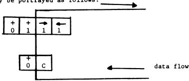
The modification(s) to data as it passes from one register to another is specified by the MOD portion of the data transmission instruction. If no modification is selected (MOD = 0000), then data passes through the two +0 paths, which results in a direct 16-bit parallel transfer. The FAST key words (2.3) used to specify modifications to data are:
