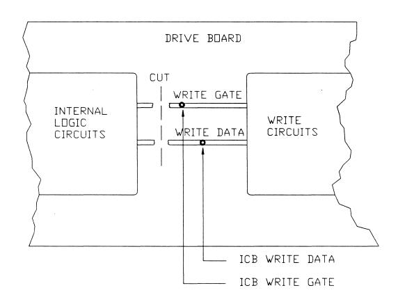
FIG. 7.1: WRITE SIGNAL CONNECTION (TRACES)
