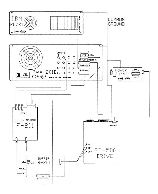
FIG. 4.1: ST-506 CONNECTION DIAGRAM
