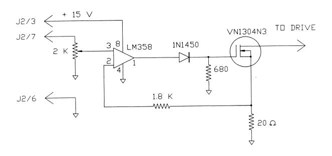
FIG. 13.2: CURRENT SOURCE CONVERTER (TO CURRENT)
