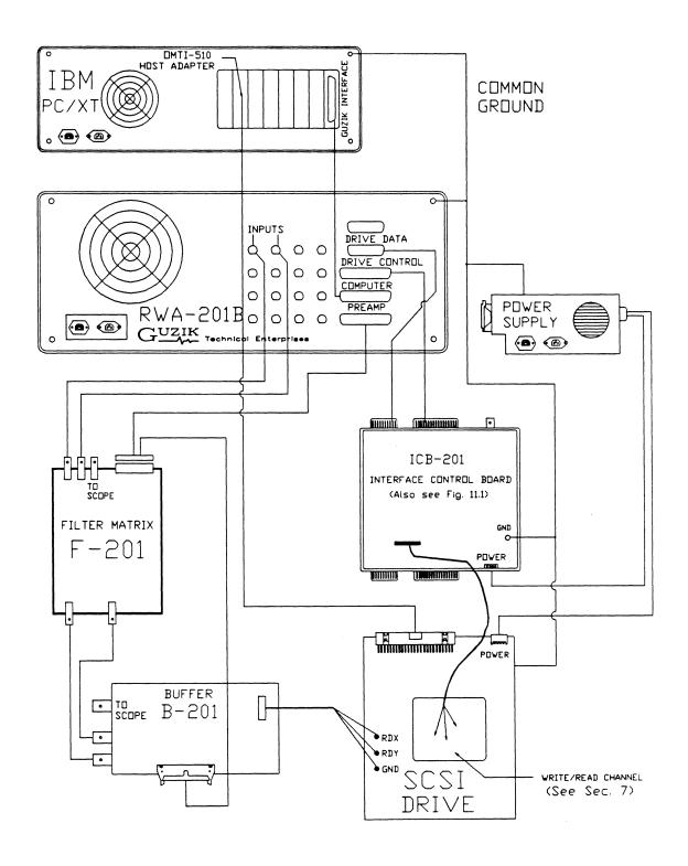
FIG. 4.3: SCSI CONNECTION DIAGRAM
