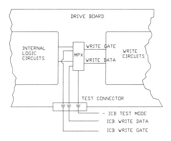
FIG. 7.4: WRITE SIGNAL CONNECTION (MULTIPLEXED)
