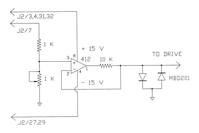
FIG. 13.1: CURRENT SOURCE CONVERTER (TO VOLTAGE)
