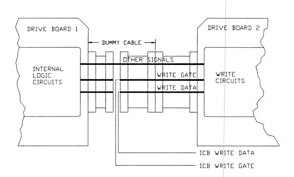
FIG. 7.2: WRITE SIGNAL CONNECTION (DUMMY CABLE)
