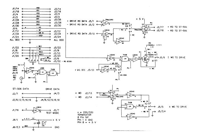
FIG. 11.2: INTERFACE CONTROL BOARD ICB-201 (SCHEMATIC)
