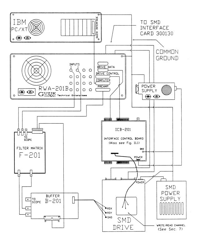
FIG. 4.4: SMD CONNECTION DIAGRAM
