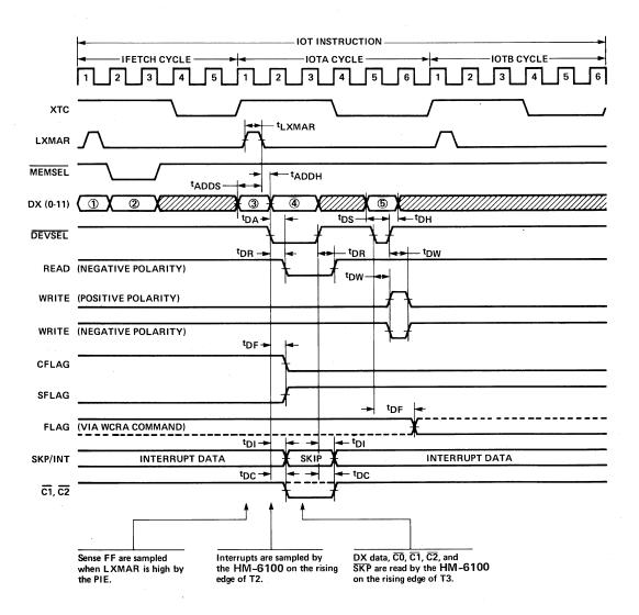
All PIE timing is generated from HM-6100 signals LXMAR DEVSEL, and XTC. No additional timing signals, clocks, or one shots are required. Propagation delays, pulse width,
