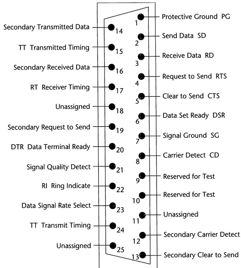
The physical connector as well as the pin numbers of the end of the cable on the DTE side will vary according to the DTE's serial port.
