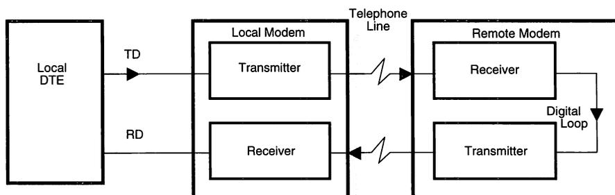
Before initiating remote digital loopback, establish a connection with a remote modem. Then, enter the command state and issue the **&T6** command to begin the test.
