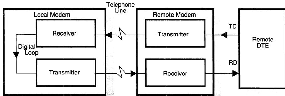
To begin local digital loopback, establish a connection with a remote modem, then enter the command state and issue the **&T3** command.
