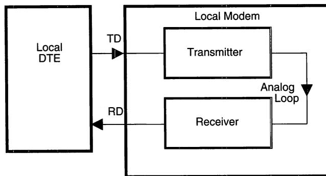
Set the local computer to echo characters and the local modem to echo commands received from the local computer (the **E1** option selected). Initiate the test with **&T1**. Type a few sentences; they will be looped back to the local computer.
