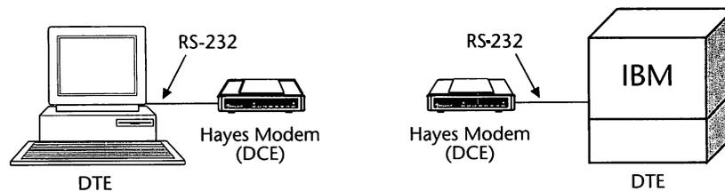
Hayes modems support the electrical portion of the RS-232 standard completely. However, signal definition varies from modem to modem.
