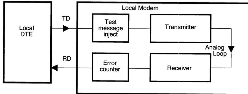
Set the computer to echo characters and the local modem to echo commands received from the computer (the **E1** command selected). Initiate the test with **&T8**. When the test is terminated, with the **&T0** command, the modem will return a three-digit test result (e.g., 000=no errors, 012=12 errors). If the error count reported is 000, the local modem passed the test. An error count of 255 indicates that 255 or more errors were detected.
