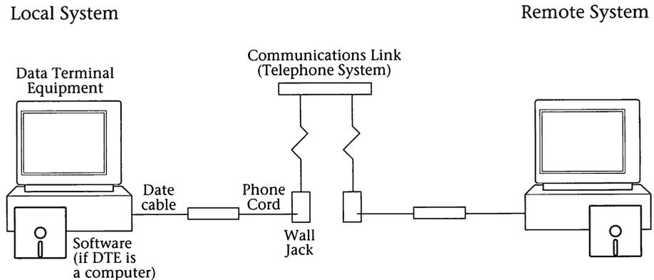
The configuration above represents the communication link as discussed in this section. Although your modem may be an internal one, that is, installed inside the computer, the operational concepts are still the same.
