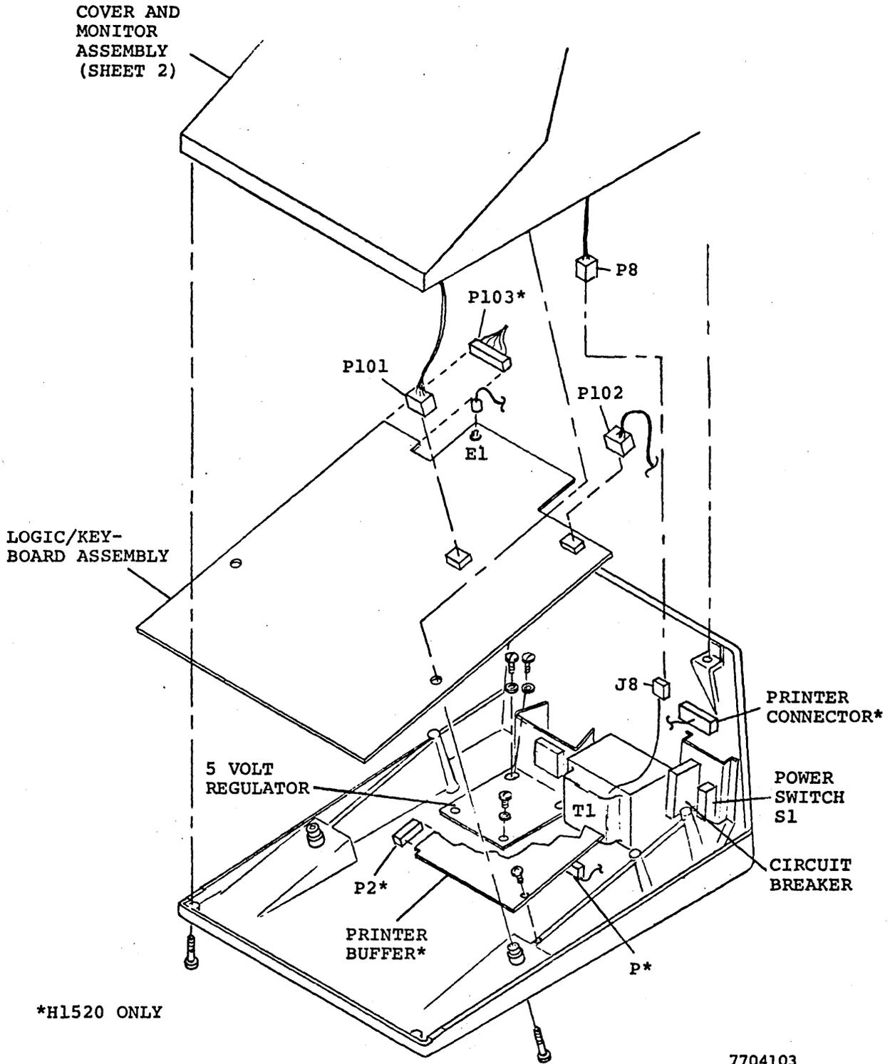
Figure B-1. Terminal, Exploded View (Sheet 1 of 2)
