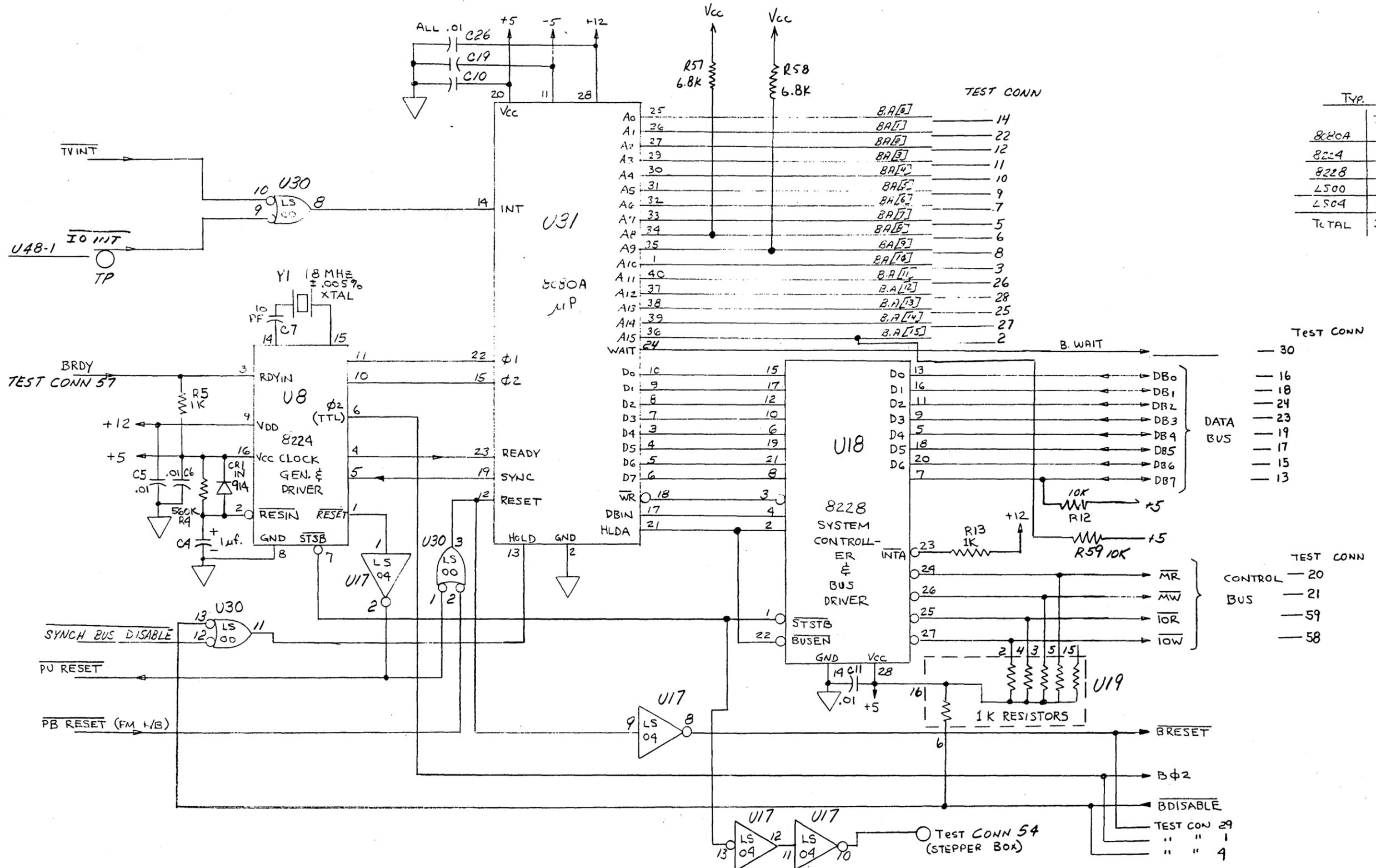
Figure B-5. Logic/Keyboard Assembly, Schematic Diagram (Sheet 1 of 9)
