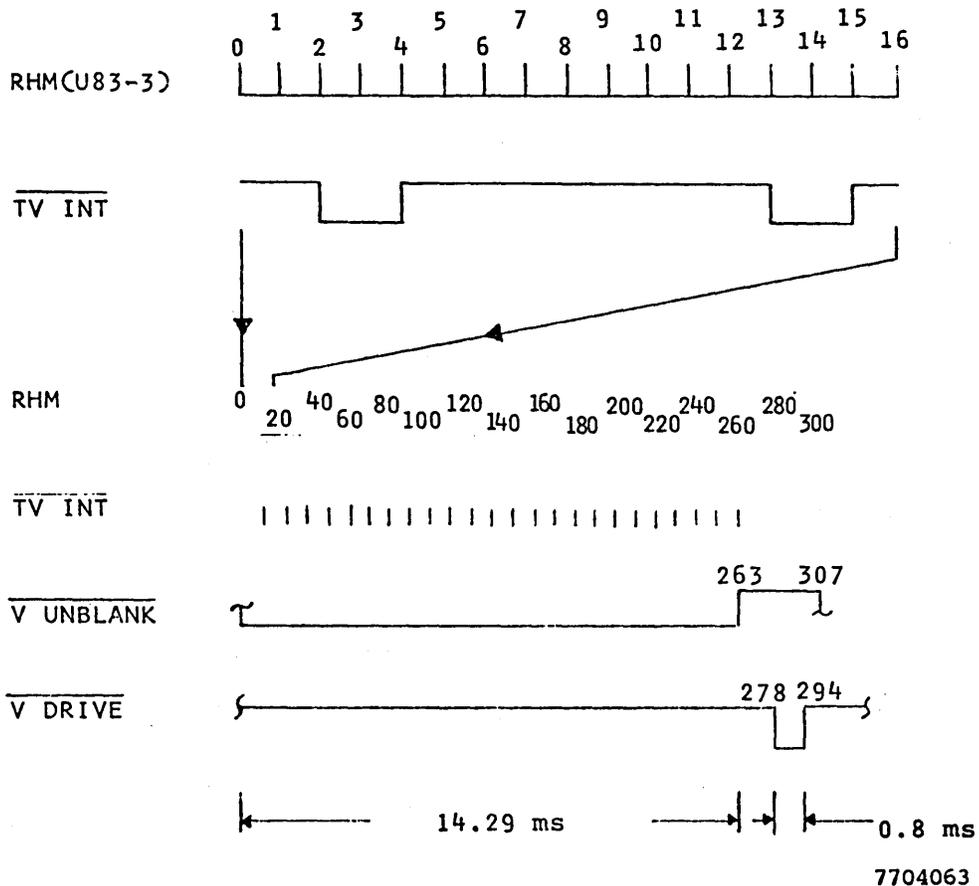
Figure 1-11. Vertical Timing
