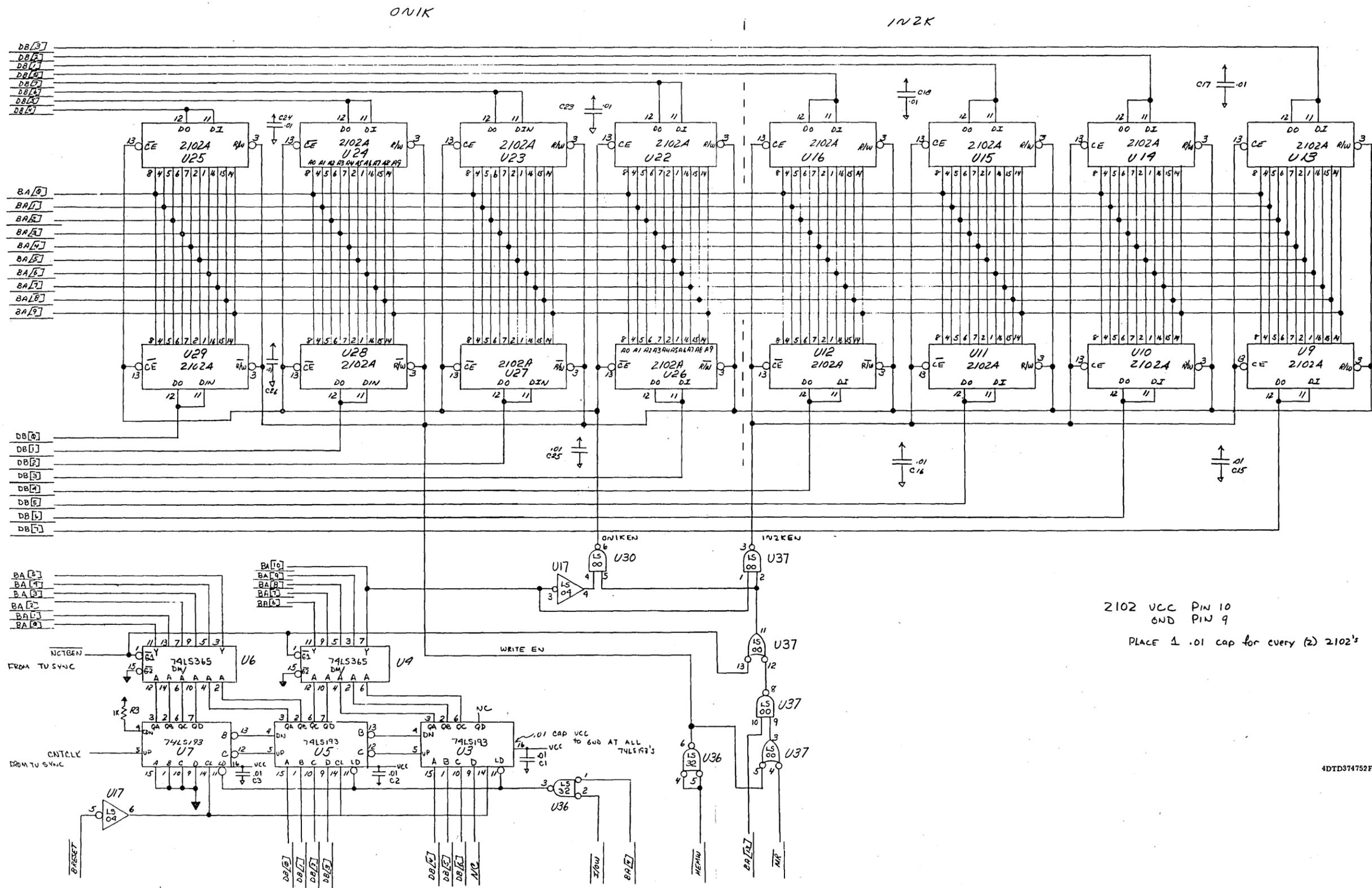
Figure B-5. Logic/Keyboard Assembly, Schematic Diagram
