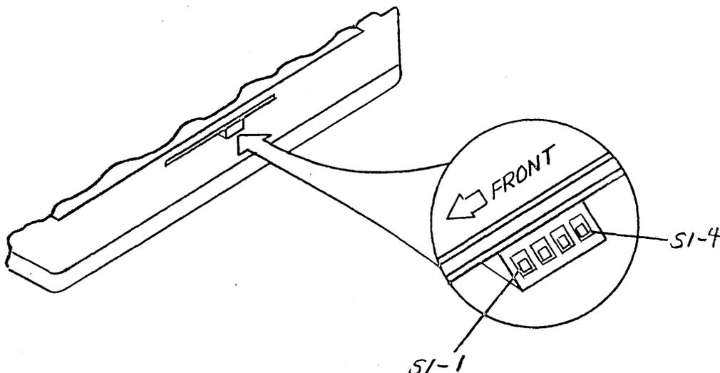
Figure 1-2. Switch S1 on Printer Buffer
