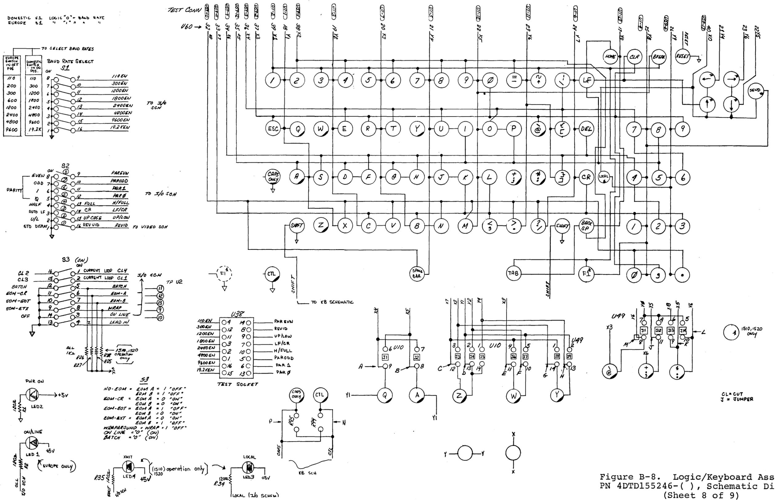
Figure B-8. Logic/Keyboard Assembly PN 4DTD155246-(), Schematic Diagram (Sheet 8 of 9)
