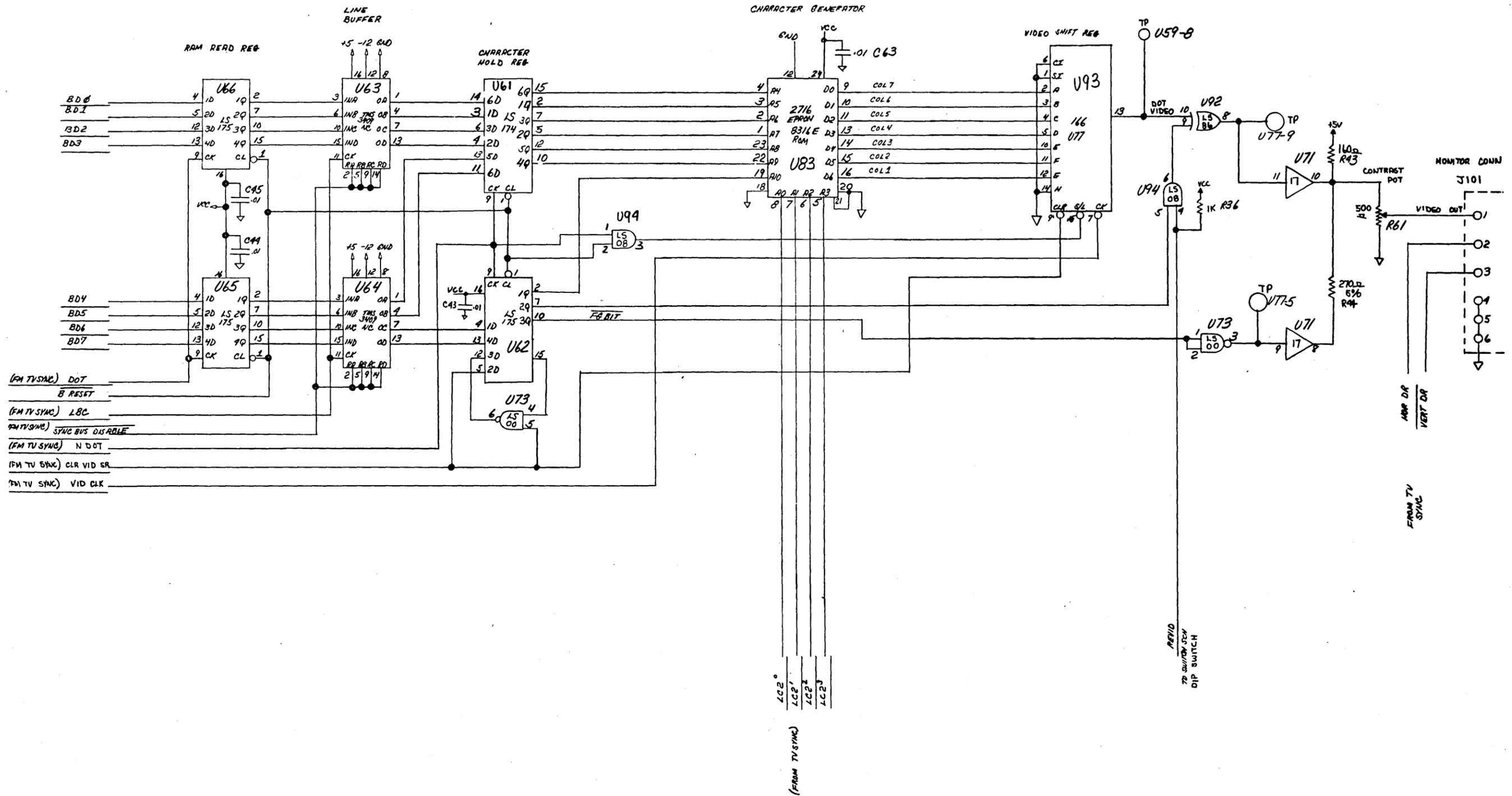
Figure B-8. Logic/Keyboard Assembly PN 4DTD155246-( ), Schematic Diagram (Sheet 5 of 9)
