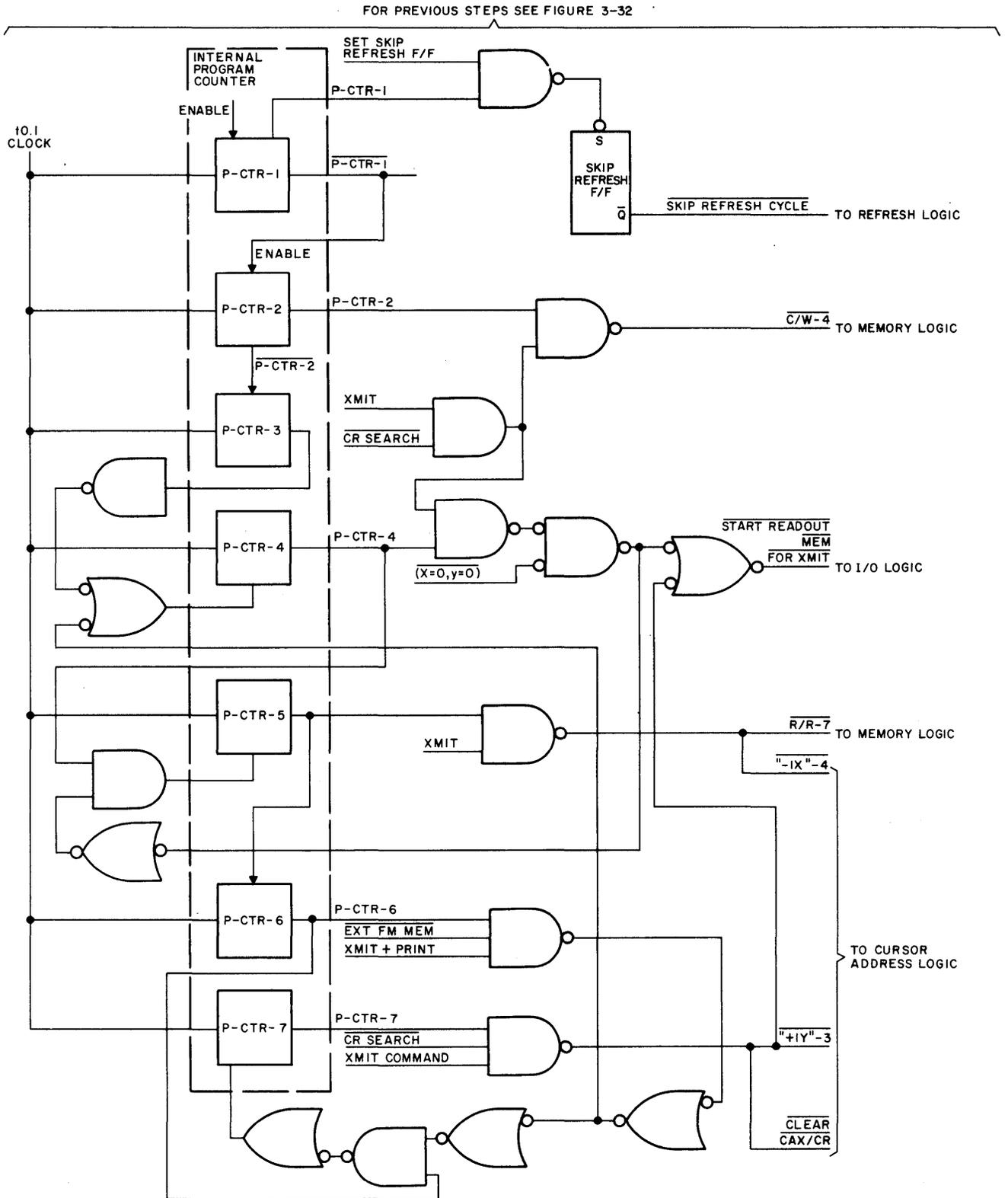
Figure 3-41. TRANSMIT Logic Flow Diagram
