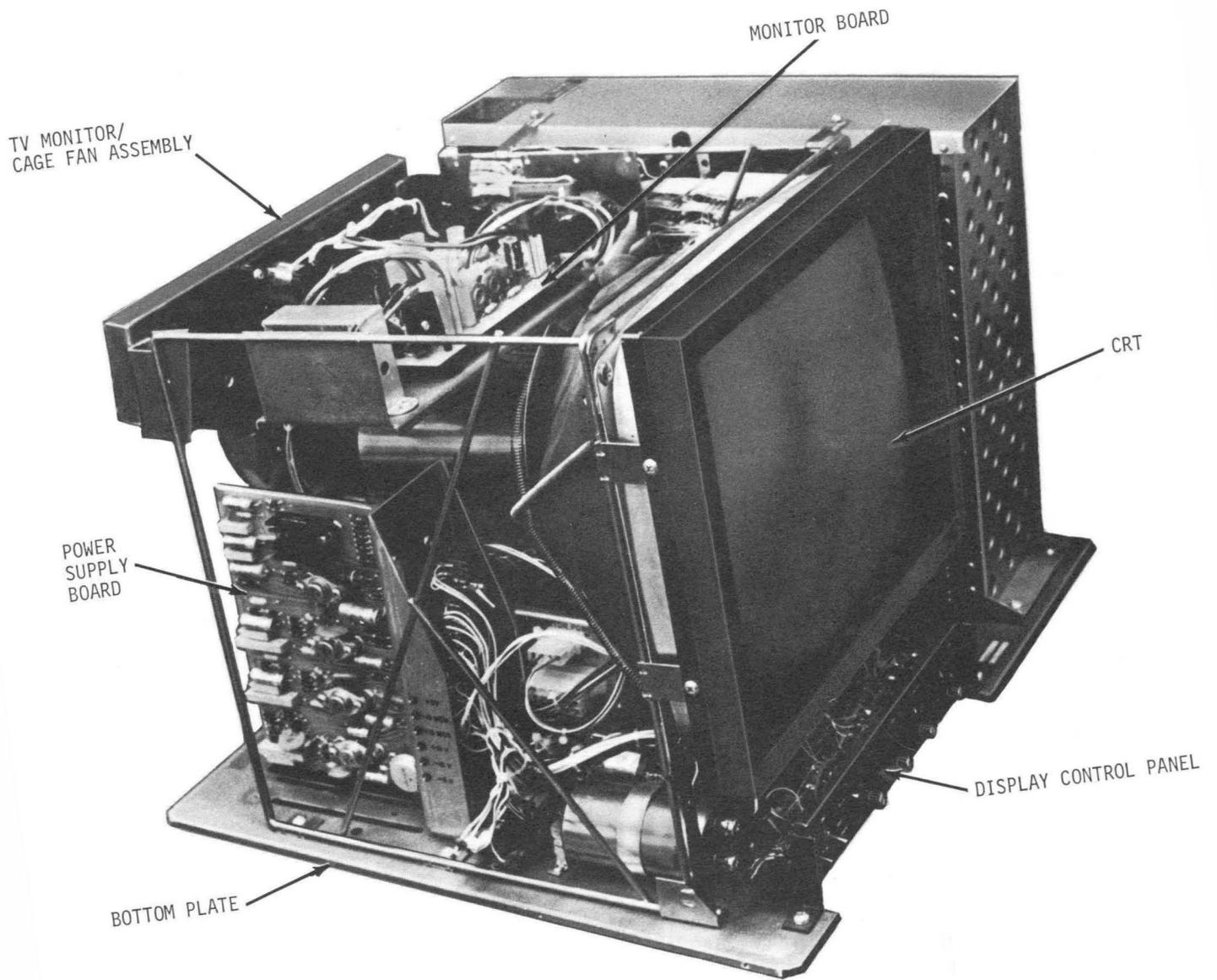
Figure 2-2. Display Unit, Front Left Side View
