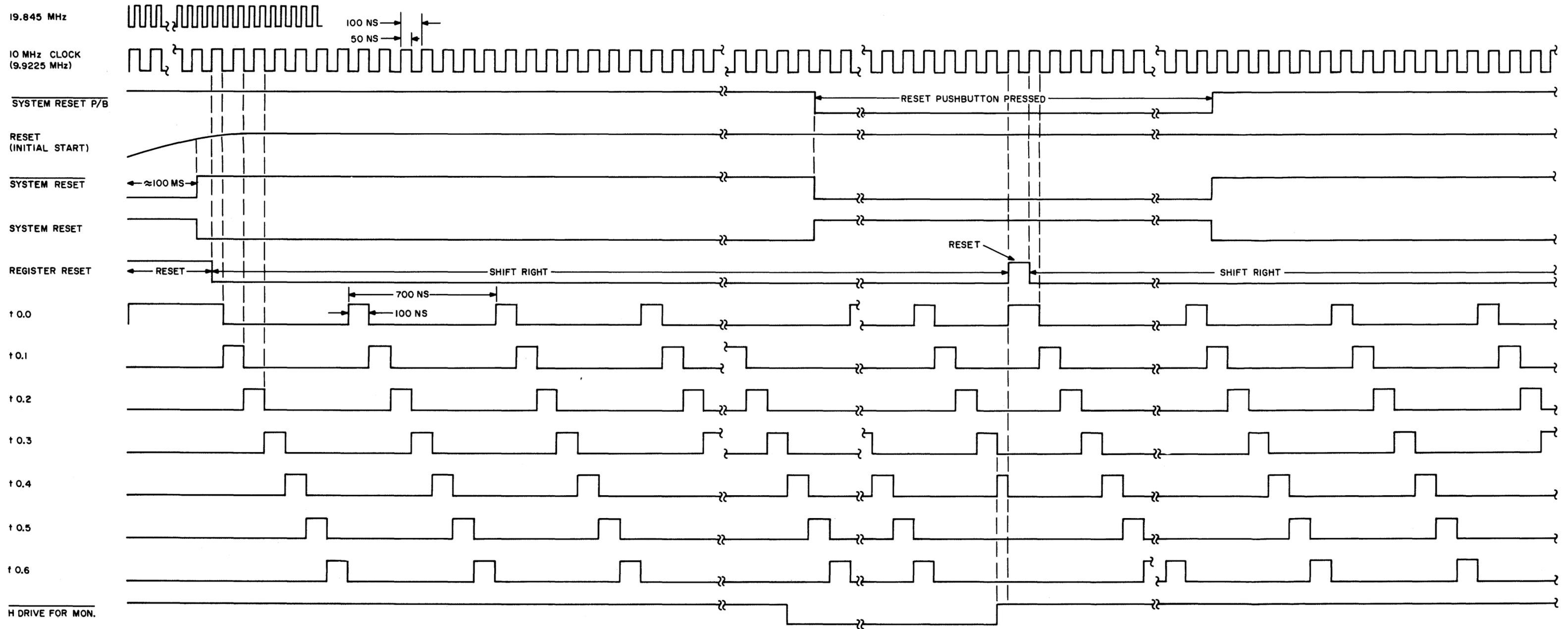
Figure 3-5. Master Clock and t-Pulse Generator, Timing Diagram
