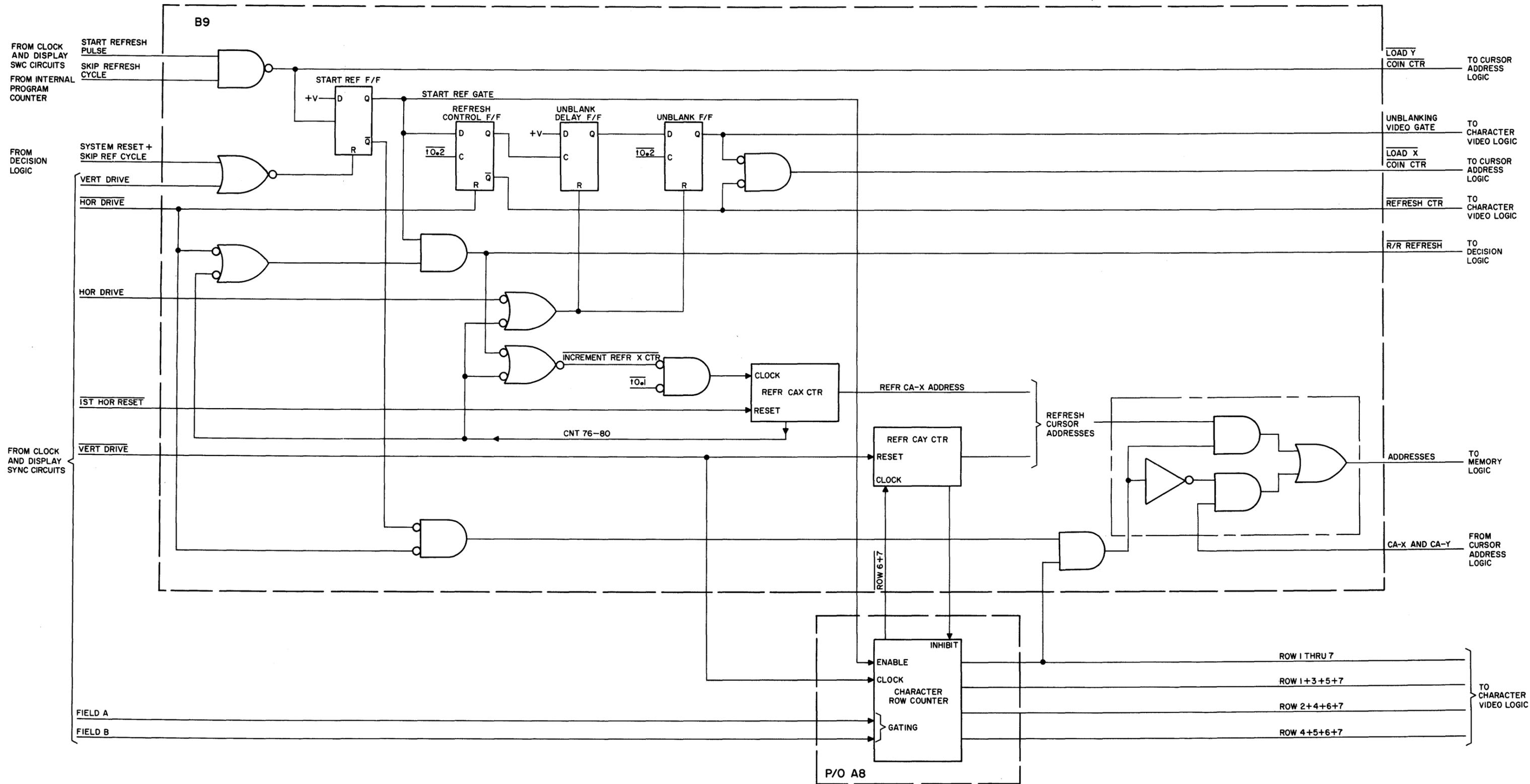
Figure 3-16. Refresh Logic Diagram
