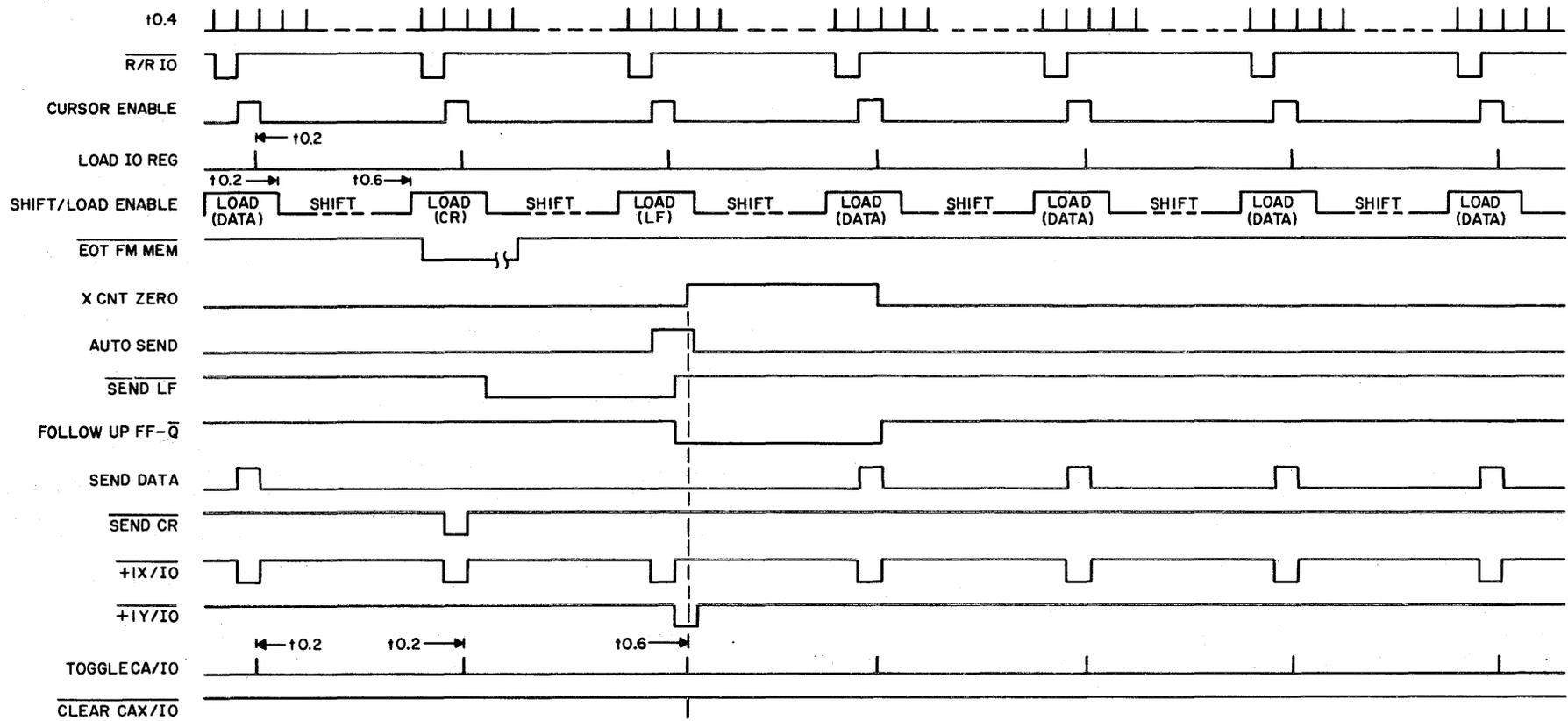
Figure 3-23. Auto-Send State Counter (EOT FM MEM), Timing Diagram
