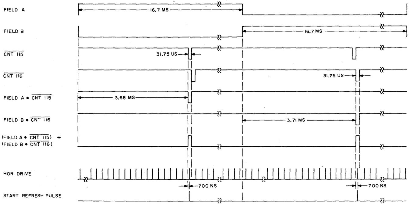
Figure 3-10. Start Refresh Pulse Logic (60-Hz Models), Timing Diagram
