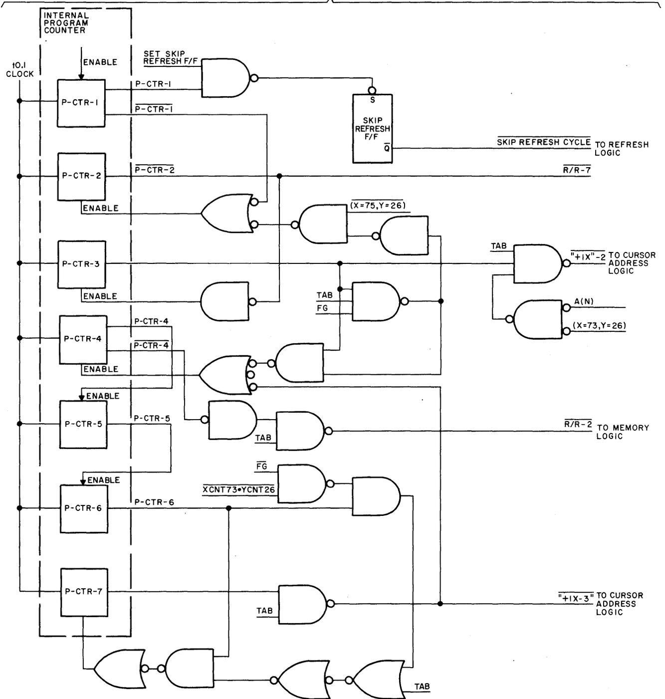
Figure 3-42. TAB Logic Flow Diagram
