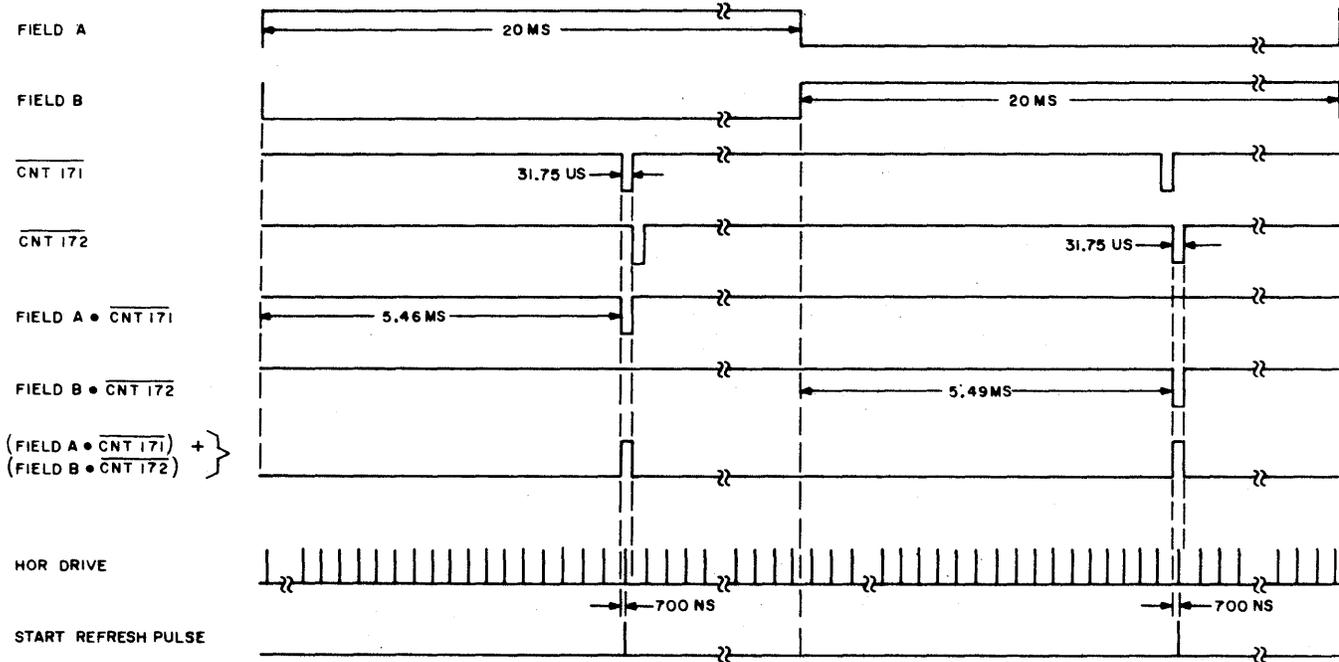
Figure 3-11. Start Refresh Pulse Logic (50-Hz Models), Timing Diagram
