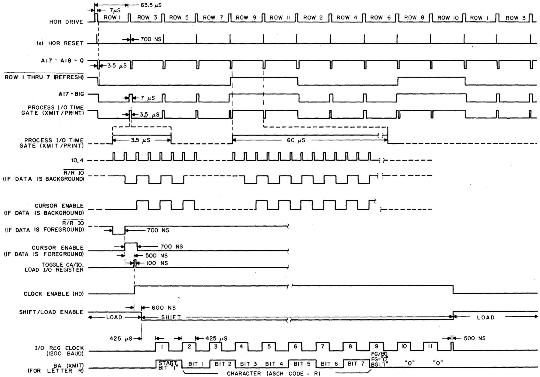
Figure 3-19. I/O Processor (Xmit Mode), Timing Diagram
