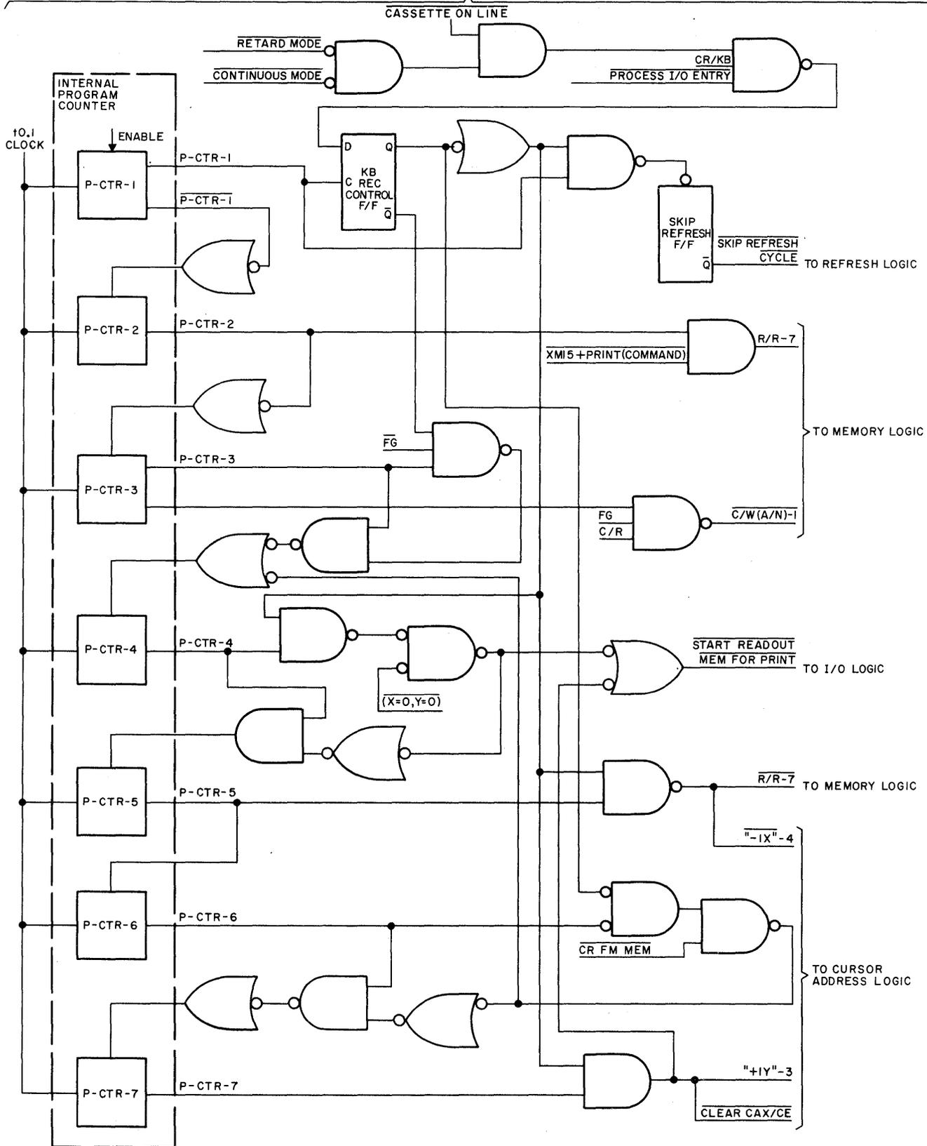
Figure 3-44. RECORD (OFF-LINE CONTINUOUS) Logic Flow Diagram
