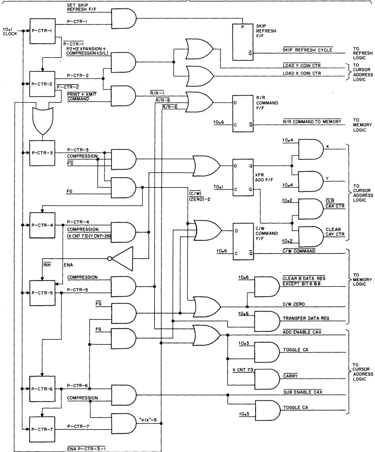
Figure 3-40. DELETE CHARACTER Logic Flow Diagram
