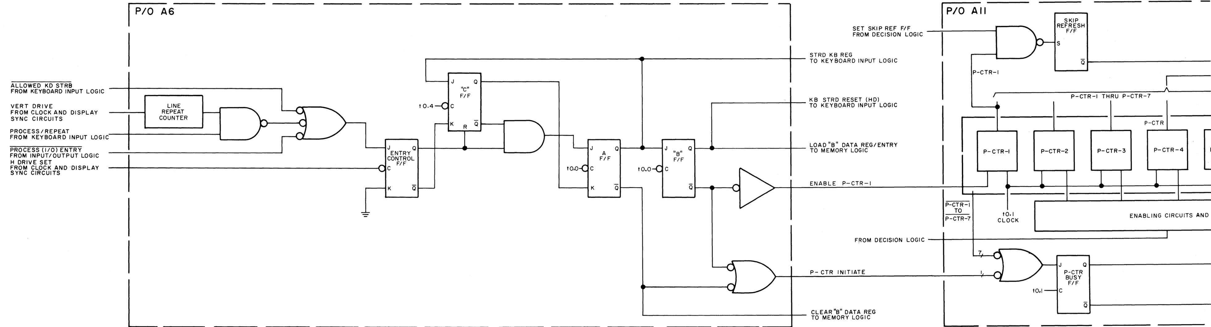
Figure 3-12. Internal Program Counter Block Diagram
