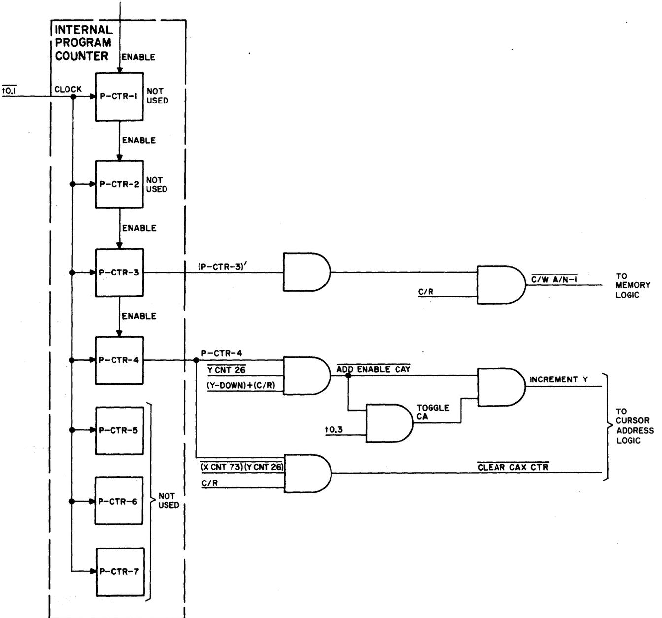
Figure 3-33. C/R Logic Flow Diagram
