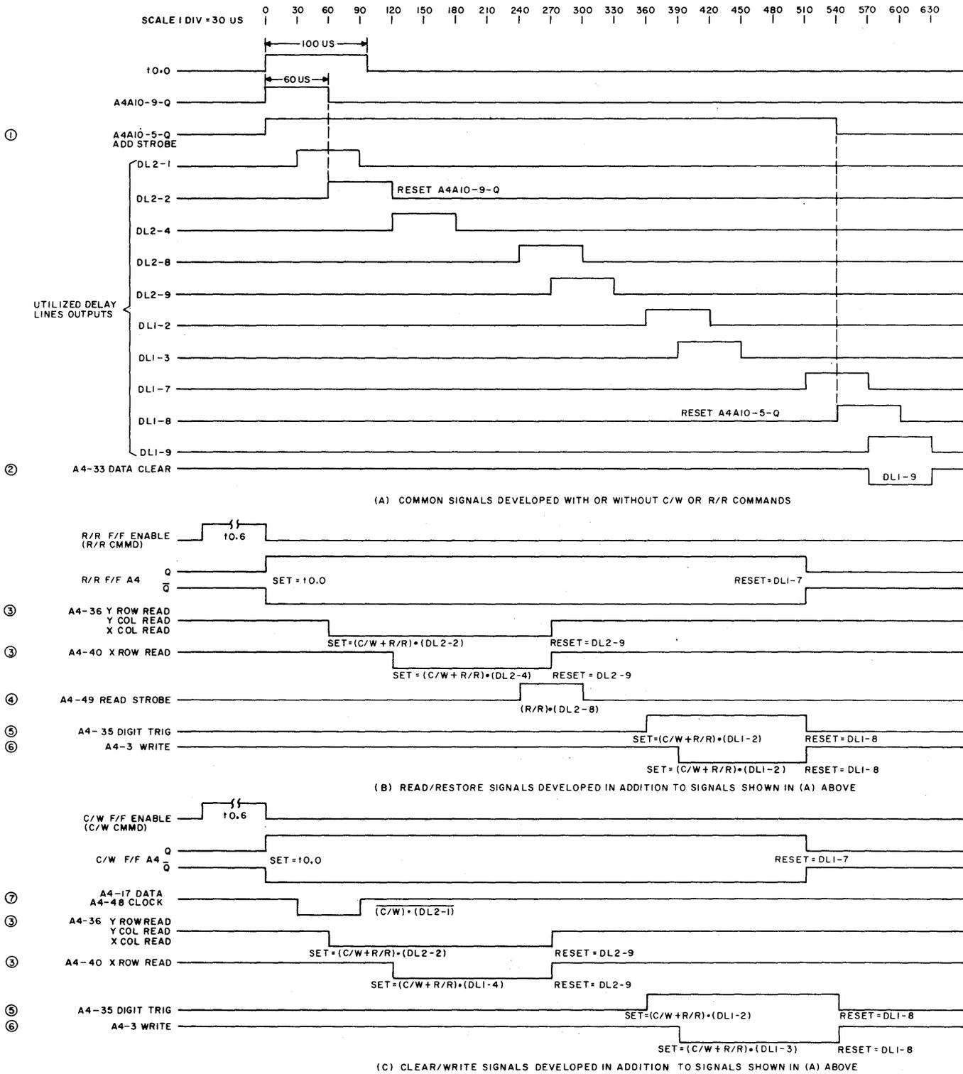
Figure 3-15. Memory Control Timing Diagram
