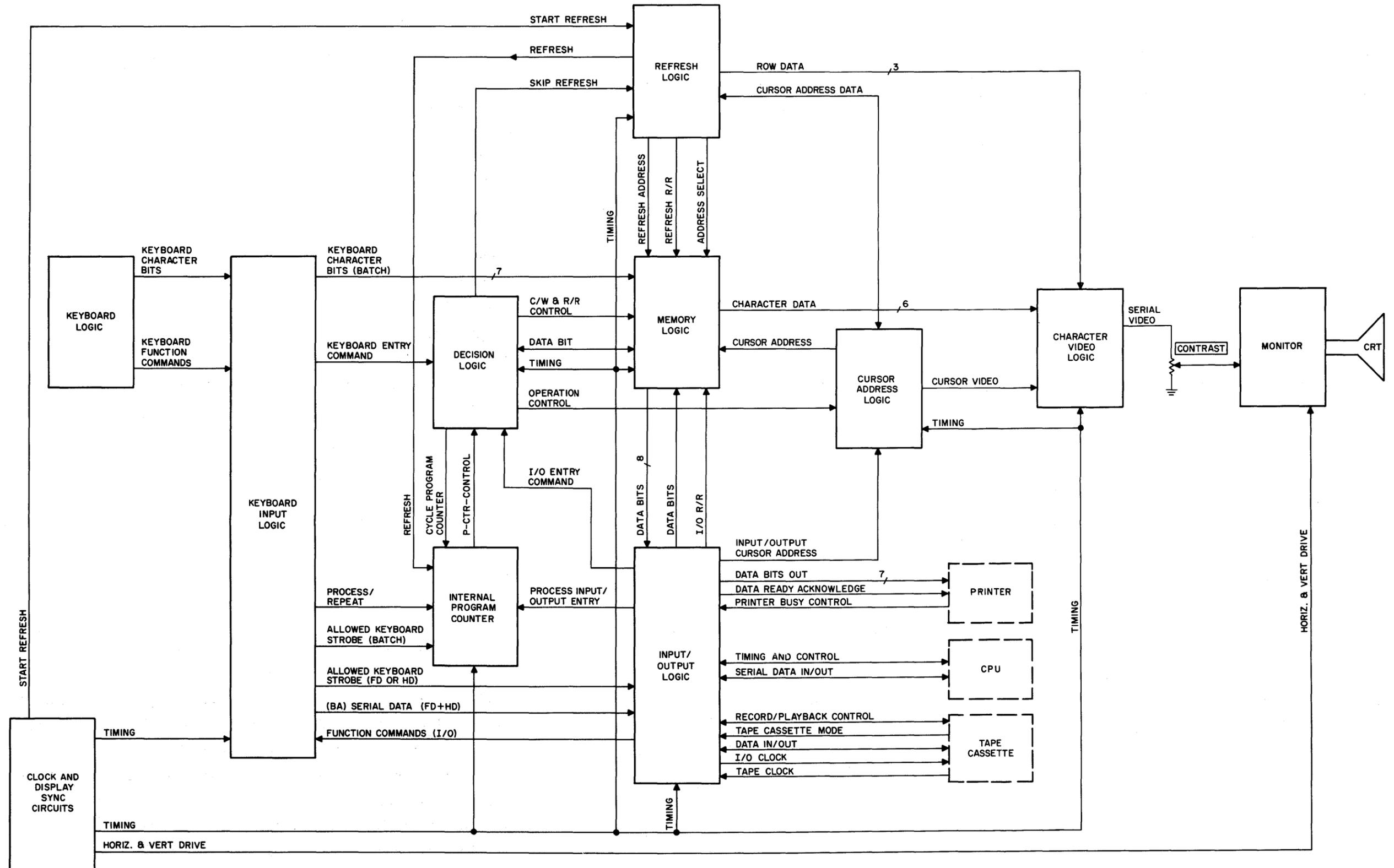
Figure 3-1. Video Display Terminal Functional Block Diagram
