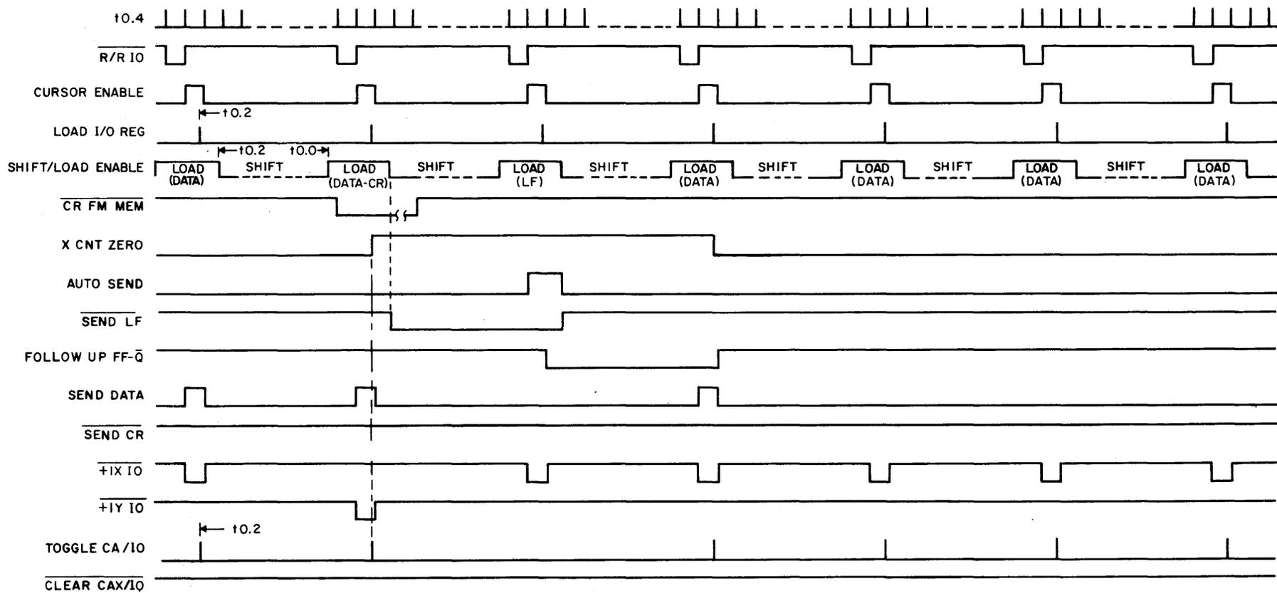
Figure 3-22. Auto-Send State Counter (CR FM MEM), Timing Diagram
