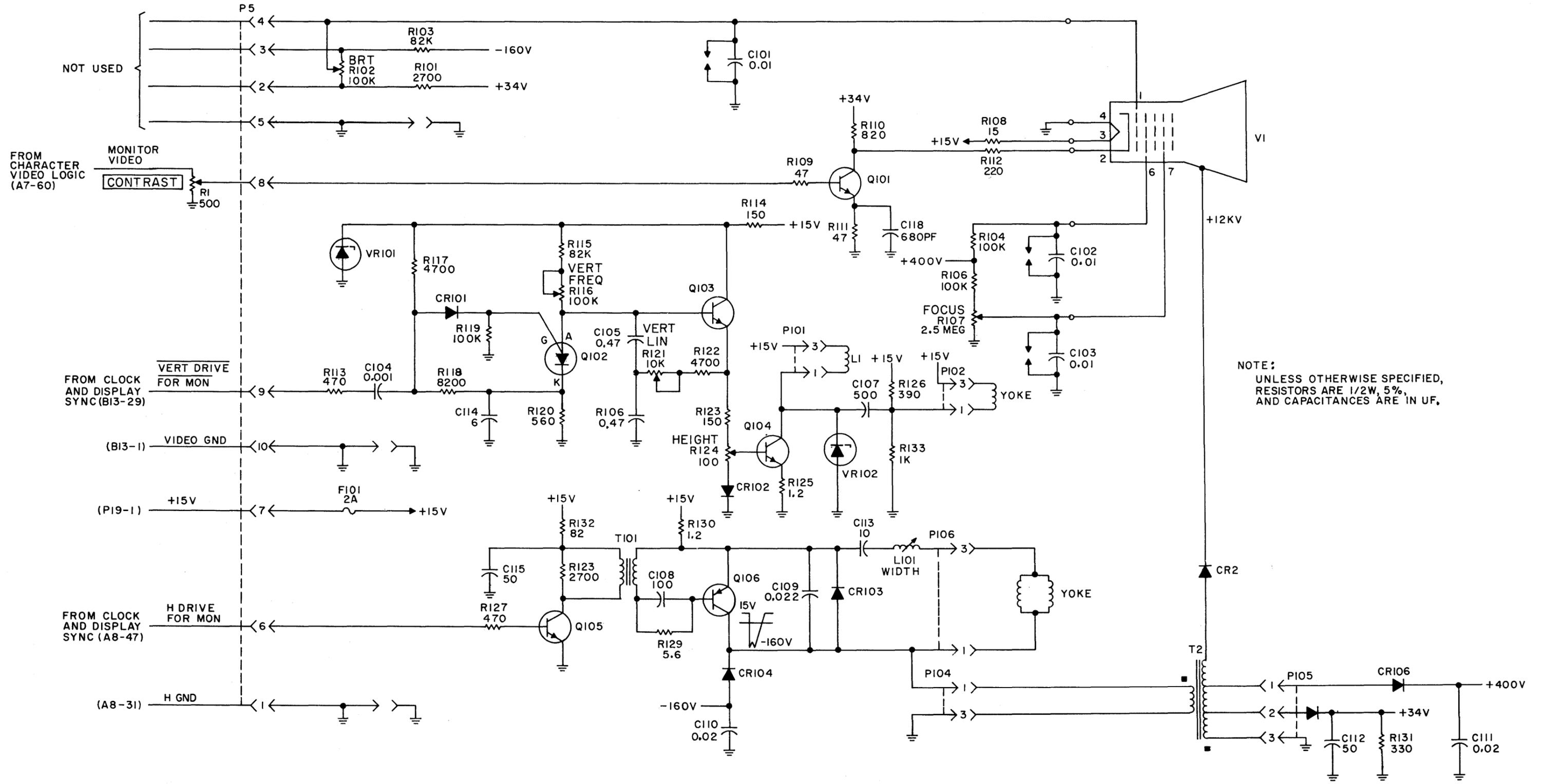
Figure 3-29. Monitor Circuits, Schematic Diagram
