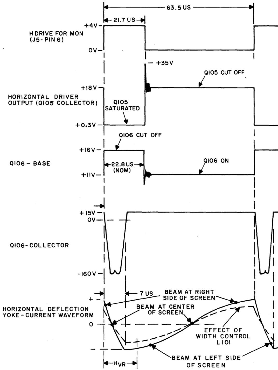
$H_{VR}$  = TOTAL RETRACE TIME = 9.5 μs (INCLUDES DEFLECTION DELAY TIME)
