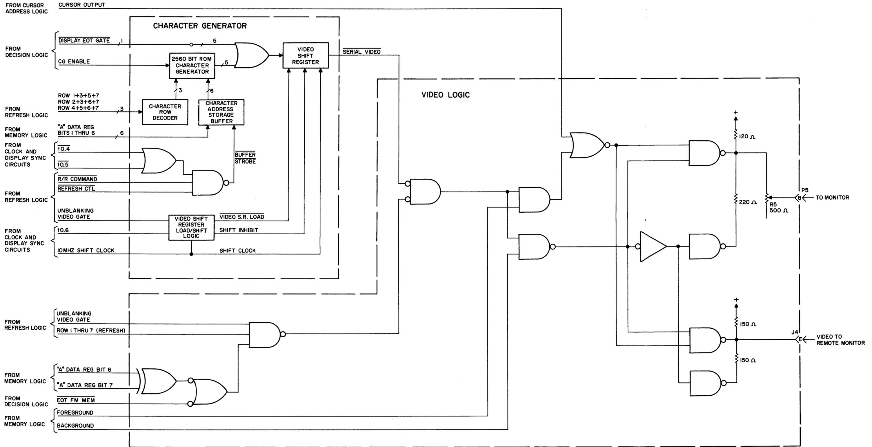
Figure 3-27. Character Video Logic Block Diagram
