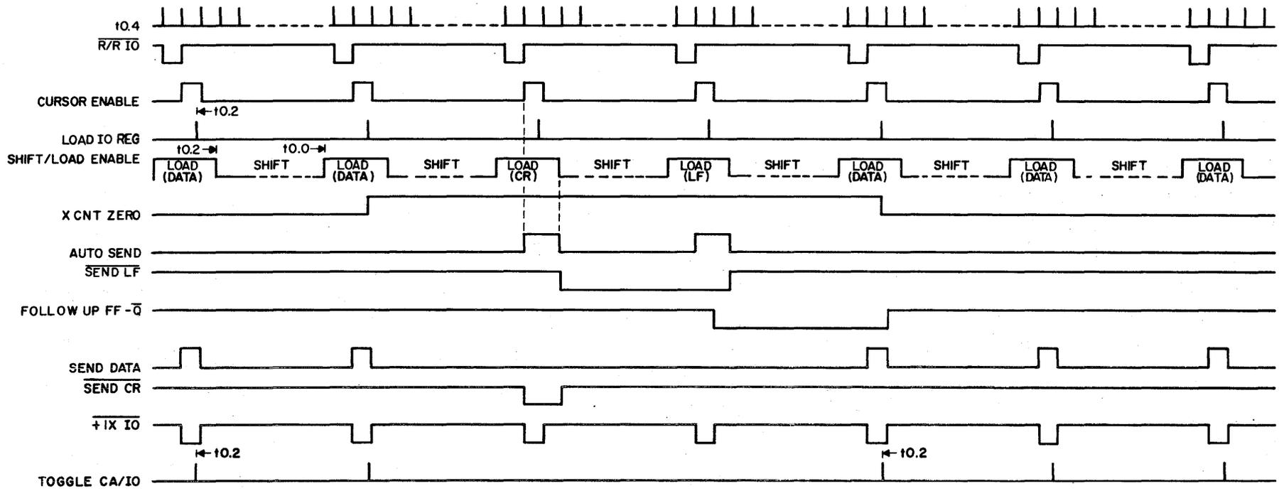
Figure 3-21. Auto-Send State Counter (Print, Record, X-CNT=0), Timing Diagram
