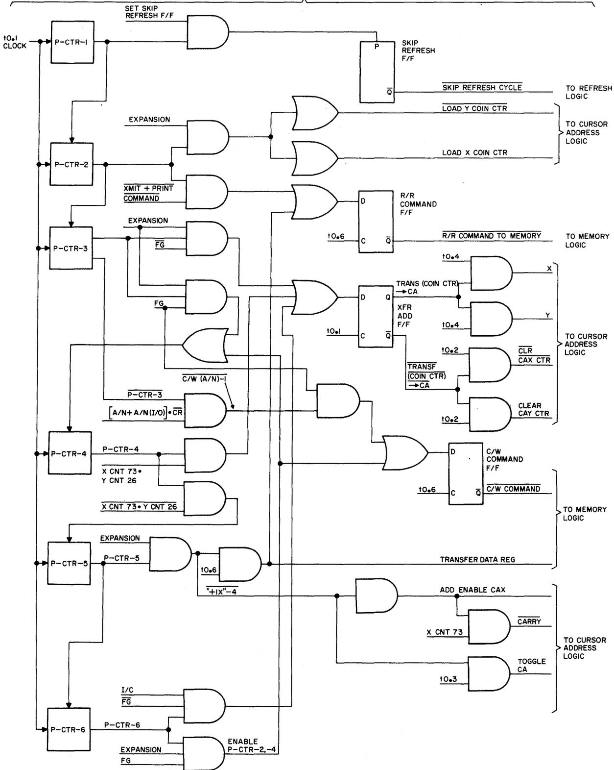
Figure 3-39. INSERT CHARACTER (I/C) Logic Flow Diagram
