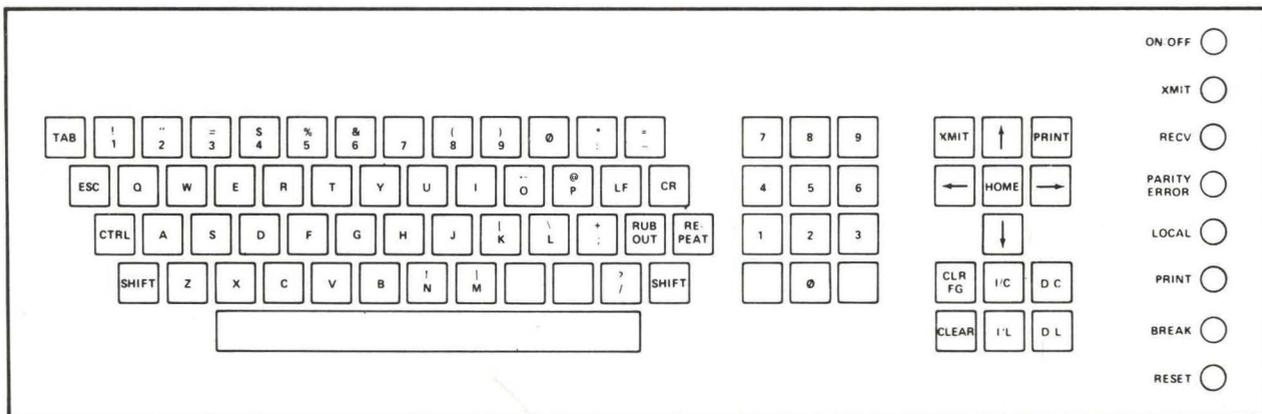
Figure 4-2. Keyboard Keys, Control Switches, and Indicators
