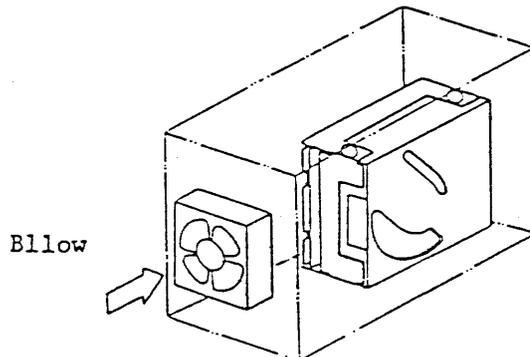
Figure 3-4 An Example of Forced Cooling
