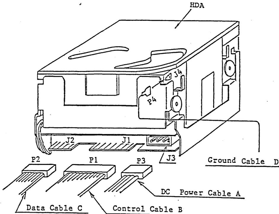
Figure 3-5 Cable Connector Locations
