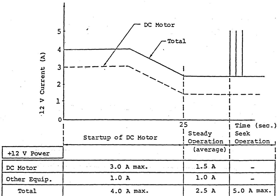
Figure 4-1 +12 V DC Power Requirements
