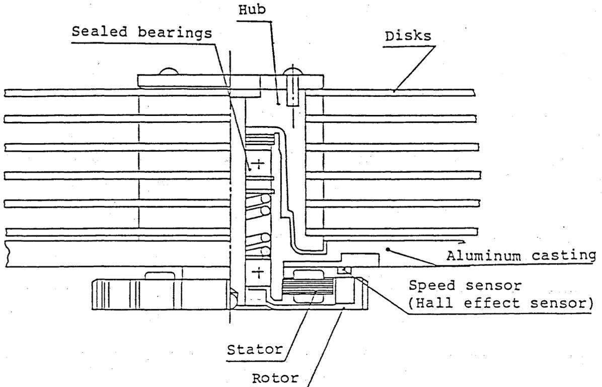
Figure 2-2 Spindle Motor
