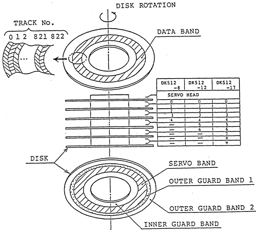
Figure 2-5 Head and Cylinder Address
