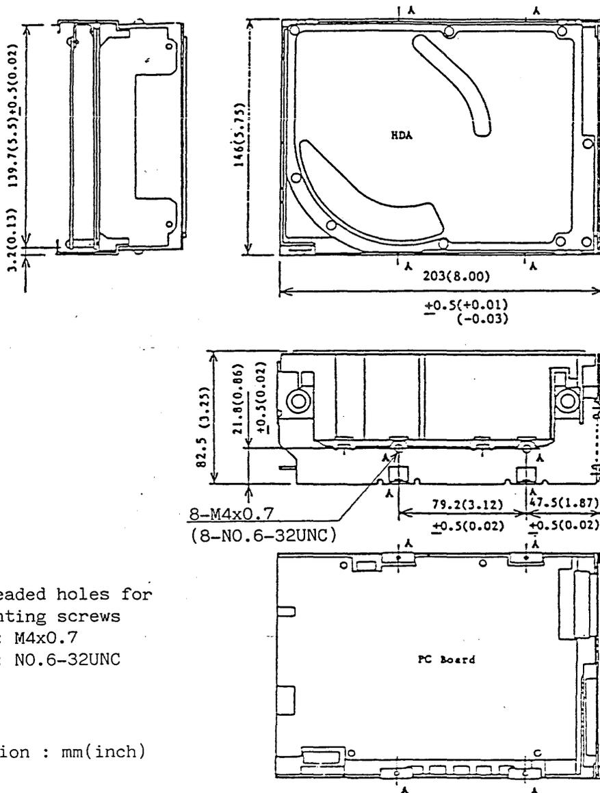
Figure 3-3 DK512 Mounting Dimensions: Side and Top Views
