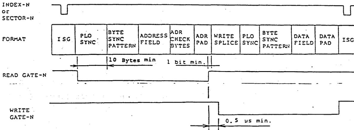
Figure 5-6 WRITE GATE Timing When Writing Data
