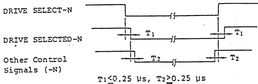
Figure 5-13 DRIVE SELECTED Timing with DRIVE SELECT and Control Signals
