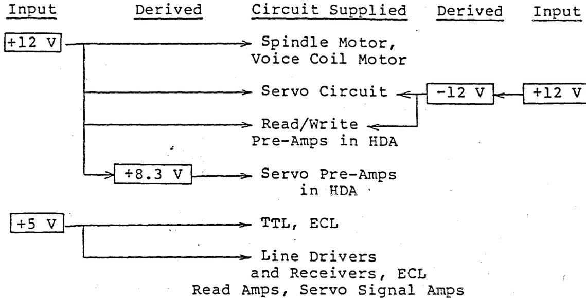
Figure 2-6 Voltage Utilization
