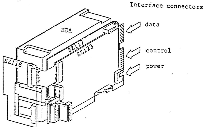
Figure 3-1 DK512 PC Boards and Interface Connectors
