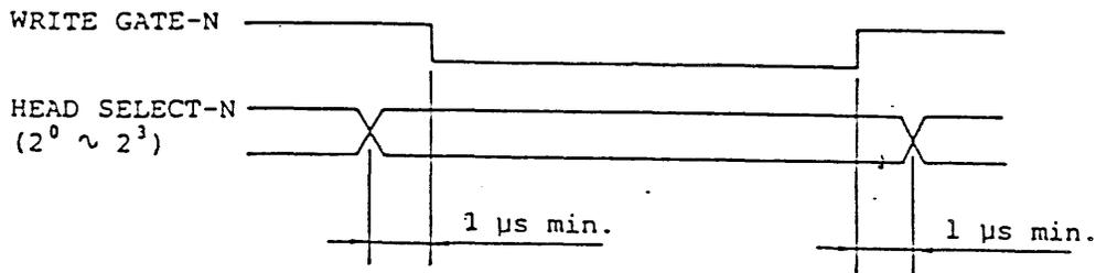
Figure 5-8 WRITE GATE Timing with HEAD SELECT
