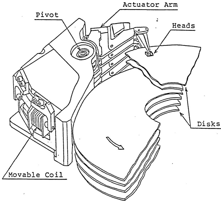
Figure 2-3 Actuator Arm Assembly
