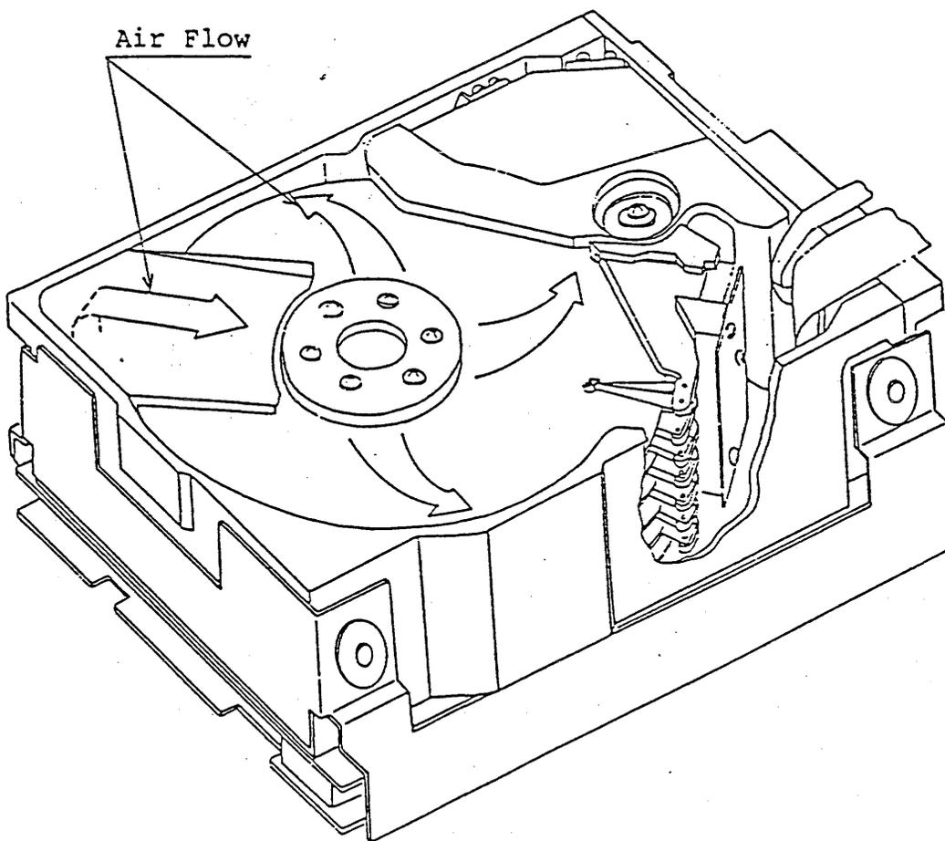
Figure 2-4 Air Circulation Inside Head and Disk Assembly
