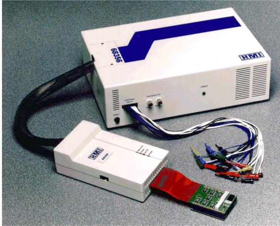
HMI 200 Series emulators are high performance development systems which combine the control of an in-circuit emulator with the power of a logic analyzer to provide a complete debugging environment for hardware and software.
