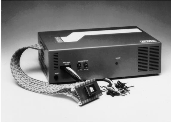
The HMI-200-8096 emulator is a high performance development system which combines the control of an in-circuit emulator with the power of a logic analyzer to provide a complete debugging environment for hardware and software.
