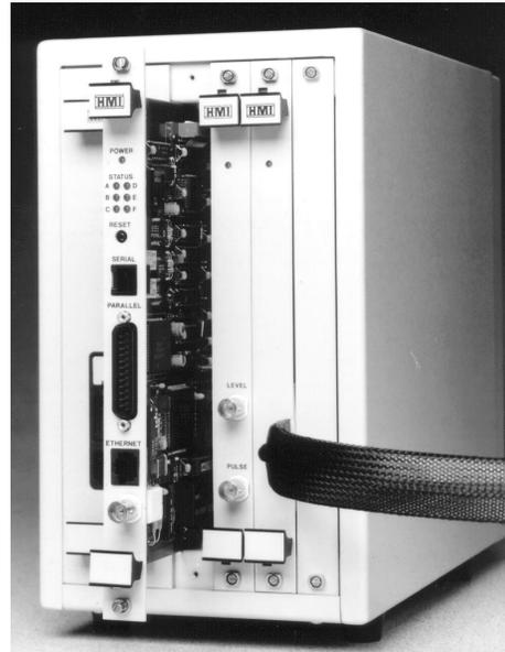
Backplane based design results in high reliability and allows for easy expandability and in-field service. 3' emulation cable for those tough to reach target systems.
