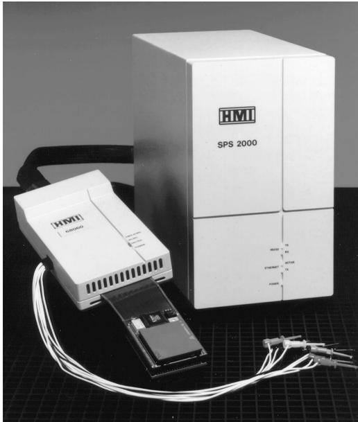
The SPS 2000 68060 emulator is a high performance development system which combines the control of an in-circuit emulator with the power of a logic analyzer to provide a complete debugging environment for hardware and software.
