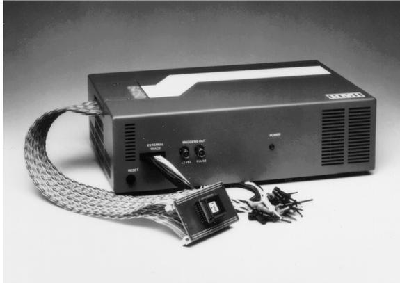
The HMI-200-Z80 emulator is a high performance development system which combines the control of an in-circuit emulator with the power of a logic analyzer to provide a complete debugging environment for hardware and software.
