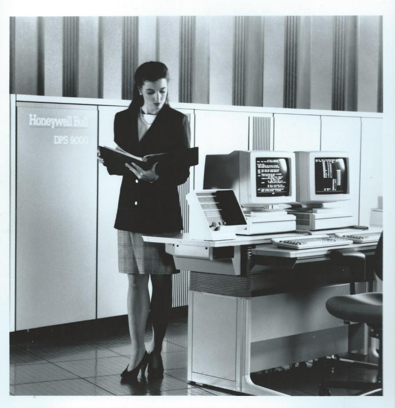
HONEYWELL BULL'S DPS 9000, THE MOST POWERFUL general purpose mainframe computer in the world. Targeted for high-volume, information-intensive usage such as transaction processing and data management, the DPS 9000 is rated at more than 1,000 transactions per second in the industry standard debit/credit benchmark.
