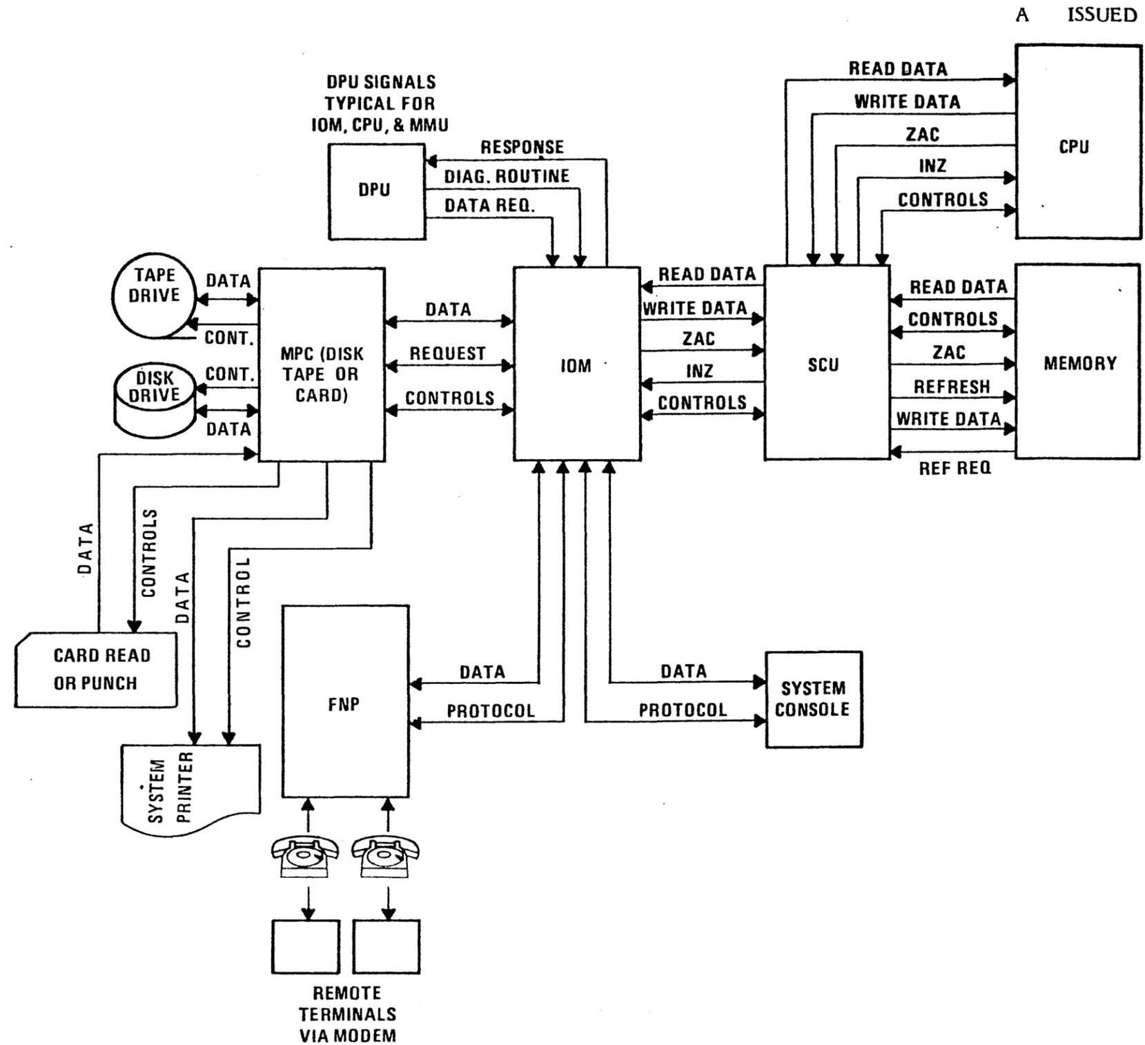
FIGURE 1-3. SIGNAL FLOW
