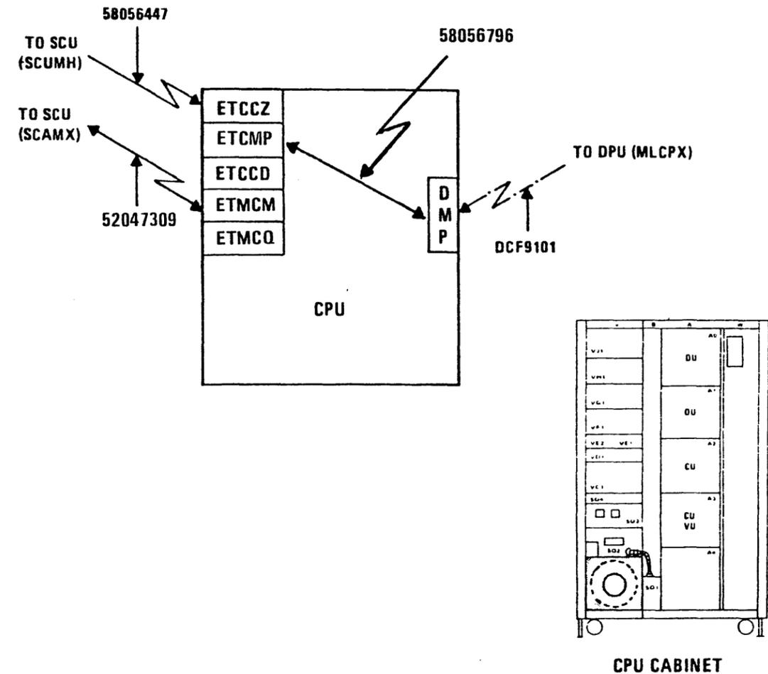
FIGURE 3-5 CPU CABINET INTERFACES
