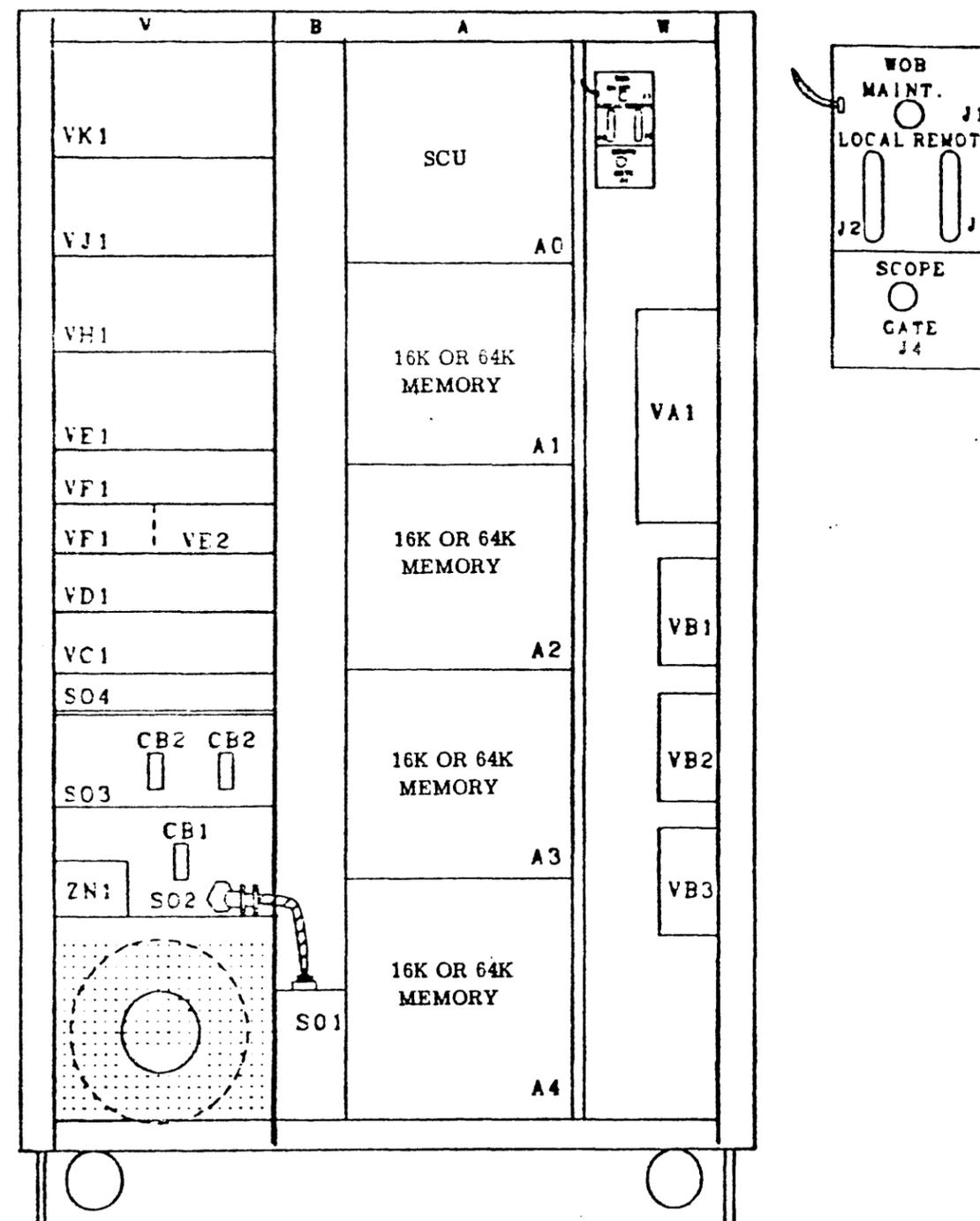
FIGURE 2-4 MMU CABINET FRONT VIEW WITH DOORS REMOVED
