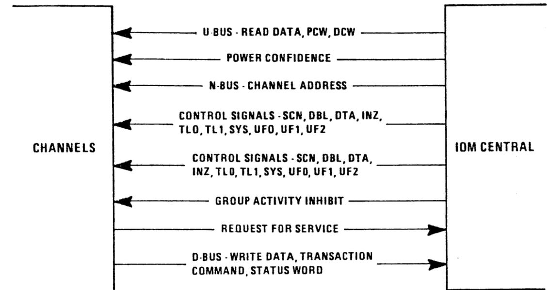
FIGURE 3-4 I/O BUS INTERFACE
