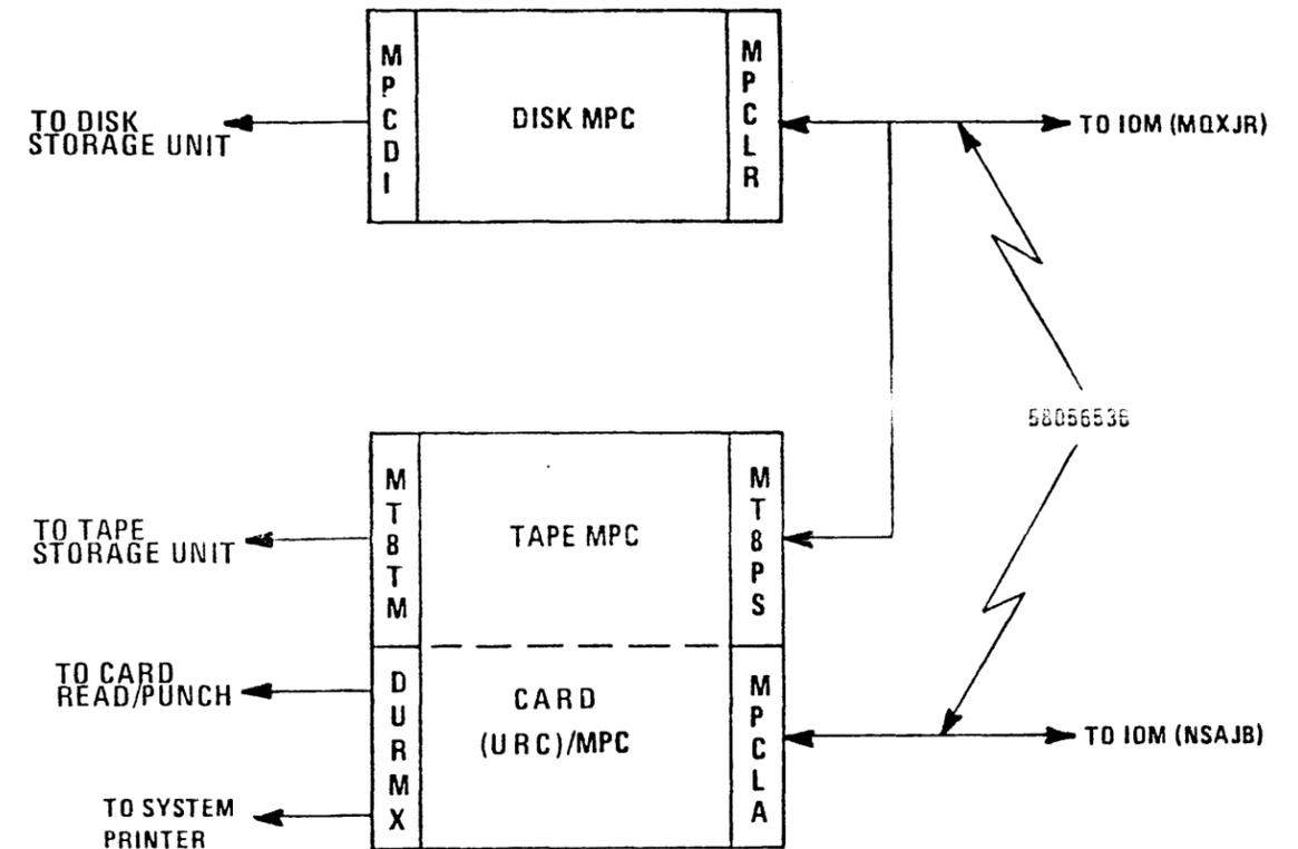
FIGURE 3-6 MPC CABINET INTERFACES
