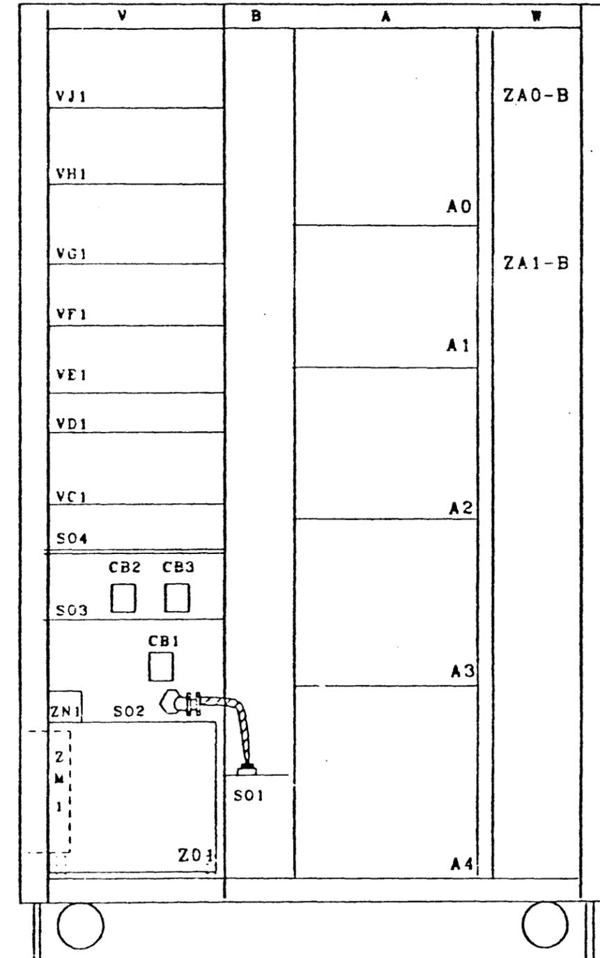
FIGURE 2-6 BASIC MPC (DISC/TAPE) CABINET FRONT DOORS REMOVED
