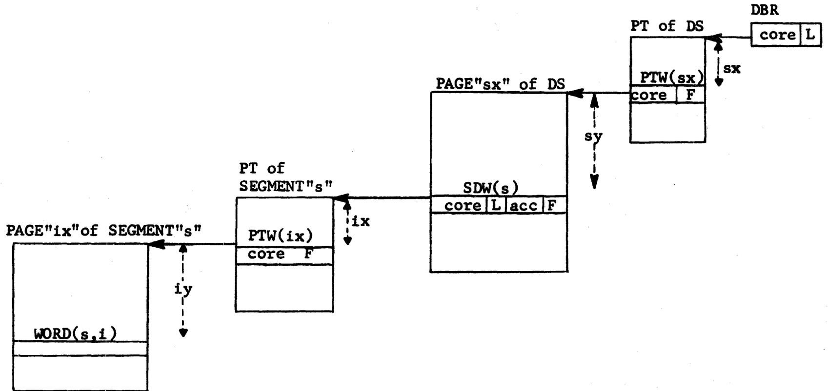
Figure 3. Hardware Segmentation and Paging in the 645
