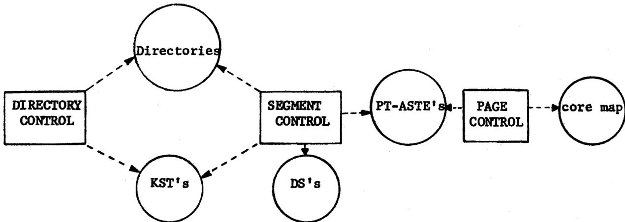
Figure 6. Supervisor Functional Modules and Data Bases
