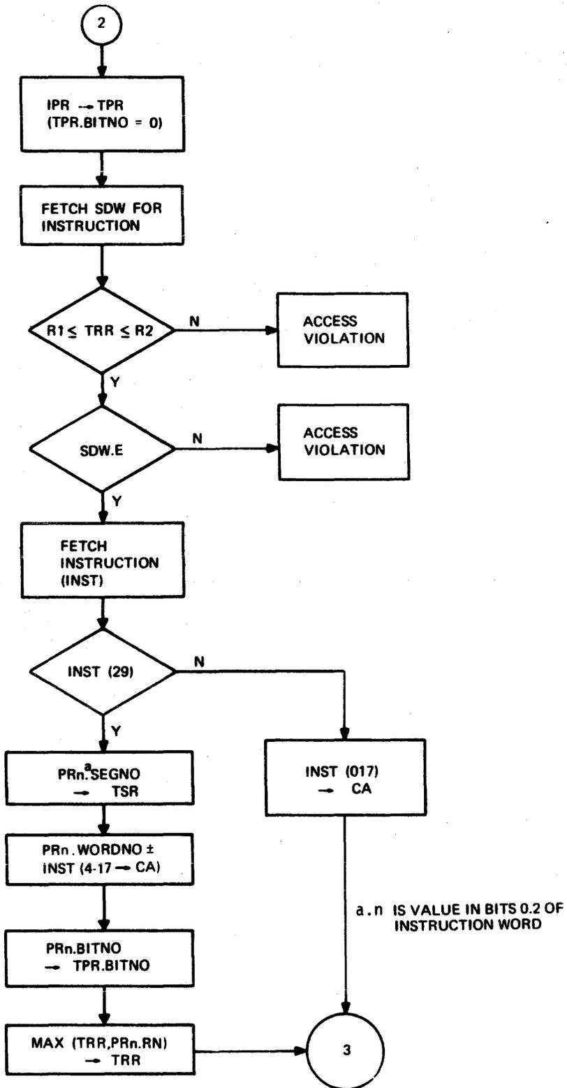
Figure 2. Instruction Fetch and Initial Address Calculation
