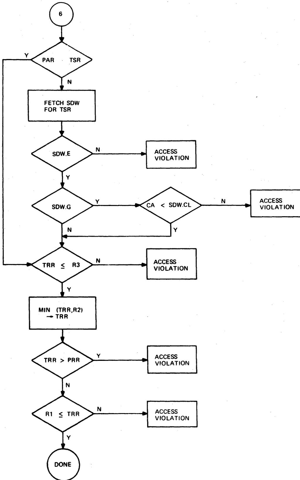
Figure 6. Access Checks for CALL Instruction
