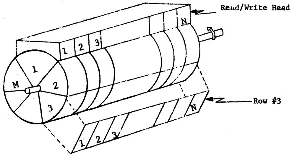
Figure 1. Drum Configuration
