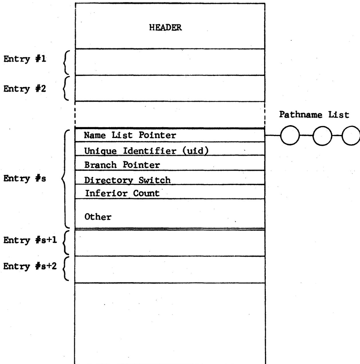
Figure 1. Structure of the Known Segment Table (KST)
