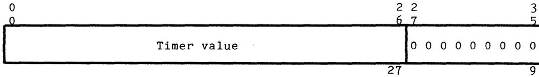
Figure 3-9. Timer Register (TR) Format
