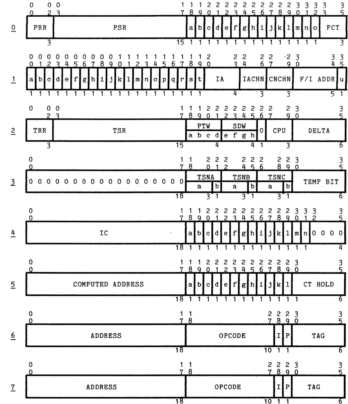
Figure 3-32. Control Unit Data Format
