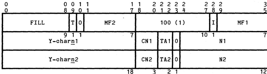
Figure 4-17. Move Alphanumeric Left to Right (mlr) EIS Multiword Instruction Format
