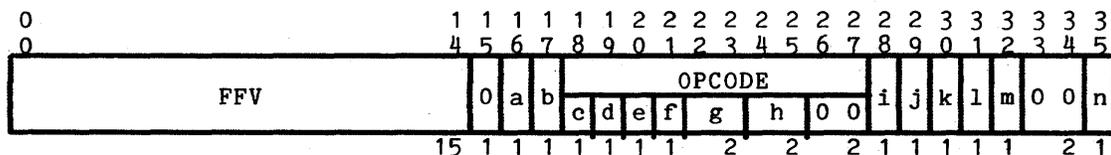
Figure 3-20. Mode Register (MR) Format - DPS and L68
