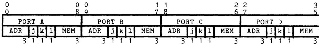
Figure 3-31. Configuration Switch Data Formats - DPS 8M
