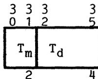
Figure 6-1. Address Modifier (TAG) Field Format
