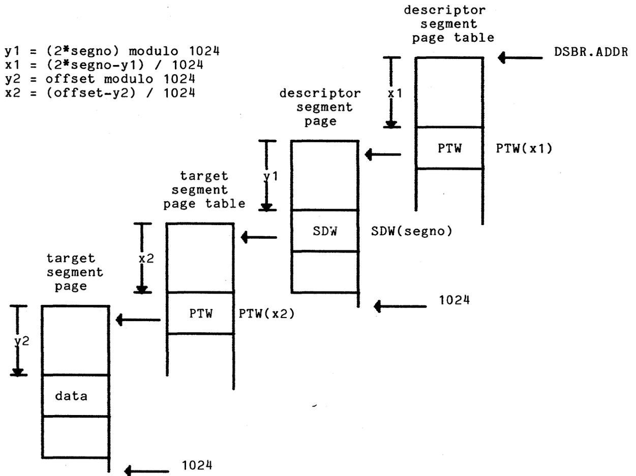
Figure 5-3. Main Memory Address Generation for Paged Segments
