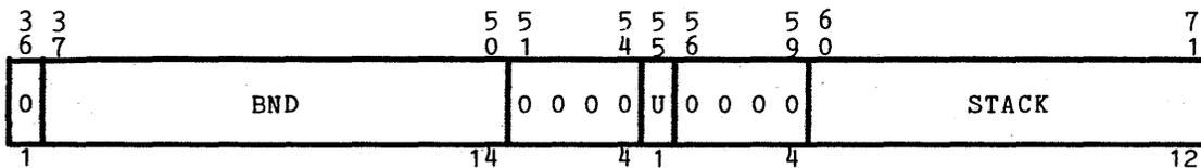
Figure 3-15. Descriptor Segment Base Register (DSBR) Format
