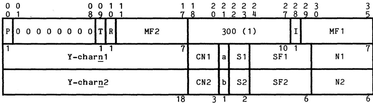
Figure 4-21. Move Numeric (mvn) EIS Multiword Instruction Format
