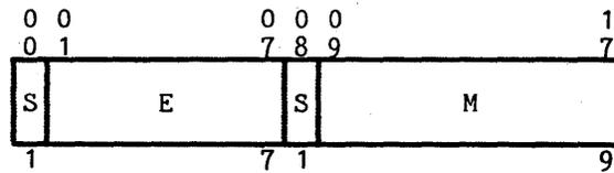
Figure 2-7. Eighteen-bit Half Word Floating-Point Binary Operand Format
