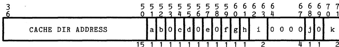
Figure 3-23. Cache Mode Register (CMR) Format - DPS 8M
