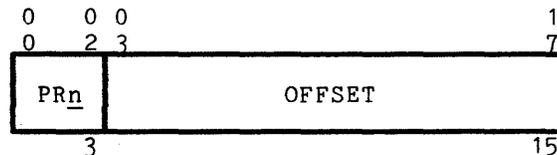
Figure 6-7. Format of Instruction Word ADDRESS When Bit 29 = 1
