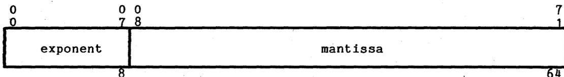
Figure 3-5. Exponent-Accumulator-Quotient Register (EAQ) Format
