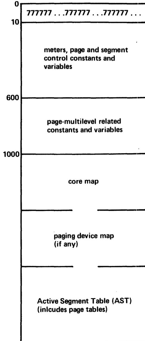
Figure 5-1. Layout of System Segment Table (SST)
