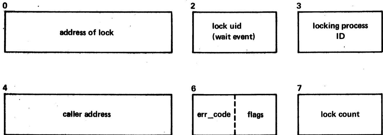
Figure 5-11. Format of Lock Entry in `lock_seg`
