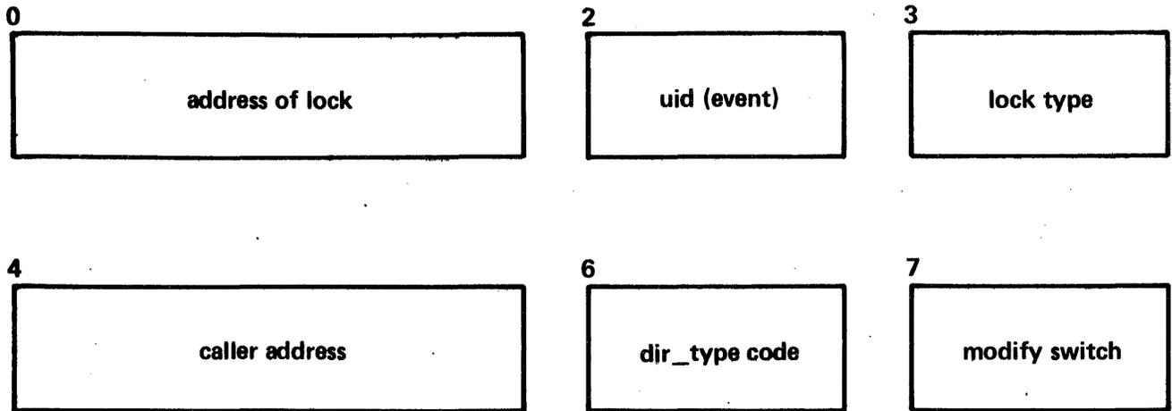
Figure 5-12. Format of Lock Array Entry
