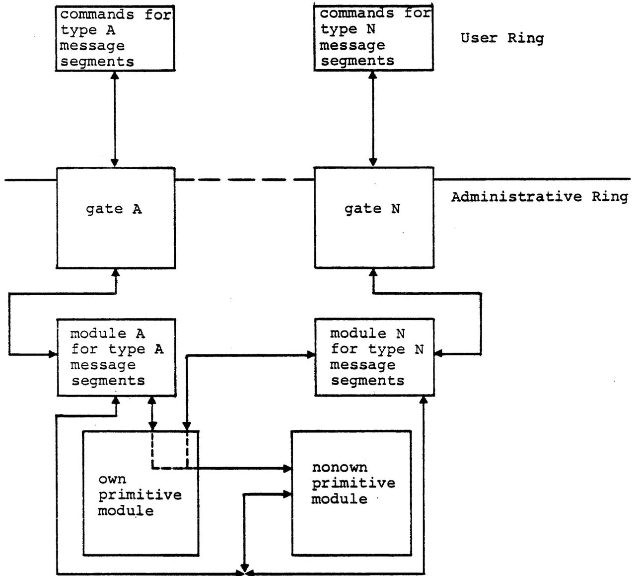
Figure 2-1. Sample Message Segment Facility Configuration
