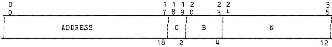
Figure 1-14. EIS Bit String Data Descriptor Format
