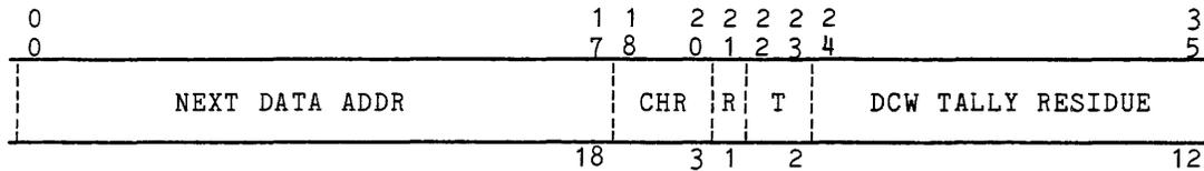
Figure 3-10. IOM Channel Status Data Format
