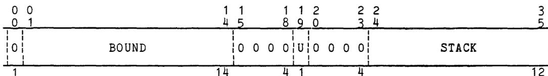
Figure 1-6. Descriptor Base Register (DBR) Format
