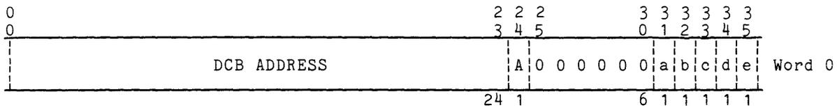
Figure B-4. Bulk Store Current Status Block (CSB) Format
