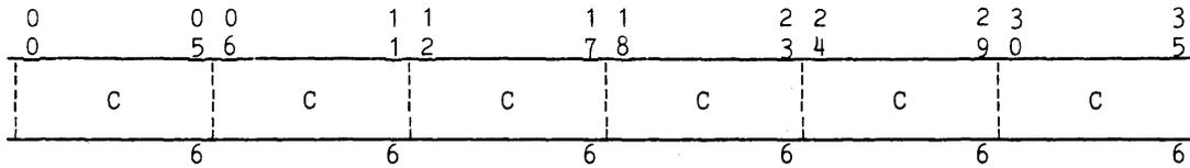
Figure 1-19. EIS Alphanumeric Data Format, 6-bit Mode
