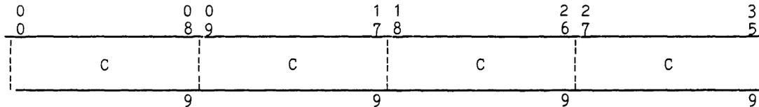
Figure 1-20. EIS Alphanumeric Data Format, 9-bit Mode
