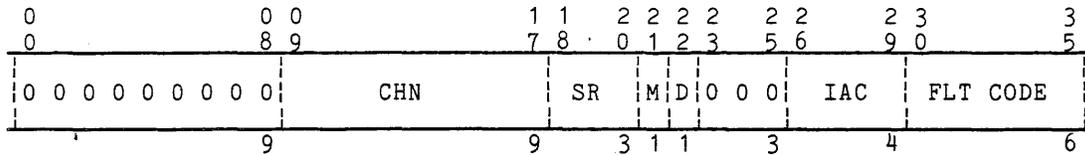
Figure 3-9. IOM System Fault Status Word Format
