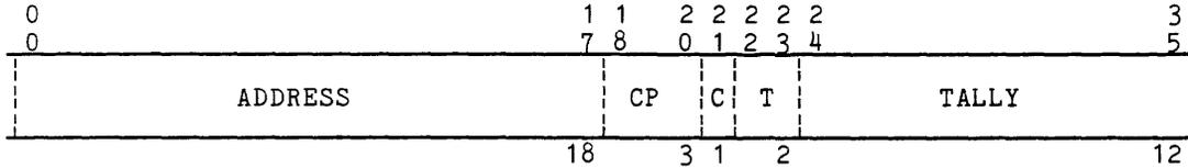
Figure 3-5. IOM Data Transmission DCW Format
