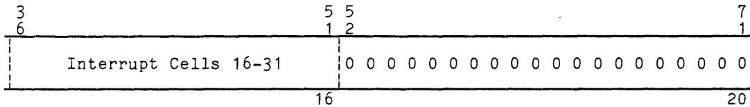
Figure 2-3. Interrupt Cells (rscr/sscr 00003X) Data Format
