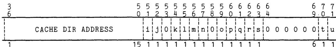
Figure 1-48. Cache Mode Register Format
