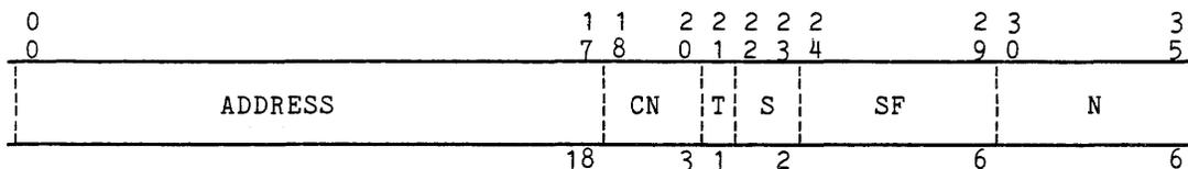
Figure 1-16. EIS Numeric Data Descriptor Format
