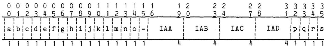
Figure 1-34. Processor Fault Register Format
