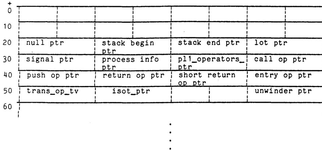
Figure 7-5. Stack Header Layout
