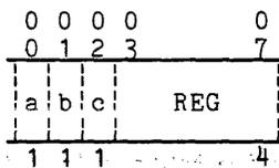
Figure 1-12. EIS Data Descriptor Modification Field (MF) Format
