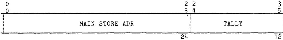
Figure 4-5. Bulk Store Data Control Block (DCB) Format, Word 2
