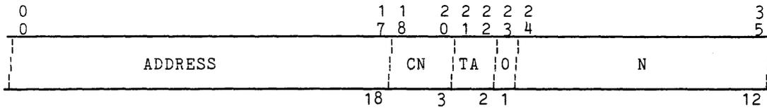
Figure 1-15. EIS Alphanumeric Data Descriptor Format
