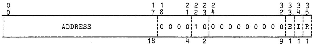
Figure 3-7. IOM Transfer DCW Format
