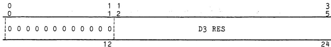
Figure 1-30. DU Pointers and Lengths Format, Word 7
