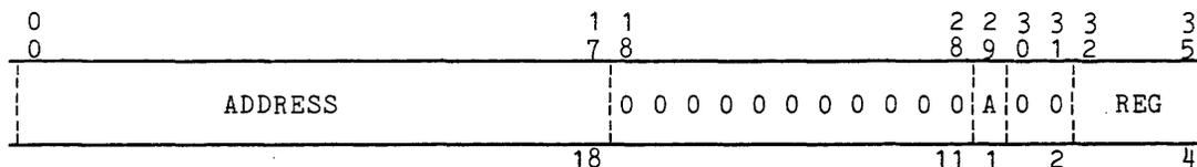
Figure 1-13. EIS Indirect Data Descriptor Pointer Format
