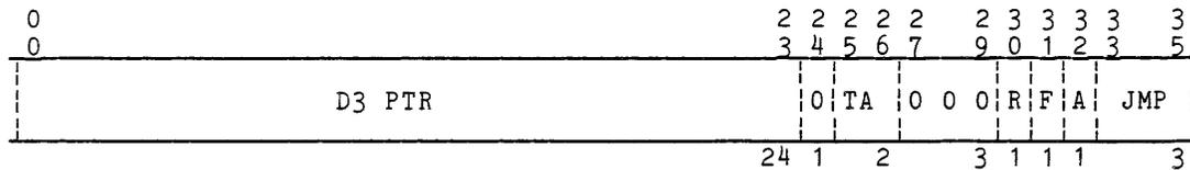
Figure 1-29. DU Pointers and Lengths Format, Word 6
