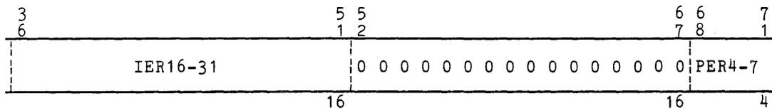
Figure 2-2. Interrupt Mask Register (rscr/sscr 000N2X) Data Format
