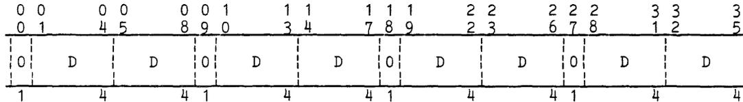
Figure 1-21. EIS Numeric Data Format, 4-Bit Mode
