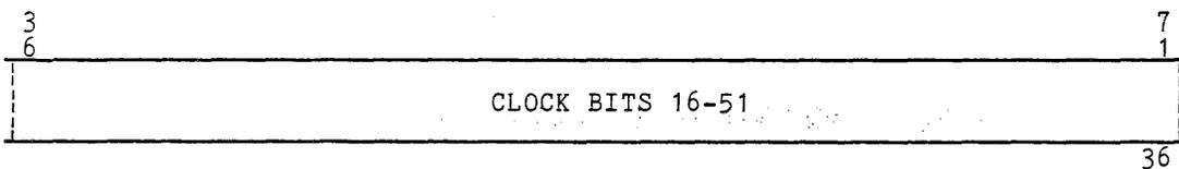
Figure 2-4. System Clock (rscr/sscr/rccl 00004X) Data Format
