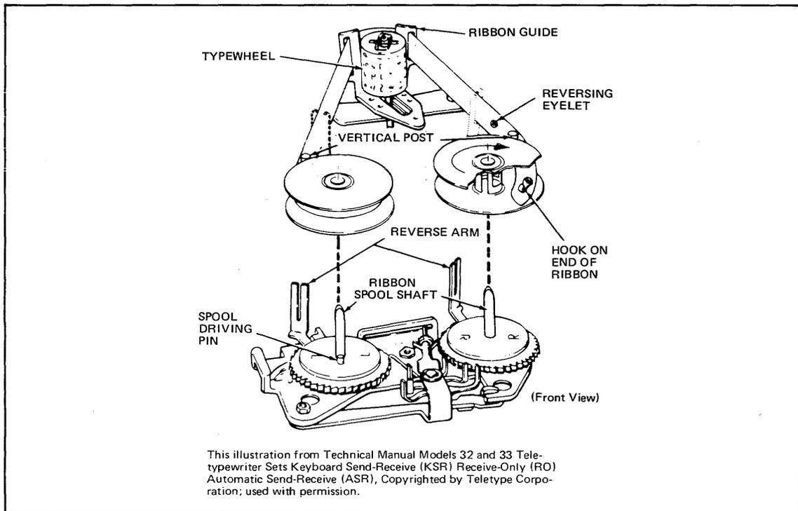
**Figure 2-6. Ribbon Installation**
