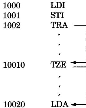
Any attempt to trap on instruction counter=10010 will fail because all the above instructions except LDA are non-interruptible. Conversely, if the LDI was loading the indicators with the "compared" value, the CP would stop only at the end of the LDA at 10020 and the instruction counter would indicate 10021 because it would be the first interruptible instruction where the condition is met.
