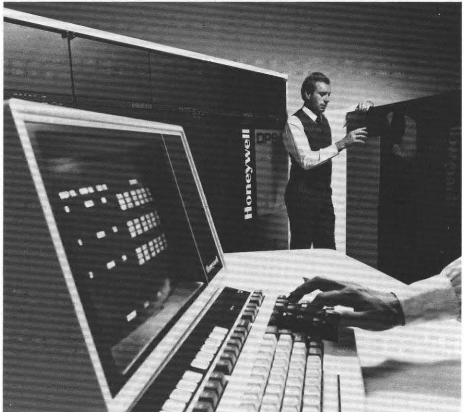
As satellite processors, Honeywell's DPS 6 family features concurrent connection to multiple hosts, local application execution, subsets of the host language, and file management functions.
