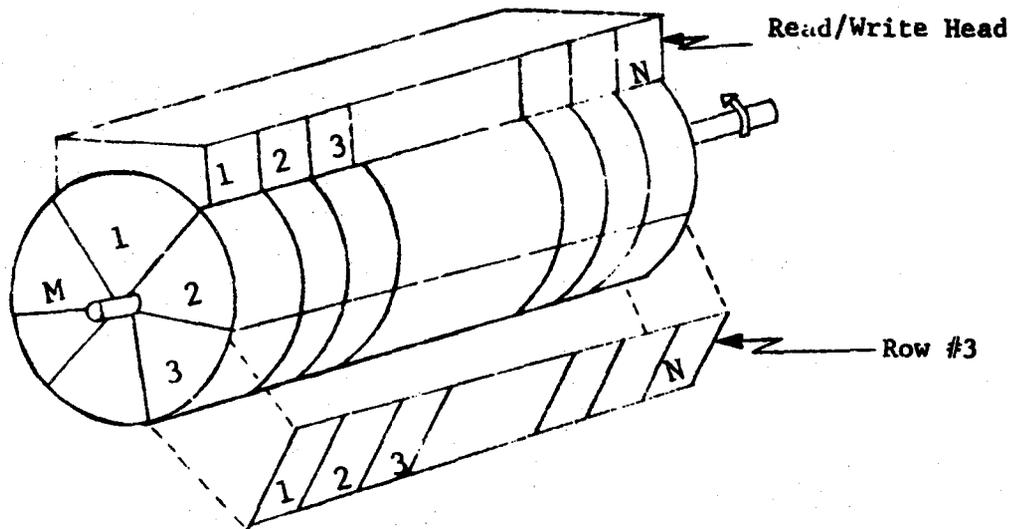
Figure 1. Drum Configuration
