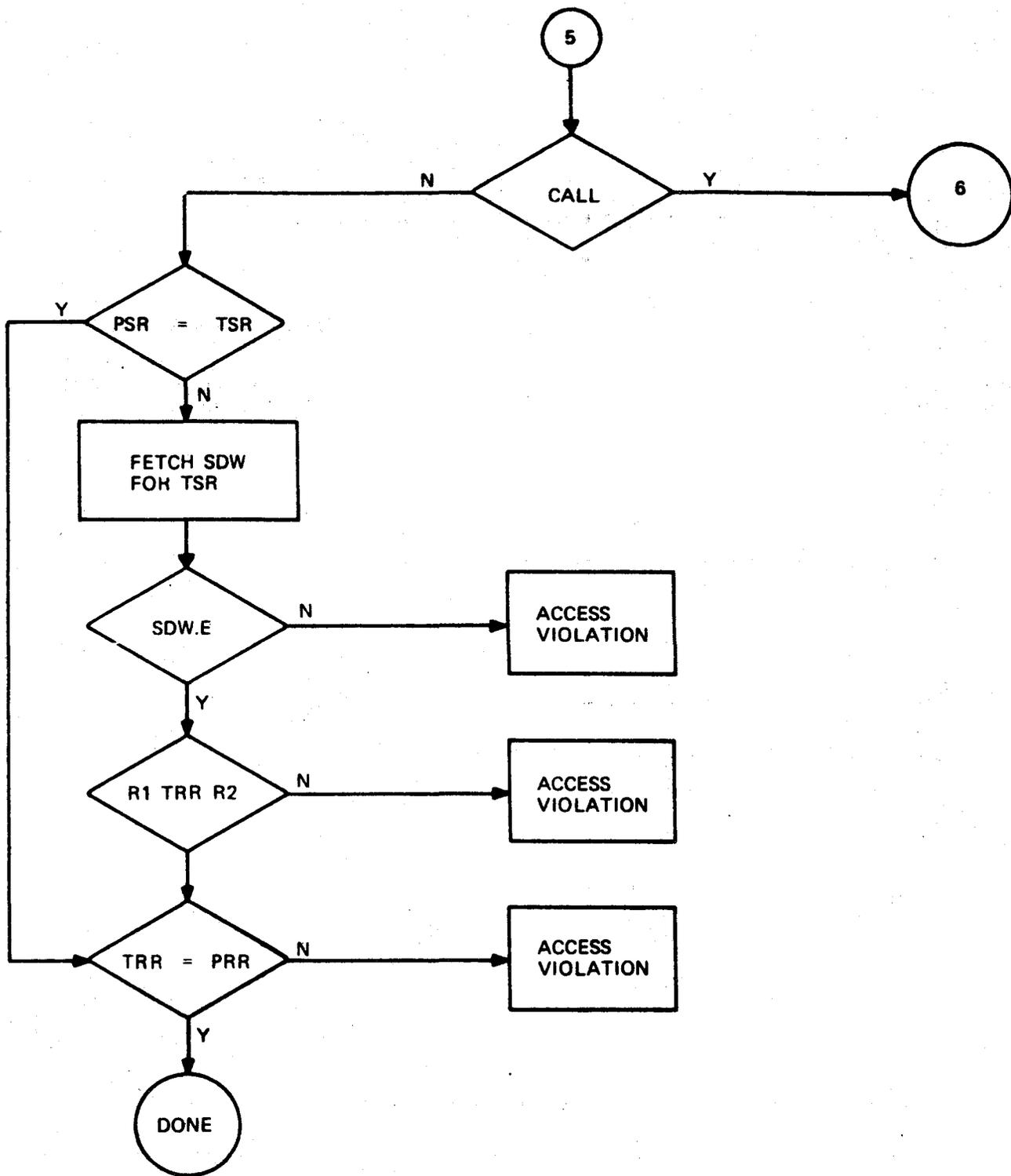
Figure 5. Access Checks for Transfer Instructions, Except CALLn
