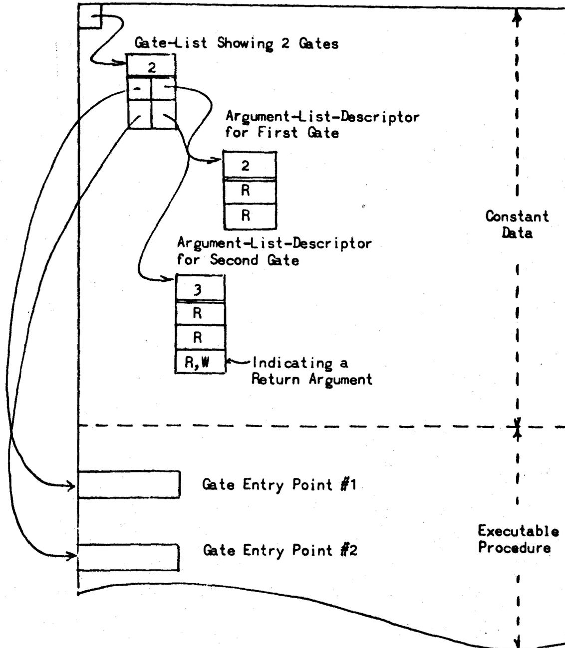
Figure 5. A Gate Segment Showing Gate Entry Points, Gate-List and Argument-List Descriptors
